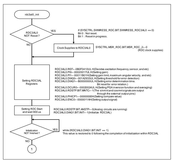
Figure 2-8 Flow of the RDC3AL initialization
