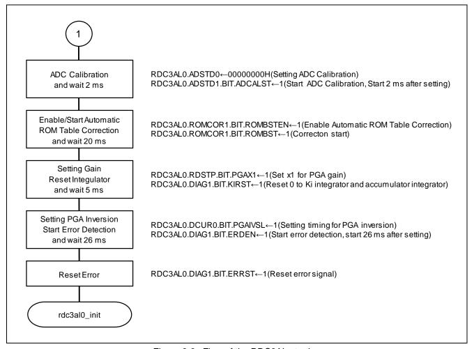
Figure 2-9 Flow of the RDC3AL starting
