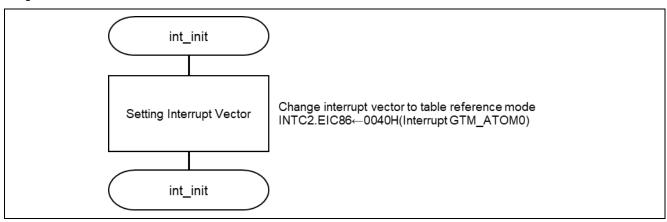
Figure 2-7 Flow of the INTC setting
