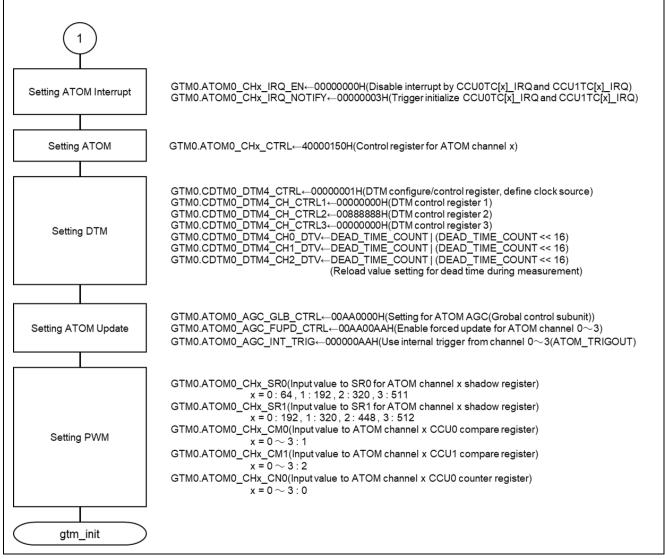
Figure 2-4 Flow of the GTM initial setting  $(x = 0 \sim 3)$
