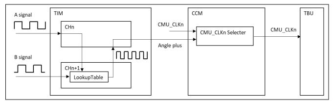
Figure 2-2 Clock flow within GTM
