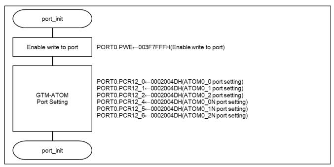
Figure 2-11 Flow of the PORT initial setting
