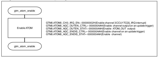
Figure 2-5 Flow of the ATOM startup setting
