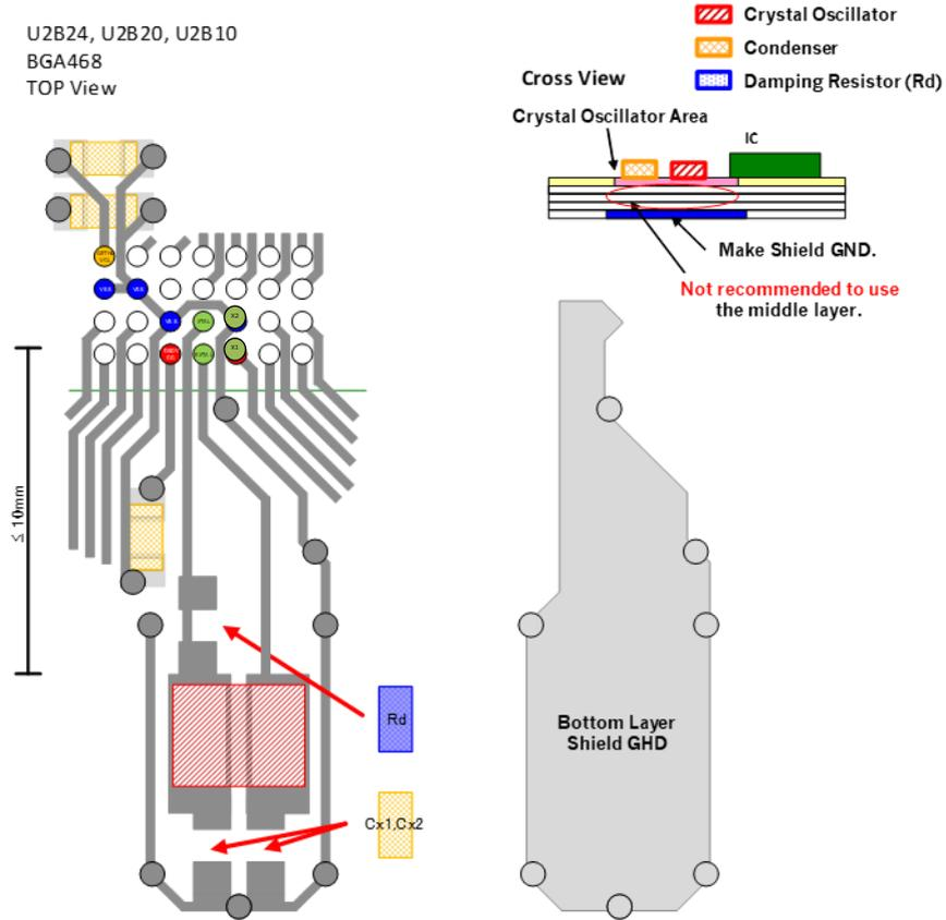
Figure 2 Bord Pattern Example for Stable Oscillation (U2B BGA468)
