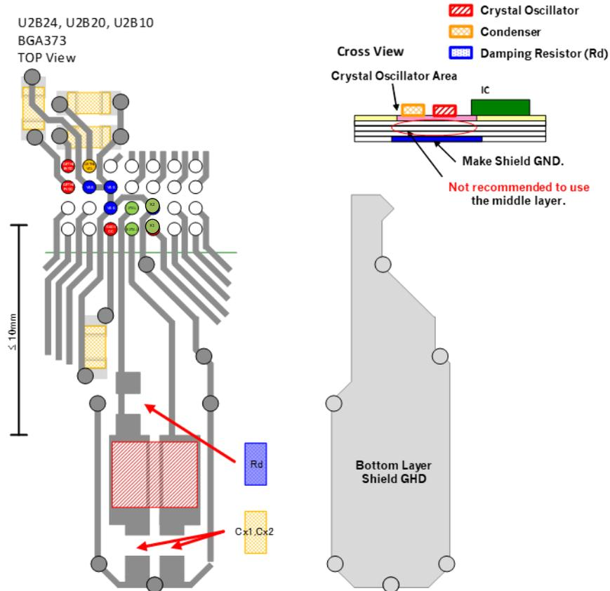
Figure 3 Bord Pattern Example for Stable Oscillation (U2B BGA373)
