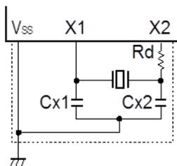
Figure 7 External Circuit Example
