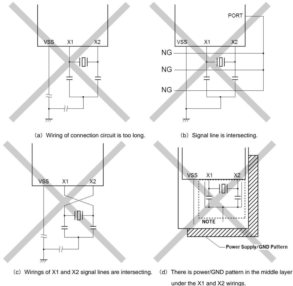
**Note** The capacitance between PINs between X1 and X2 may deteriorate the oscillation characteristics. Therefore, please avoid signal crossings. Also, when the wiring runs in parallel, pay attention to the wiring interval and parallel running distance so that the capacity during this period does not increase.
