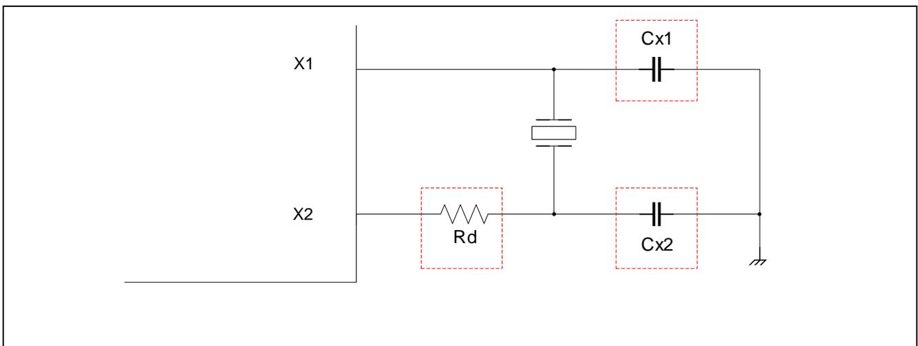
Figure 1 Recommended Connection Circuit of Crystal Oscillator
