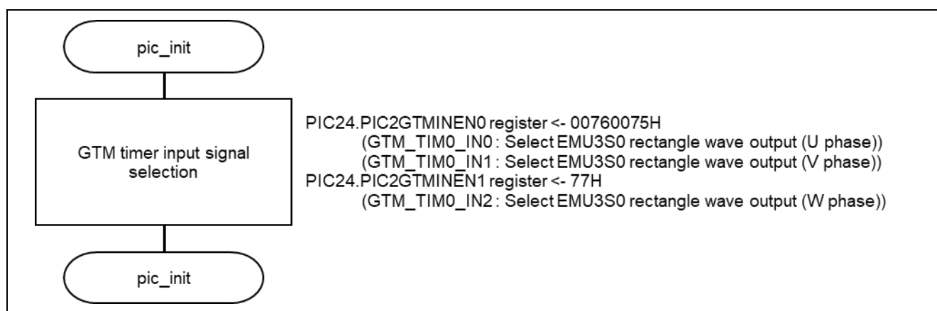
Figure 2-3 PIC initial settings
