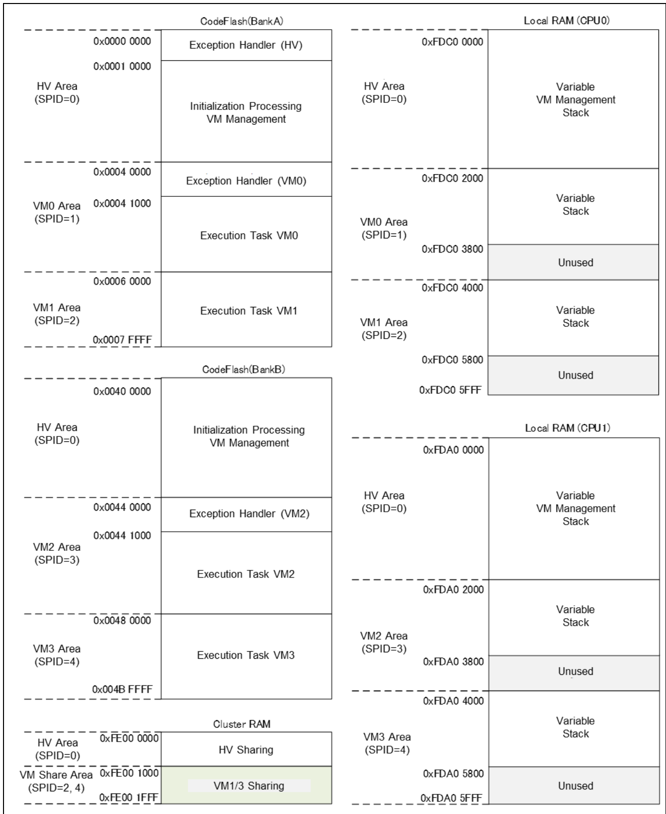
Figure 3-2 MPU Memory Management
