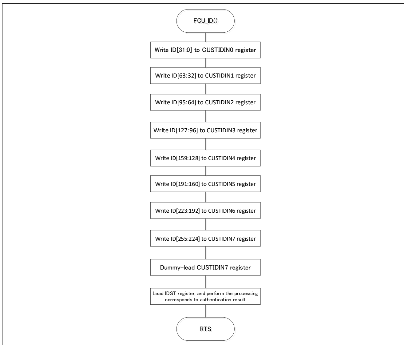
Figure 4-6 “FCU_ID() Function” Flowchart “Operation Procedure ③”
