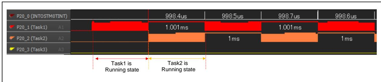
Figure 3-15 Operation waveform of Round Robin Scheduling program
