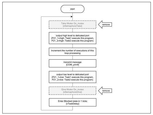
Figure 3-42 Flowchart of each task of Mutex program without using Mutex
