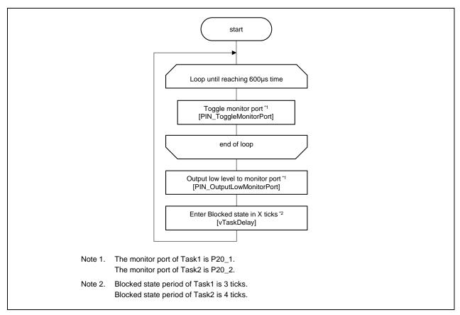
Figure 3-18 Flowchart of Task1 and Task2 of Preemption Scheduling program
