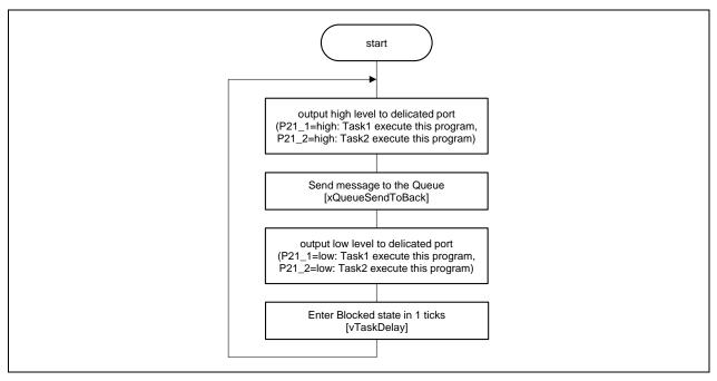
Figure 3-47 Flowchart of each task of Gatekeeper Task program
