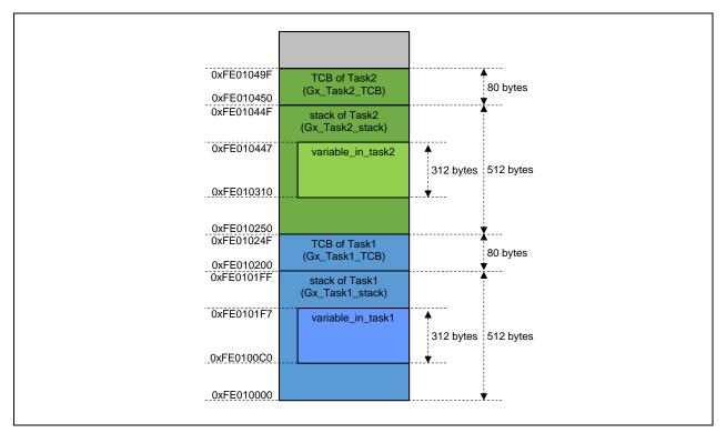
Figure 3-4 Memory allocation result for Static Memory program
