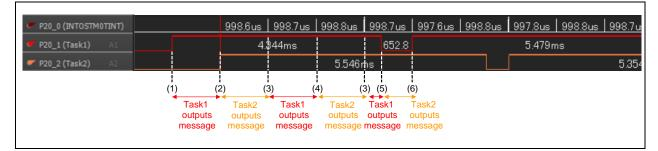
Figure 3-44 Operation waveform of Mutex program that does not use Mutex
