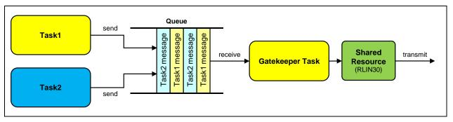
Figure 3-45 Image of messages transmission via Gatekeeper Task
