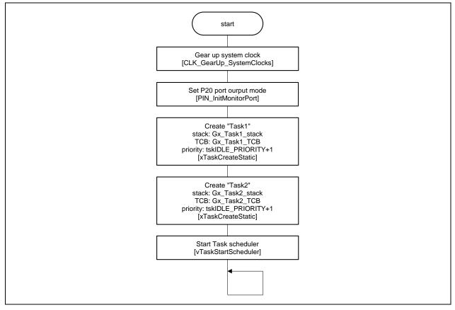
Figure 3-1 Flowchart of main of Static Memory program
