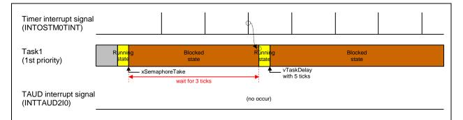
Figure 3-25 Timing chart of Binary Semaphore program when Semaphore is not released
