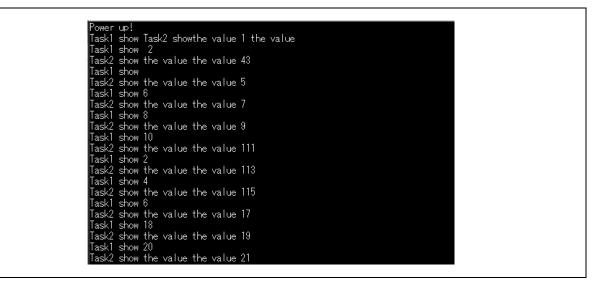
Figure 3-43 Operation log of Mutex program that does not use Mutex
