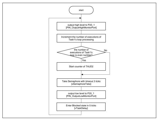
Figure 3-28 Flowchart of Task1 of Binary Semaphore program
