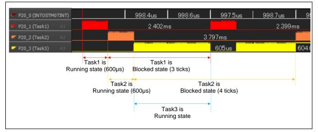
Figure 3-19 Operation waveform of Preemption Scheduling program
