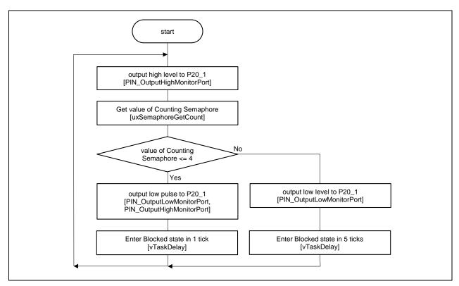
Figure 3-34 Flowchart of Task1 of Counting Semaphore program
