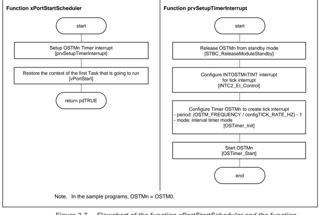
Figure 2-7 Flowchart of the function xPortStartScheduler and the function prvSetupTimerInterrupt
