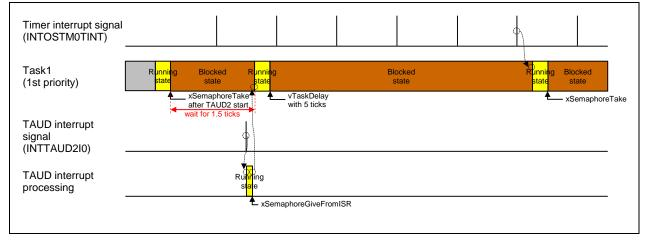
Figure 3-26 Timing chart of Binary Semaphore program when Semaphore is released
