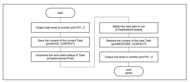
Figure 2-8 Flowchart of the function \_Intfunc\_INTOSTM0TINT
