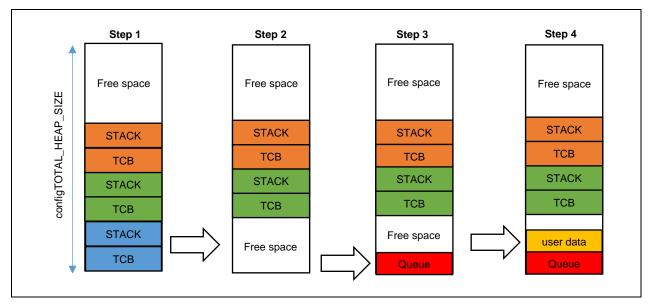
Figure 3-6 Memory allocation image after deleting Task and creating Queue
