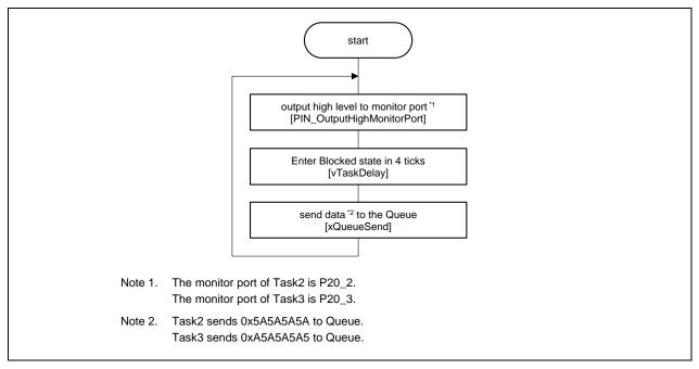
Figure 3-23 Flowchart of Task2 and Task3 of Queue program
