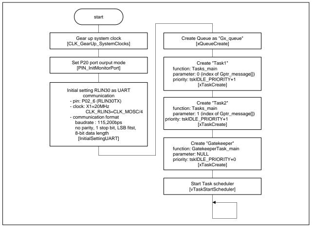
Figure 3-46 Flowchart of main of Gatekeeper Task program
