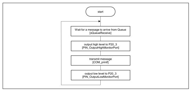
Figure 3-48 Flowchart of Gatekeeper Task of Gatekeeper Task program
