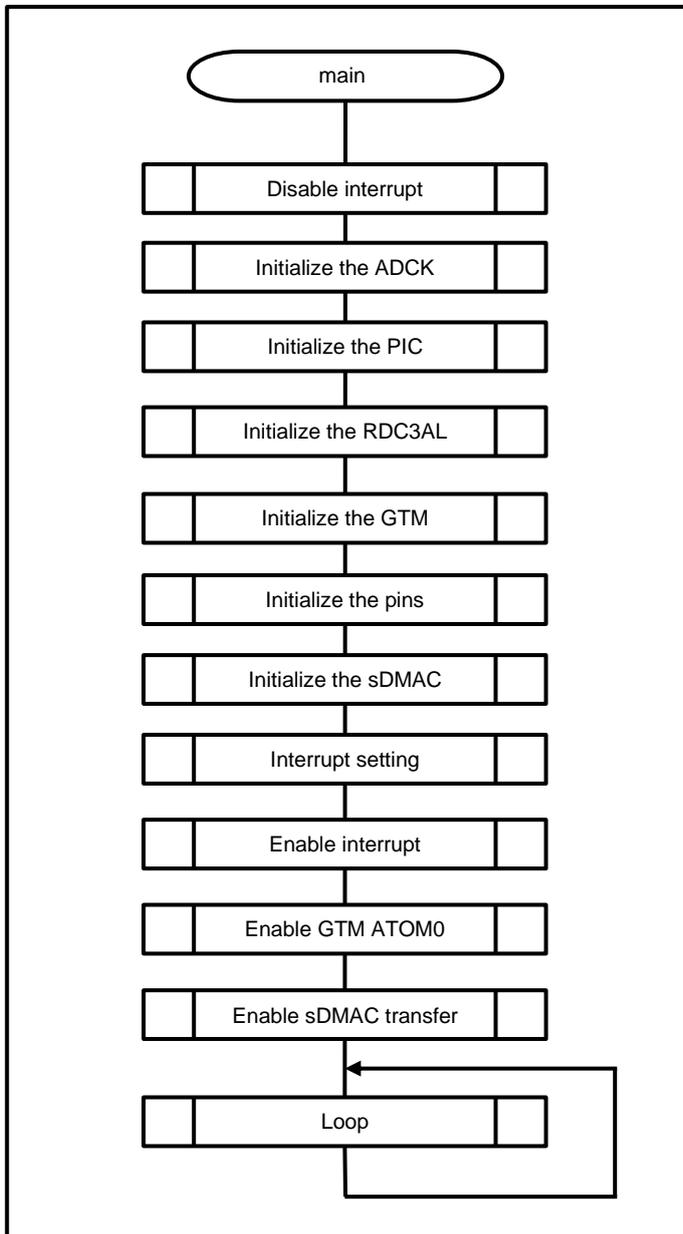
Figure 5.2 PE1 Main Processing
