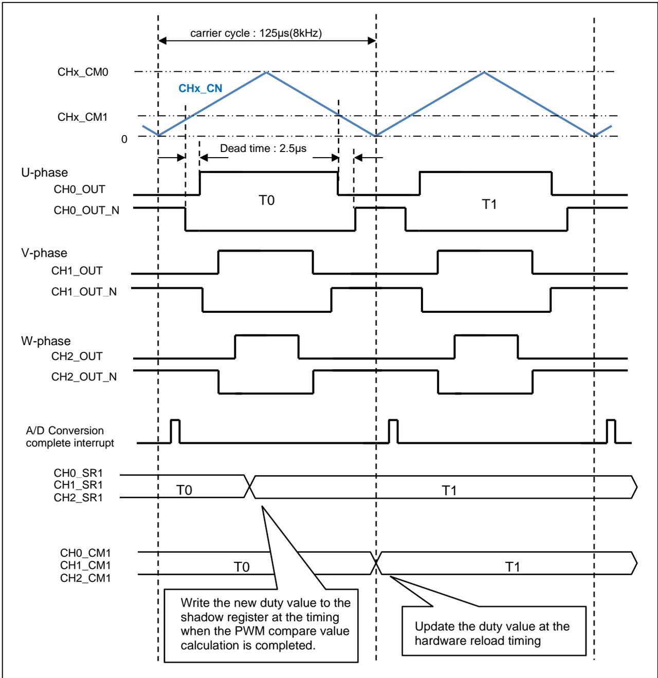
Figure 5.1 Three phase PWM waveform timing diagram
