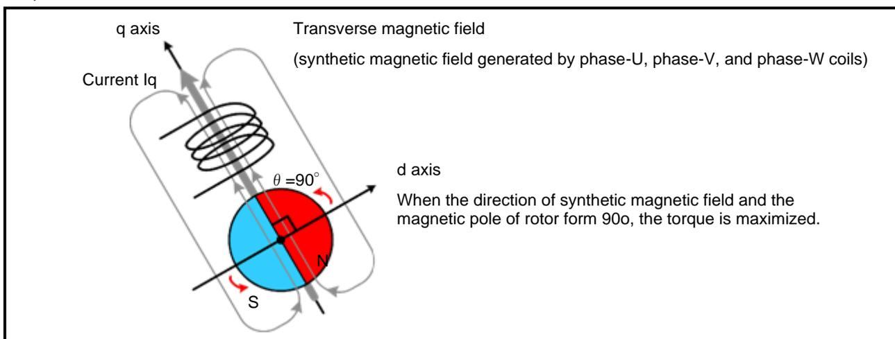
**Figure 1.2 Relationship between Synthetic Magnetic Field and Torque**
