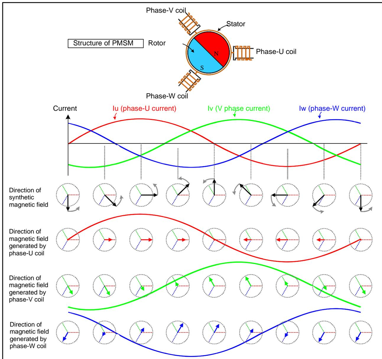
Figure 1.1 PMSM Structure and Synthetic Magnetic Field
