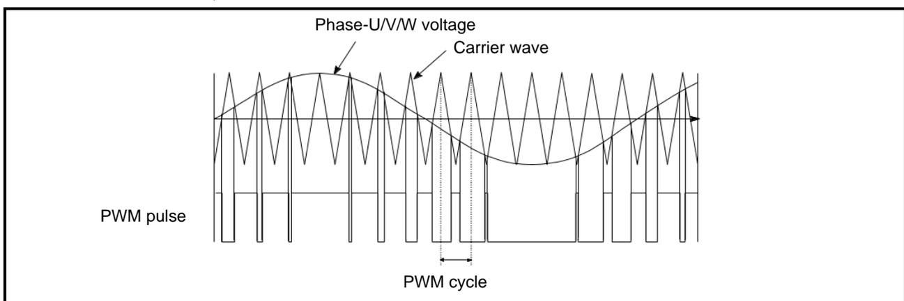
**Figure 1.4 Triangular Wave Comparison Method**
