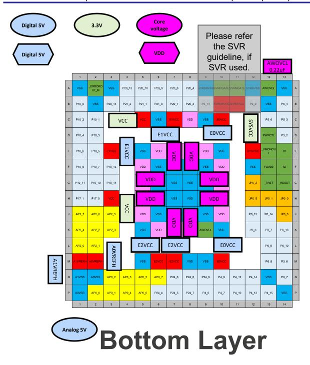
For examples of PCB board design, please refer to "3.3 Example capacitor placement for BGA292 package (U2A16/U2A8)".
