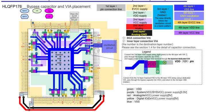
The 1st and 4th layers are displayed superimposed(Gray is the 1st layer, color is the 2nd layer, and 4th layer)
