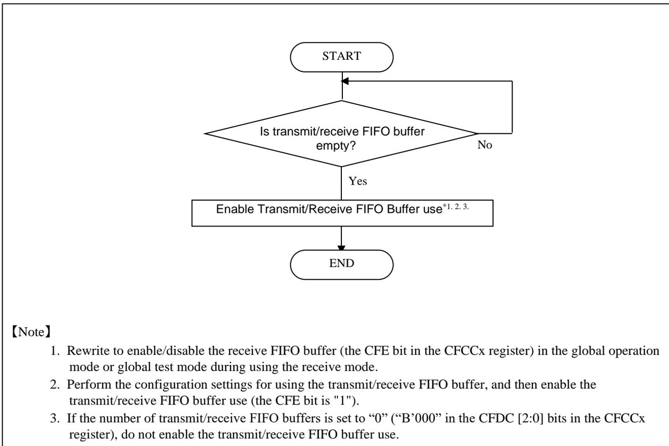
Figure 4-3 Transmit/Receive FIFO Buffer Use Enable Procedure
