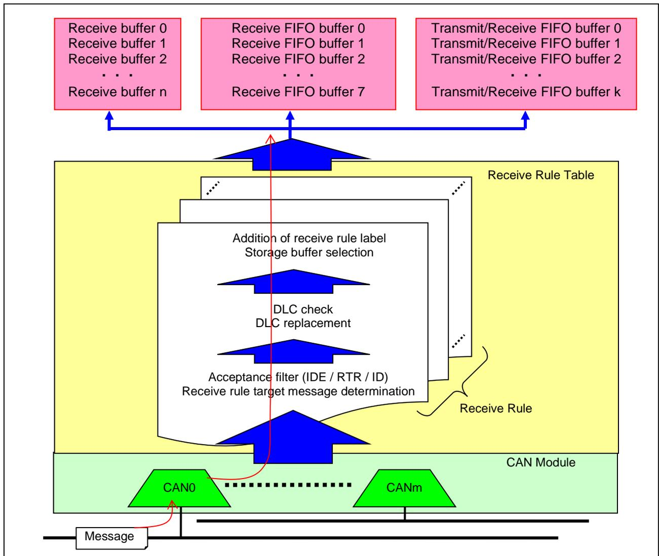
Figure 7-1 Filtering Image by receive rule table
