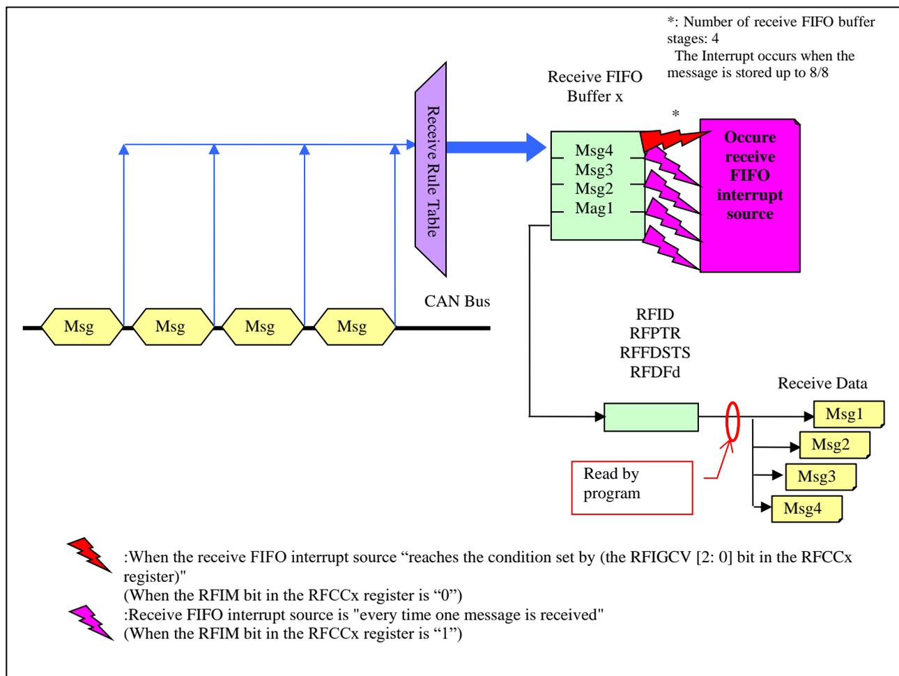
Figure3-1 Receive FIFO Buffer Operation
