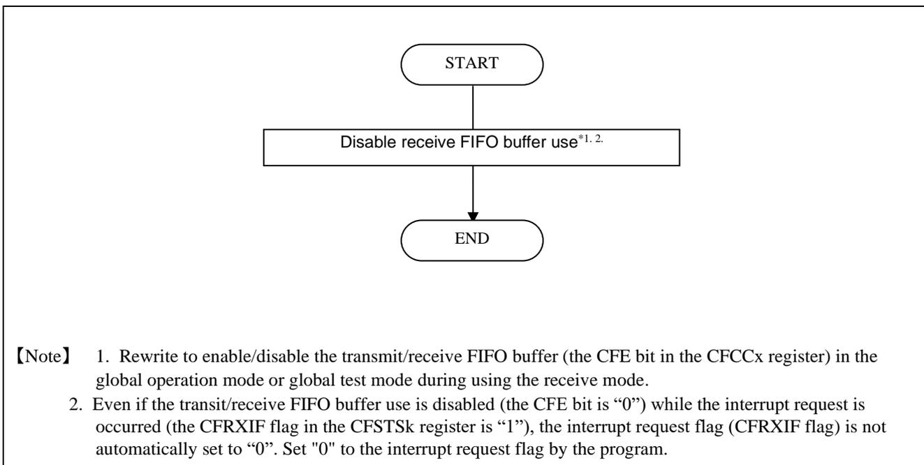
Figure 4-4 Transmit/Receive FIFO Buffer Use Disable Procedure
