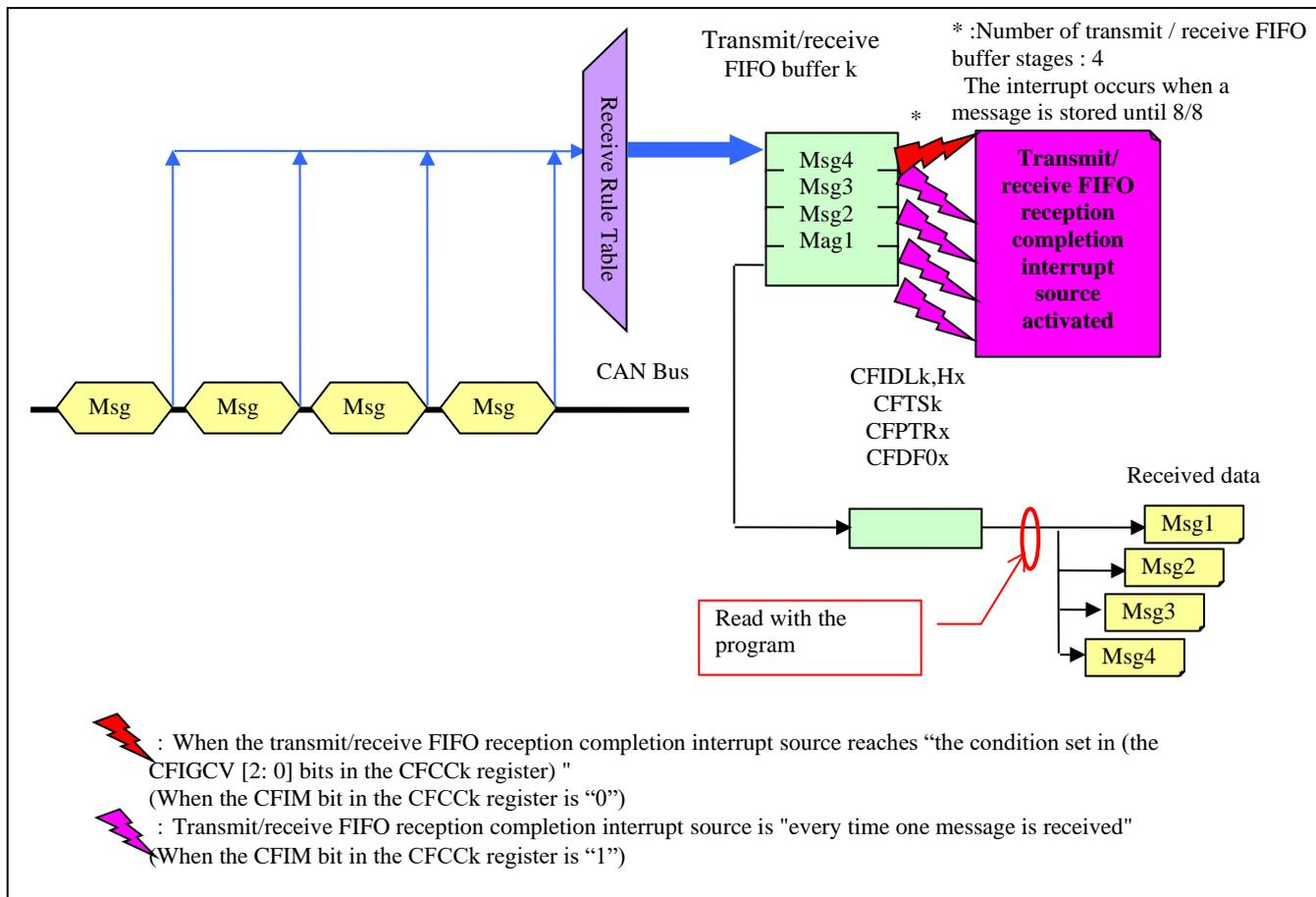
Figure 4-1 Transmit/Receive FIFO Buffer Operation (Receive mode)
