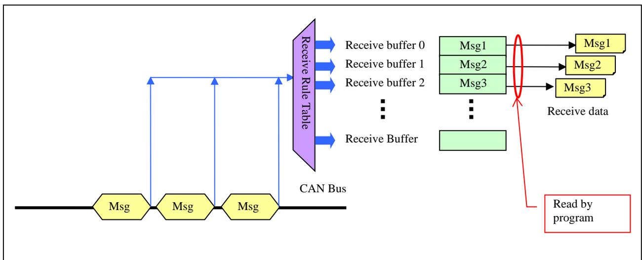
Figure 2-1 Receive Buffer Operation
