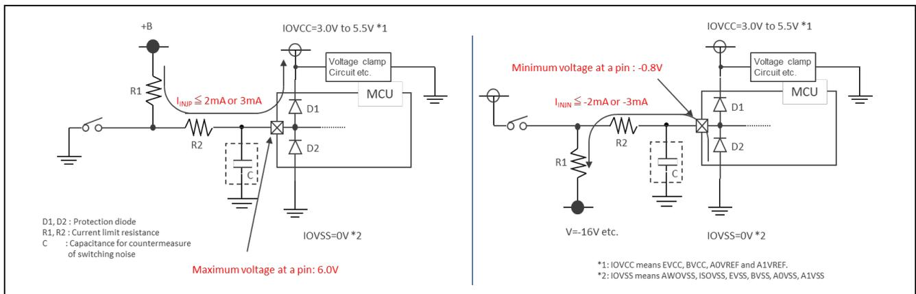
Figure 26: Mechanism of injection current
