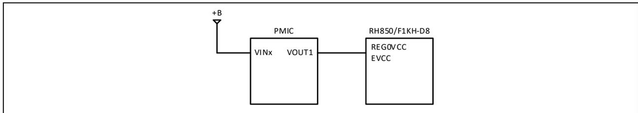
**Figure 12: Recommended REG0VCC power configuration for RH850/F1KH-D8**
