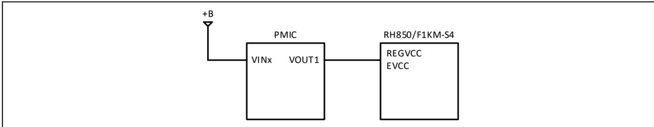
**Figure 7: Recommended REGVCC power configuration for RH850/F1KM-S4**
