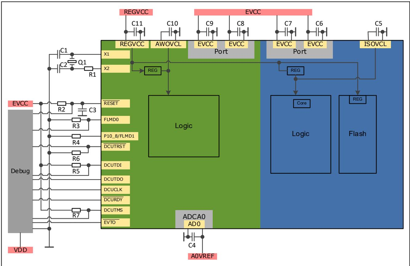
Figure 17: Minimum external components of RH850/F1KM-S1 in normal operating mode
