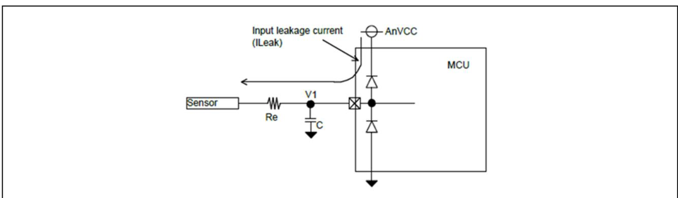
Figure 30: Schematic for sampling error 1 formula
