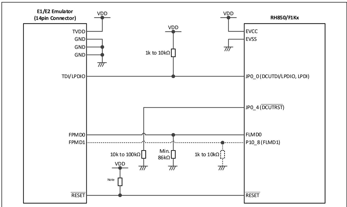
Figure 32: LPD (1 pin) connection
