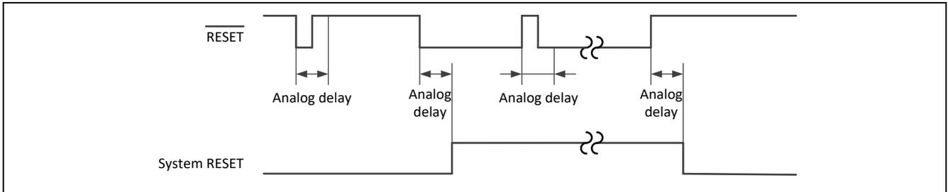
**Figure 24: External RESET timing**
