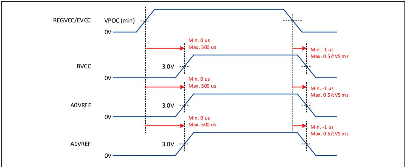
Figure 10: RH850/F1KM-S4 Power up/down timing
