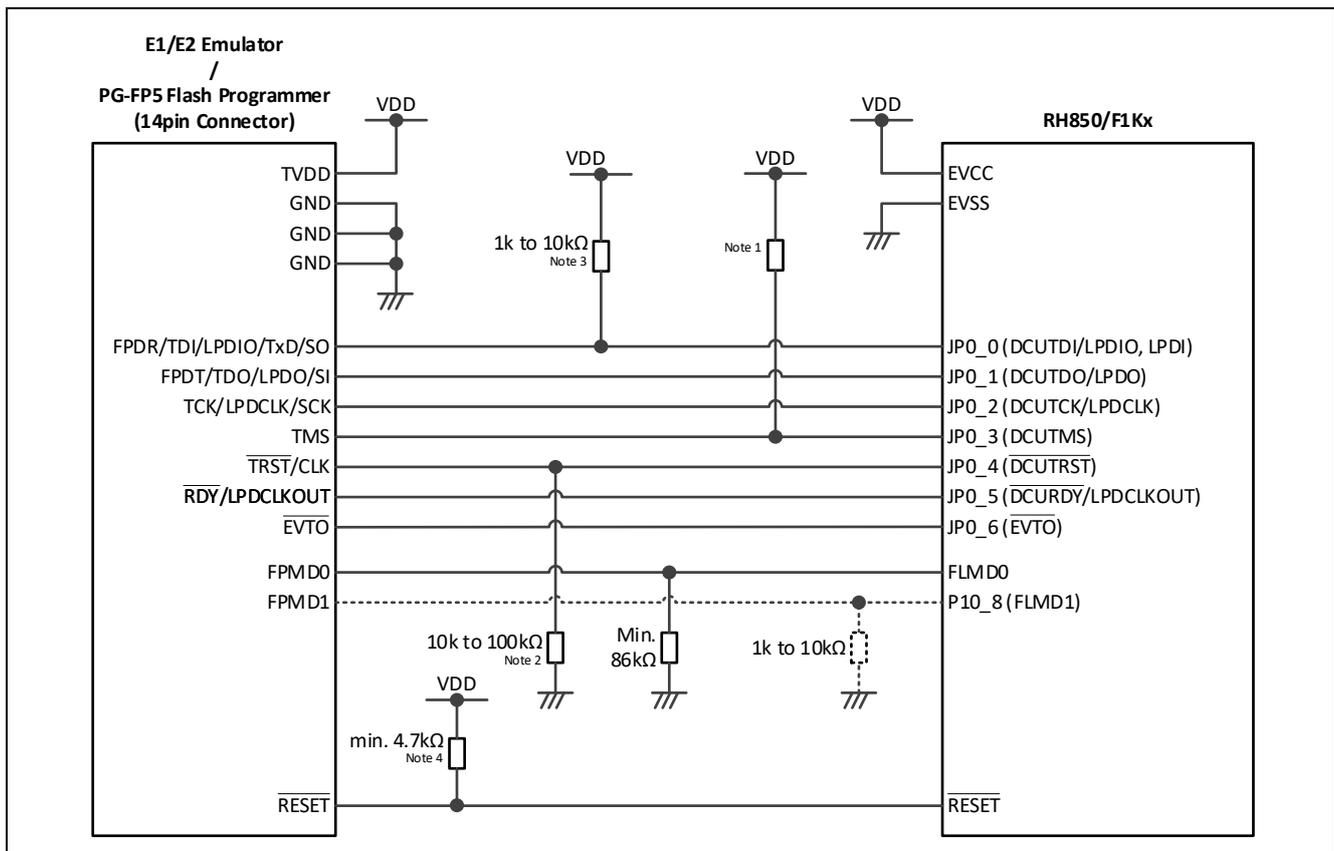
**Figure 37: Combined debug and flash programming interface connections**
