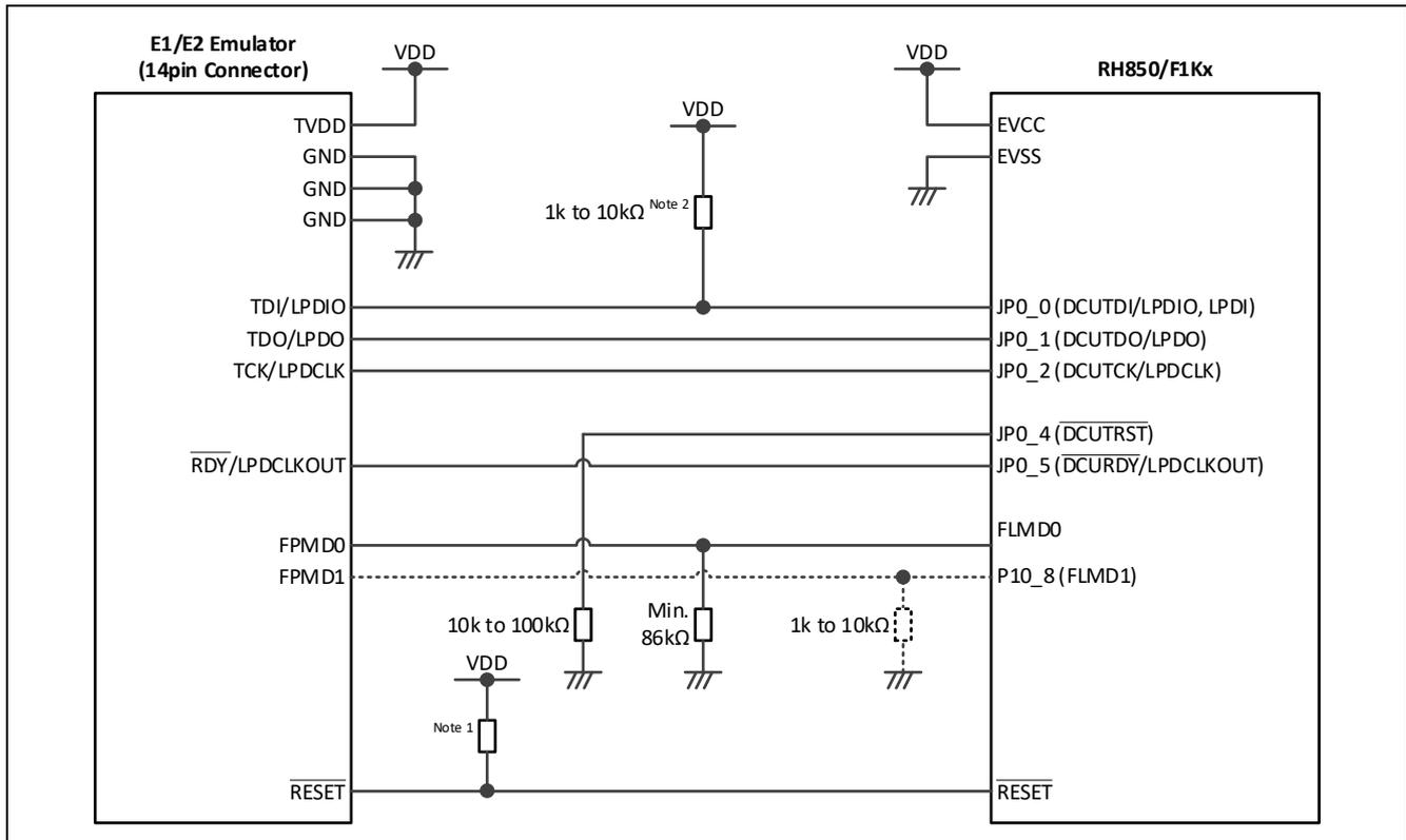
Figure 33: LPD (4 pins) connection
