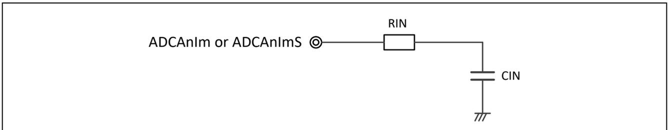
**Figure 28: ADC equivalent input circuit**
