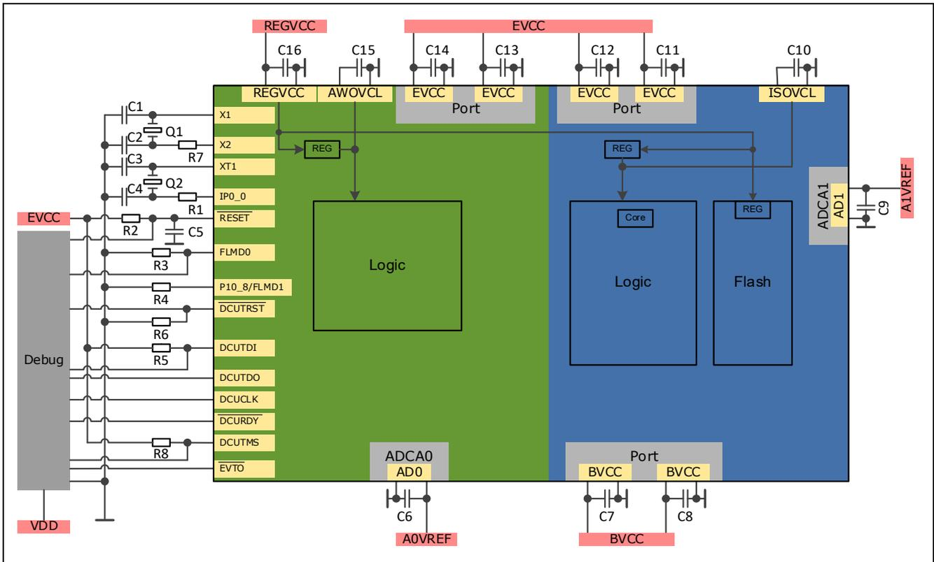
**Figure 18: Minimum external components of RH850/F1KM-S4 in normal operating mode**
