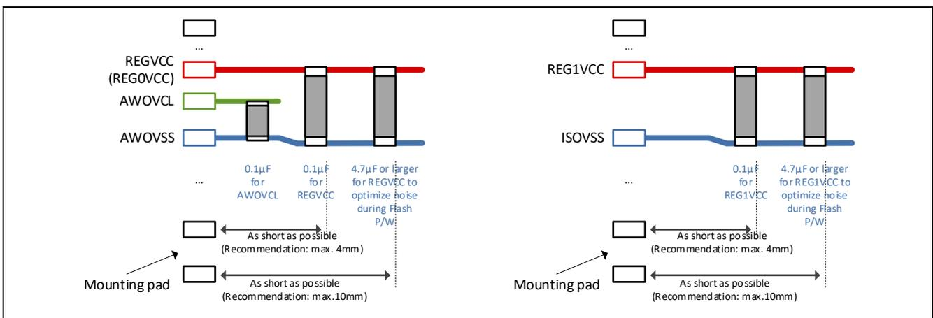
**Figure 16: Principle capacitor placement at REGVCC for EMI**
