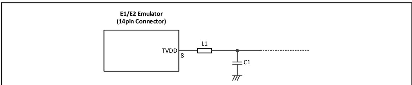
**Figure 38: Circuit configuration for hot plug-in**
