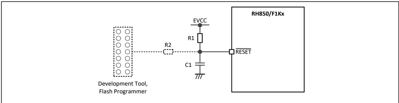
Figure 23: Minimum RESET circuit
