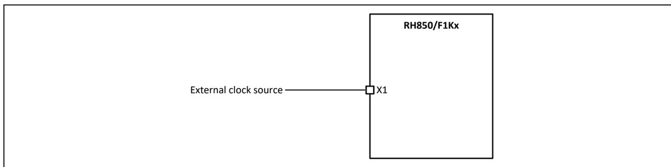
**Figure 22: Direct clock supply to X1 (MOSC)**
