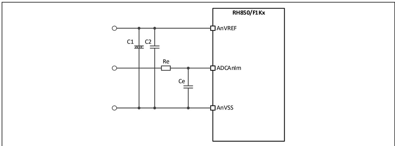
**Figure 29: ADC external circuit on analog input**
