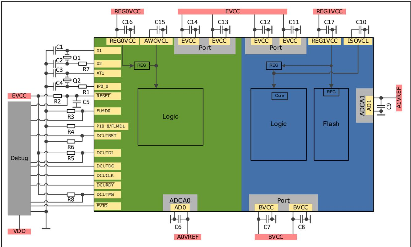
Figure 19: Minimum external components of RH850/F1KH-D8 in normal operating mode
