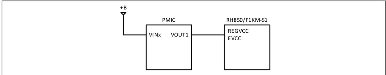
**Figure 2: Recommended REGVCC power configuration for RH850/F1KM-S1**
