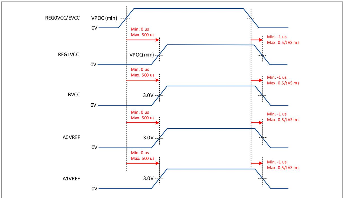
**Figure 15: RH850/F1KH-D8 Power up/down timing**
