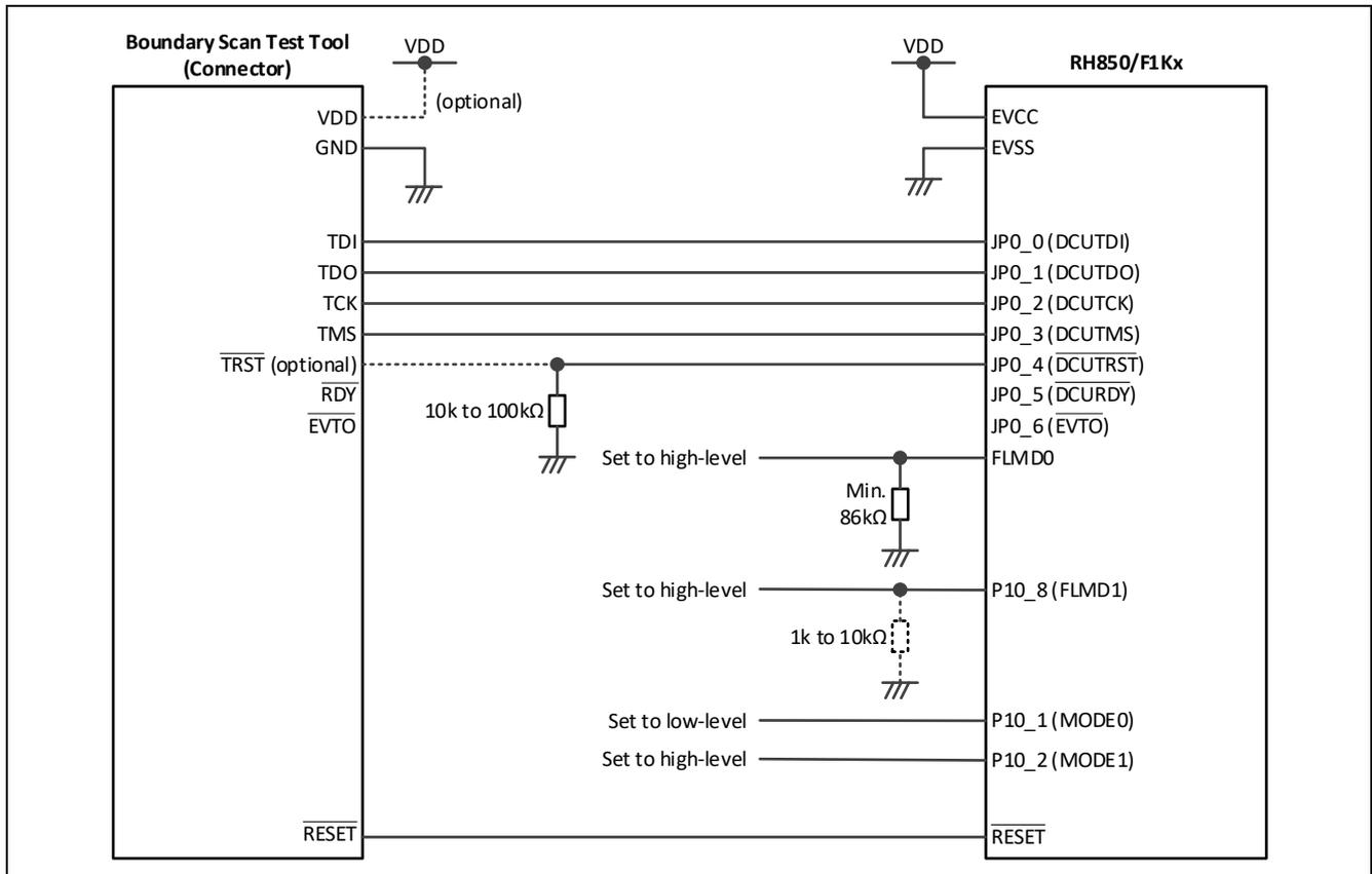
**Figure 39: Boundary scan connection of RH850/F1Kx series**
