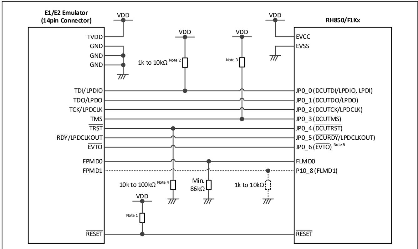
Figure 34: Nexus, LPD (4 pins) and LPD (1 pin) connection
