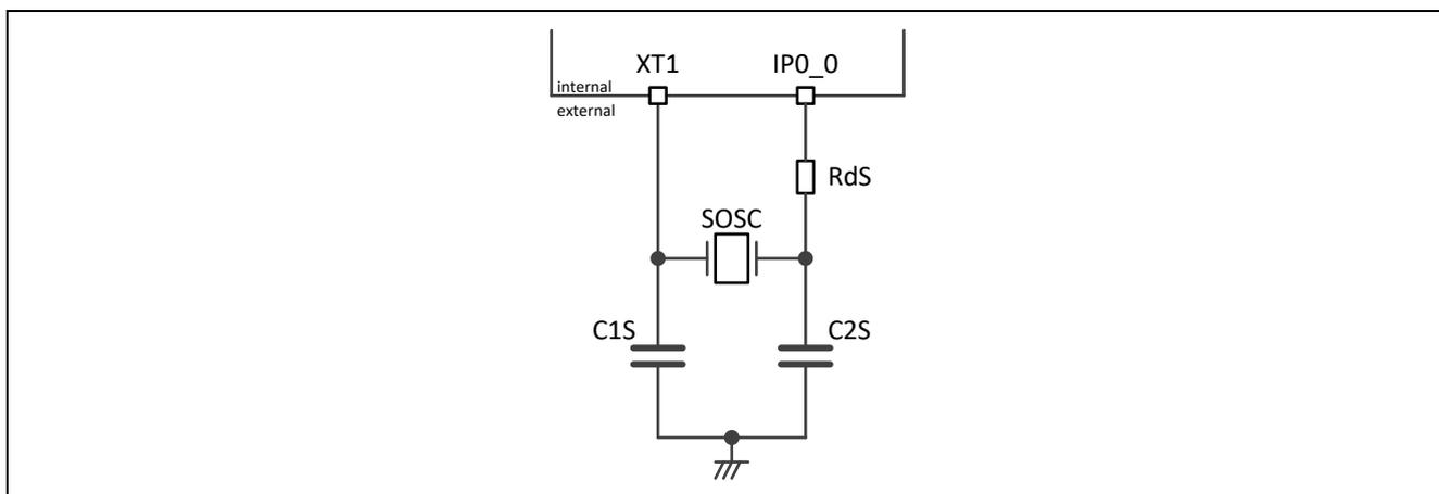
**Figure 21: Recommended sub oscillator circuit**
