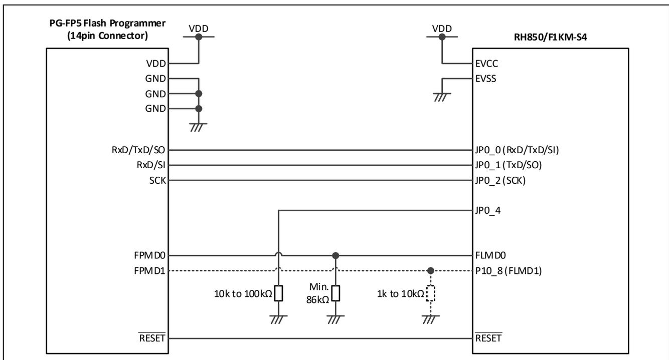
**Figure 35: PG-FP5 flash programming interface connection**
