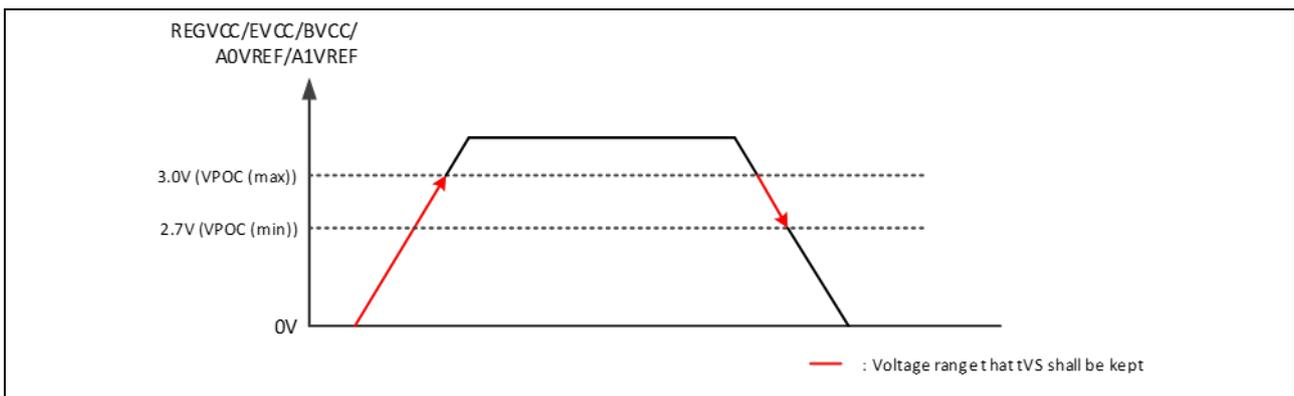
**Figure 8: The voltage range which has to be kept voltage slope for RH850/F1KM-S4**
