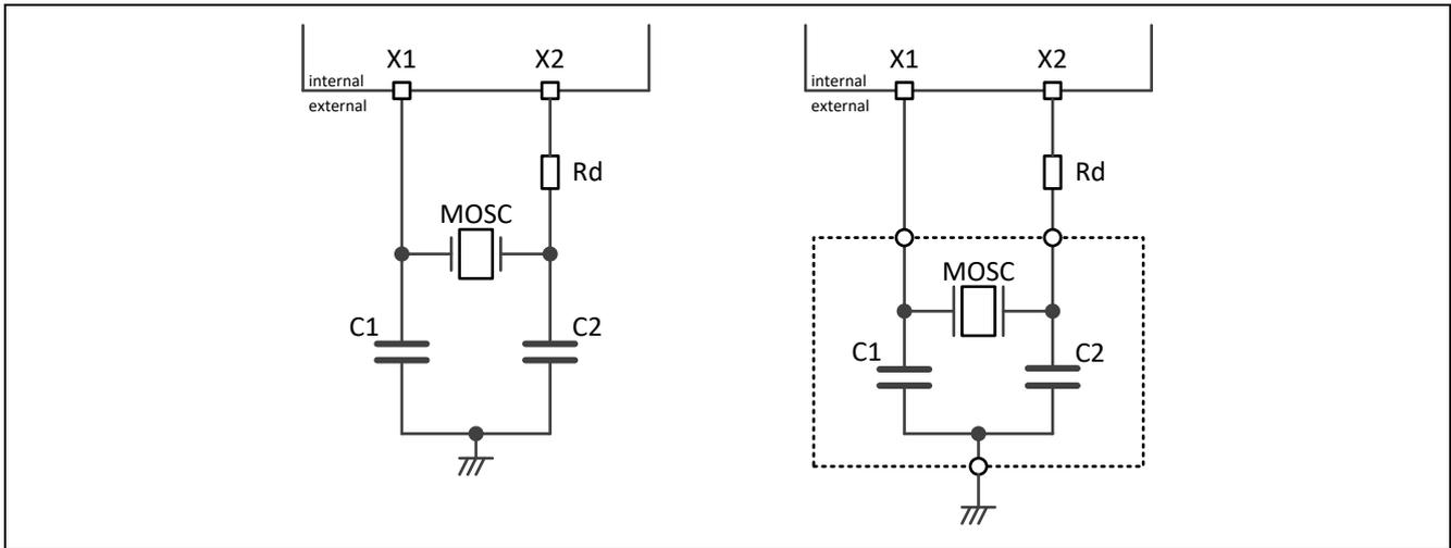
Figure 20: Recommended main oscillator circuit
