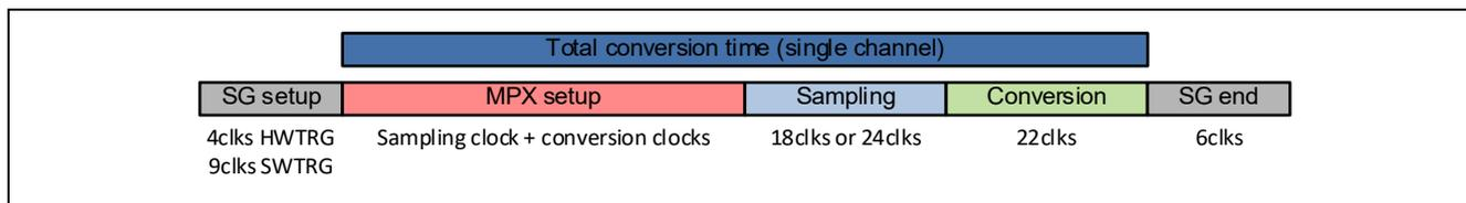
Figure 27: ADC conversion time
