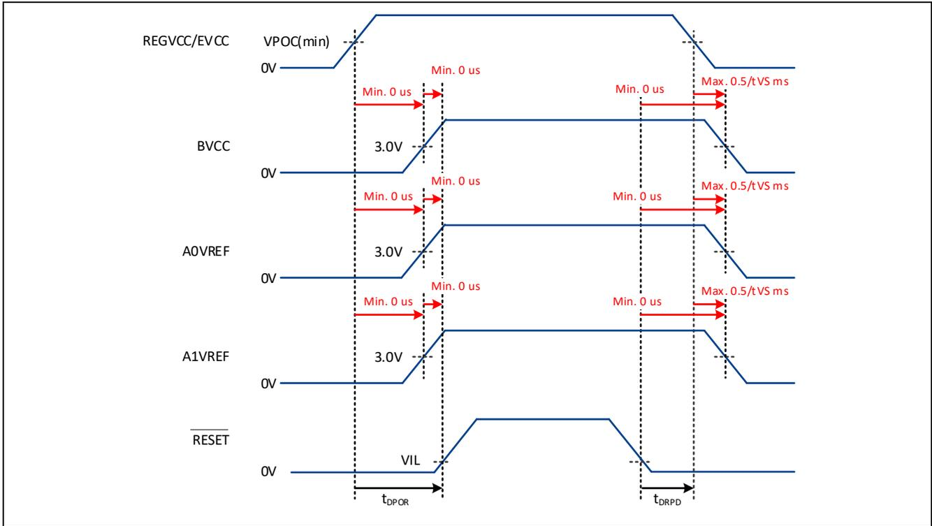
Figure 9: RH850/F1KM-S4 Power up/down timing
