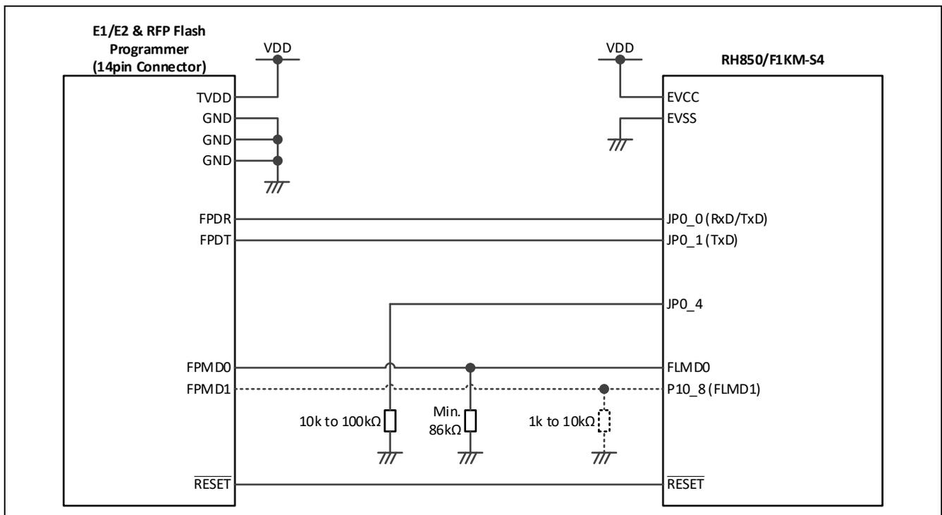
**Figure 36: E1/E2 flash programming interface connection**
