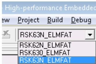
**Figure 2.** In HEW, Select the Build Configuration for the board you are going to use. Selecting configuration determines which files are included in the project, include file directory paths, build options, etc.
