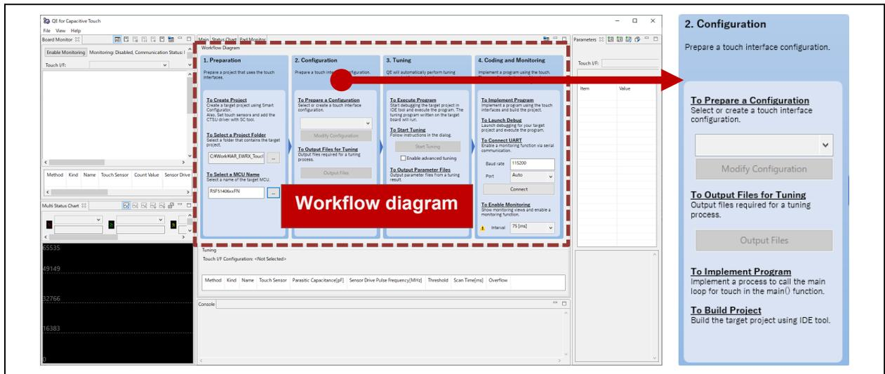
Figure 3-1 Standalone-Version QE - Workflow Diagram: <Step 2> Configuration
