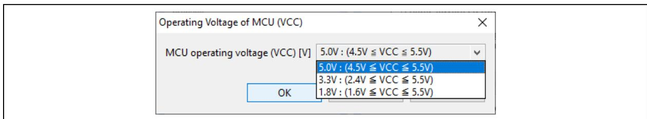
Figure 3-9 Setting the Operating Voltage (VCC) of the MCU
