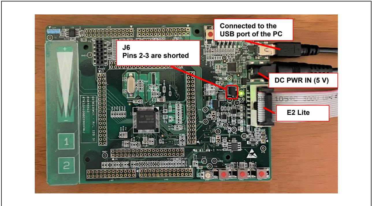
Figure 4-2 Connecting the RSK-RX140 Board
