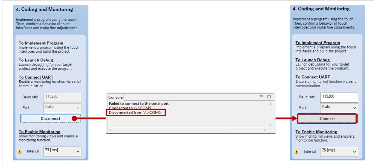
Figure 5-10 <Step 4> Coding and Monitoring: Disconnect
