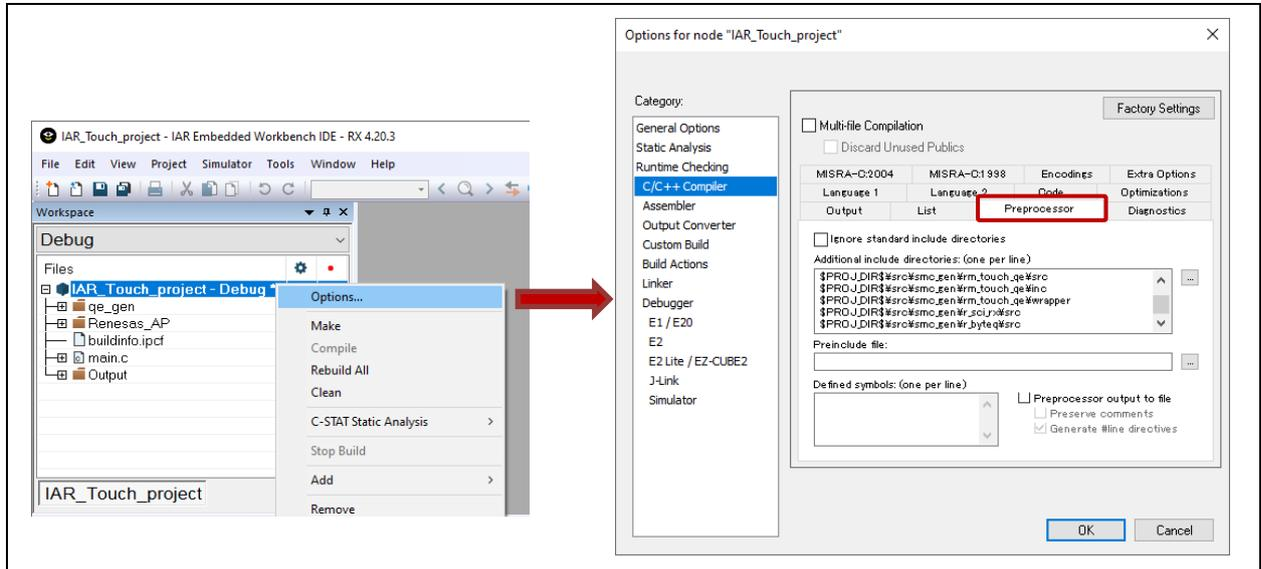
Figure 3-17 Displaying the [Preprocessor] Tab of "C/C++ Compiler"
