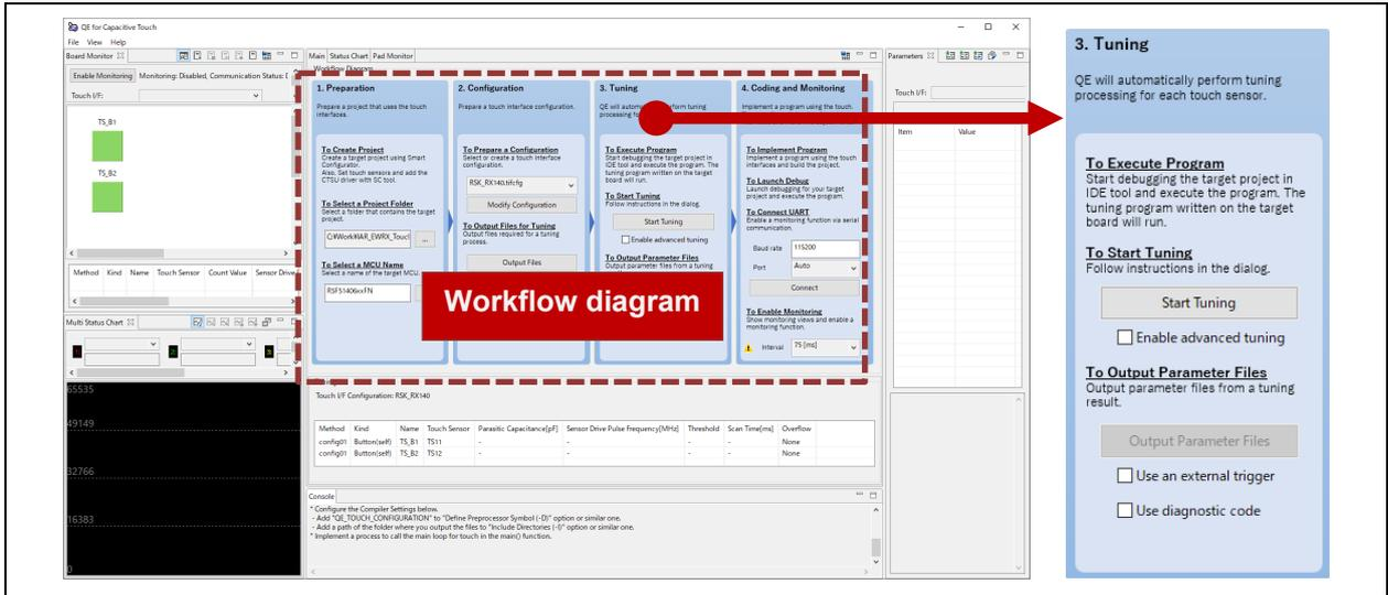
Figure 4-1 Standalone-Version QE - Workflow Diagram: <Step 3> Tuning
