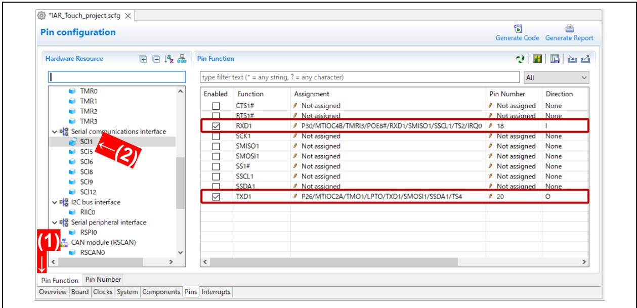
Figure 2-22 Assigning Pin Functions for SCI1 ((1): [Pin Function] Tab, (2): SCI1)
