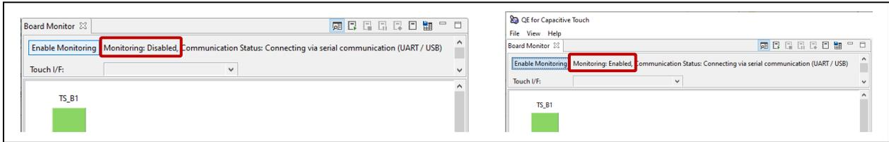
Figure 5-3 Enabling the Monitoring Function
