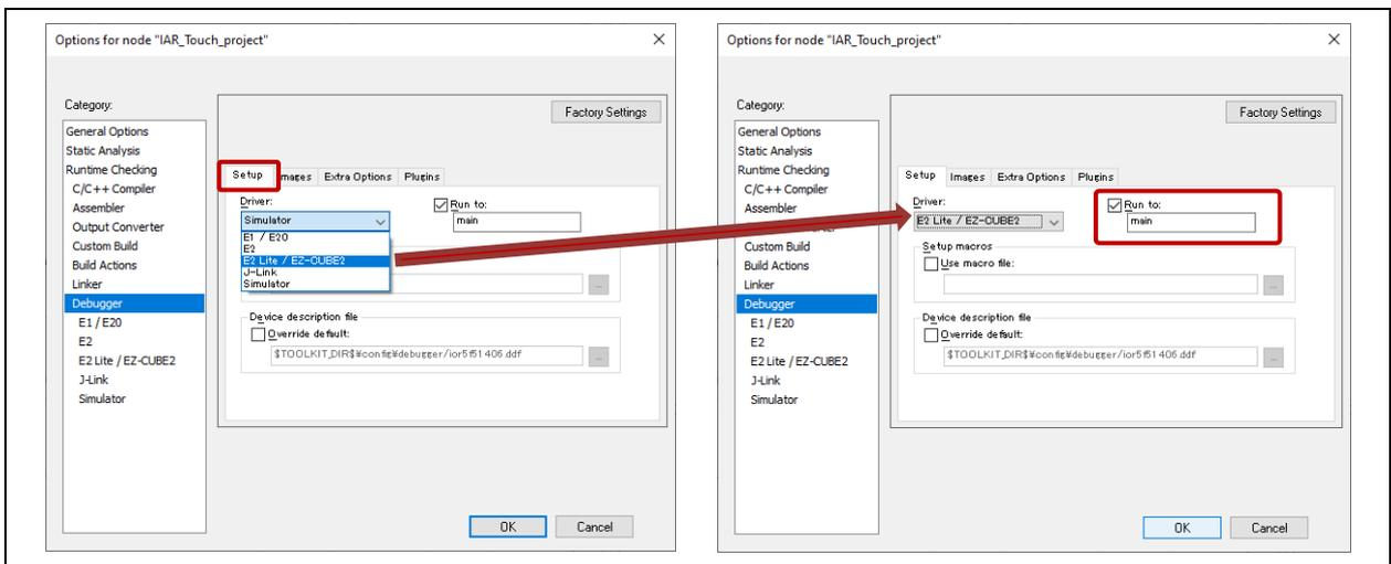
Figure 3-21 Debugger - [Setup] Tab
