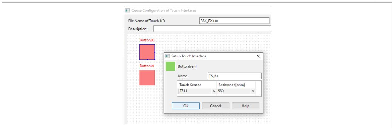
Figure 3-4 Setting the Touch Interface Items for Button00
