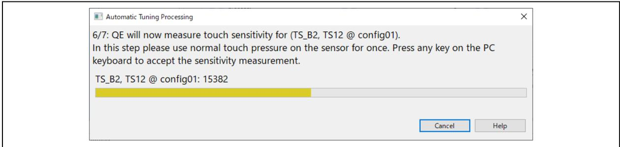
Figure 4-7 "Automatic Tuning Processing" - Measuring the Touch Sensitivity (TS\_B2)
