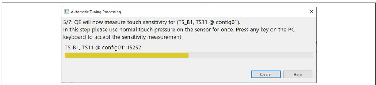
Figure 4-6 "Automatic Tuning Processing" - Measuring the Touch Sensitivity (TS\_B1)
