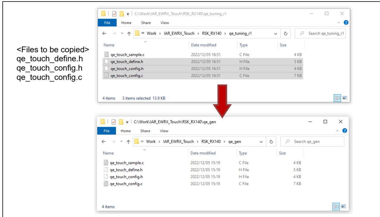
Figure 4-12 Copying the Files with Tuned Values
