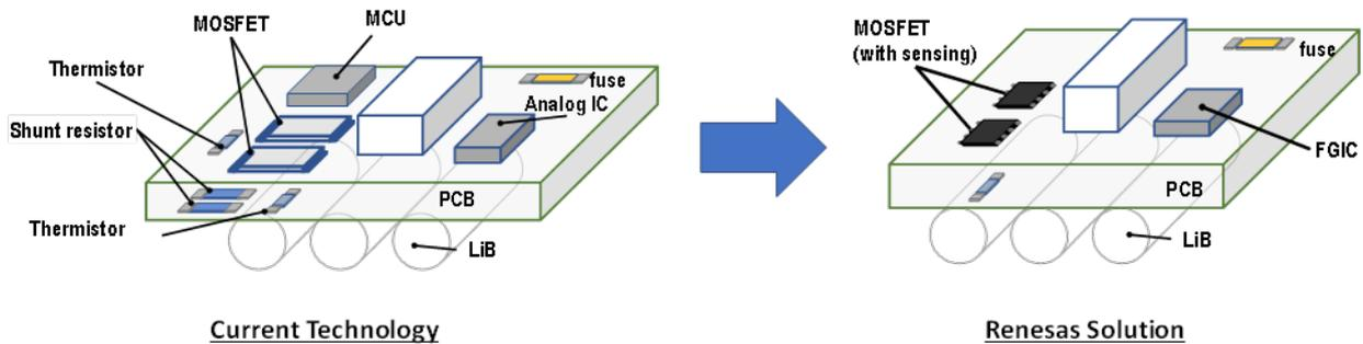
**Figure 2-4 Shunt-less solution by kits of MOSFET with sensing and FGIC**
