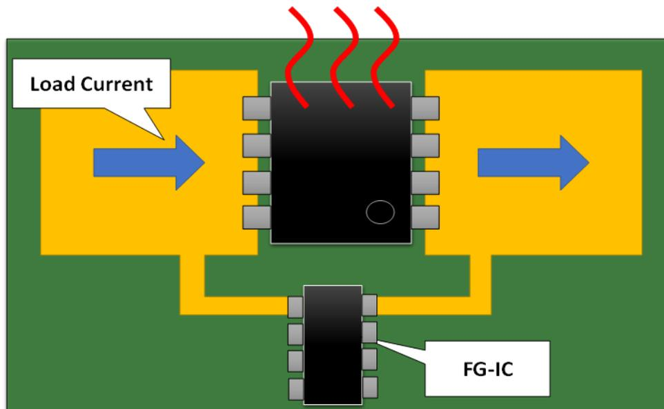
Figure 2-3 New method for MOSFET temperature monitoring
