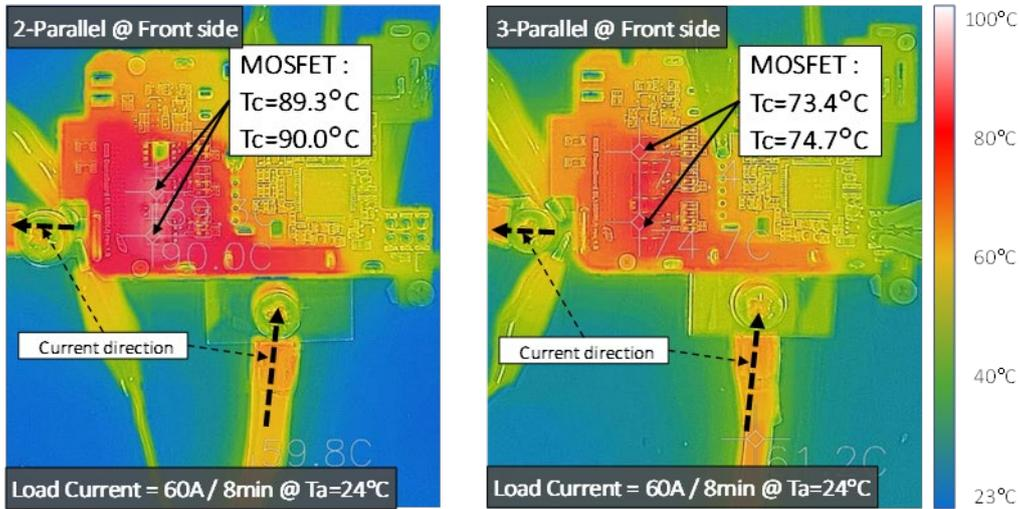
Figure 3-6 Thermograph Photo compare between 2-Parallel & 3-Parallel
