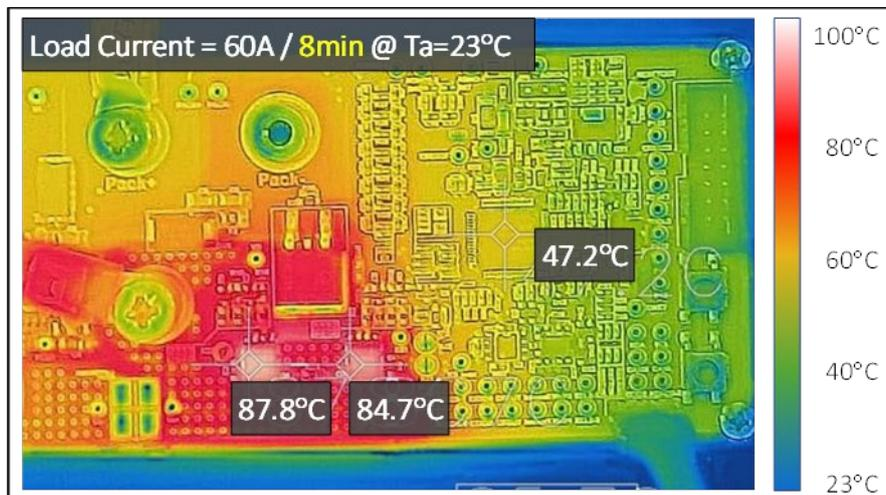
Figure 3-2 Thermograph Photo for Renesas BMS Shunt-less Solution EVB
