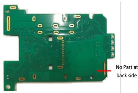
Figure 3-4 Back side of the Evaluation Board
