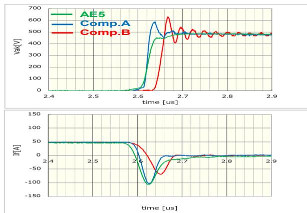
Figure 3-7 FRD waveform comparison during recovery operation
