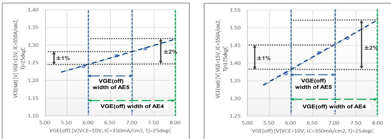
Figure 3-2  $V_{GE(off)}$  vs  $V_{CE(sat)}$
