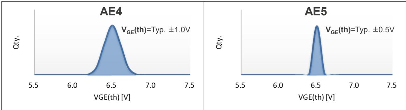
Figure 2-2  $V_{GE(th)}$  Distribution Comparison
