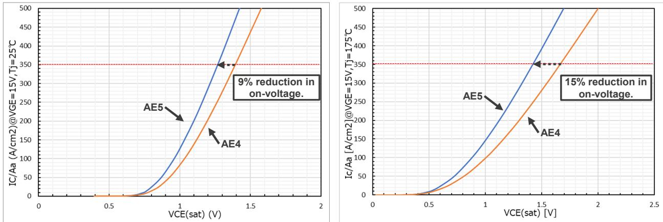
Figure 3-1  $V_{CE(sat)}$  reduction on different temperature level
