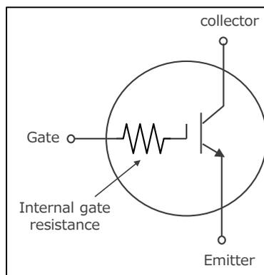
Figure 2-3 The AE5 IGBT with built-in gate resistor
