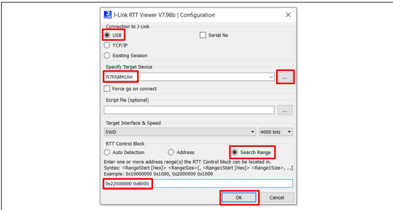
**Figure 35. Configure the RTT Viewer for RA8M1 Project**
