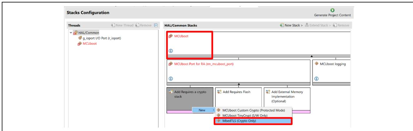
Figure 52. Add MbedTLS (Crypto Only) Module
