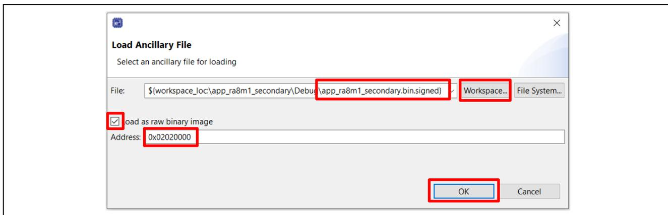
**Figure 37. Load the Secondary Application Image for Overwrite Mode**
