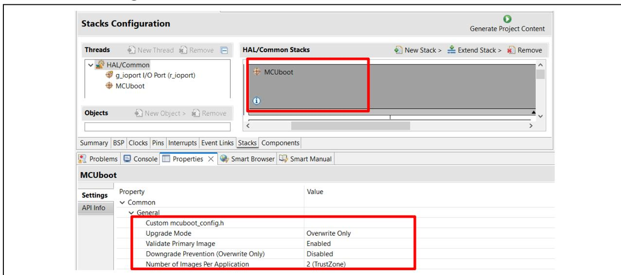
Figure 3. FSP MCUboot Module General Configuration Properties
