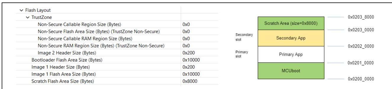
**Figure 64. Memory Configuration of Swap Test Update Mode RA8M1 without TrustZone**
