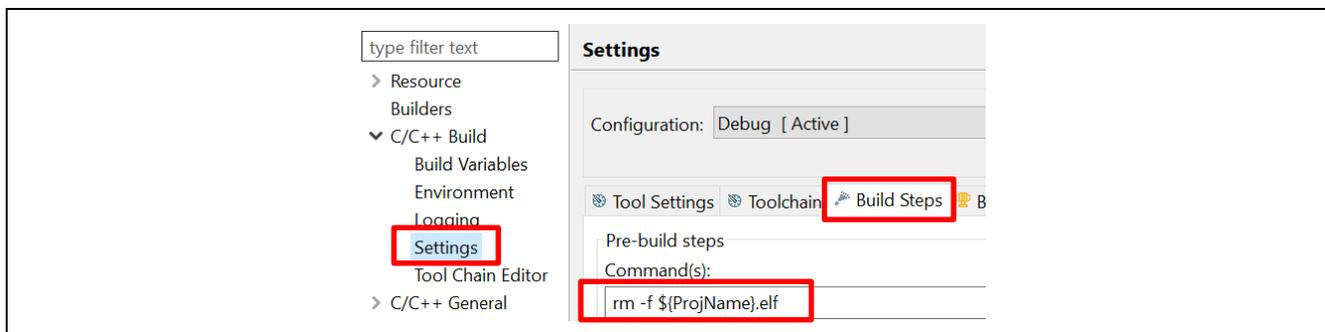
Figure 73. Configure the Pre-build Command
