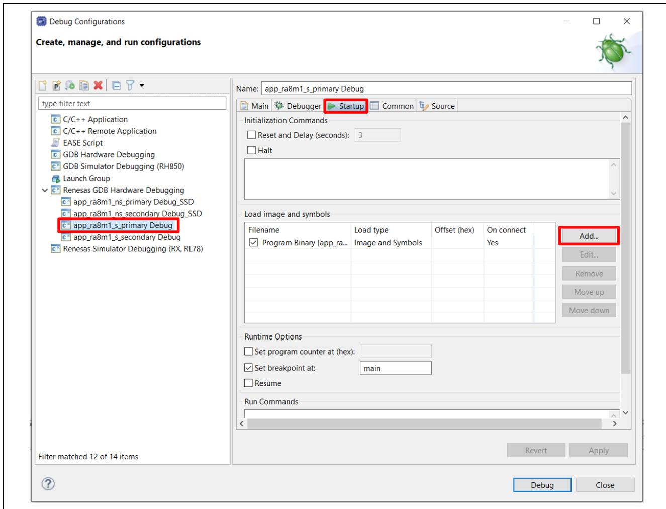
Figure 74. Configure the Primary Secure Project Debug Startup
