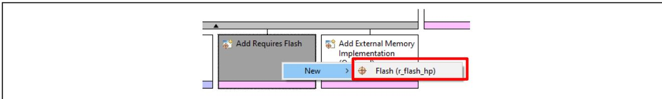
Figure 55. Add the `r_flash_hp` Stack
