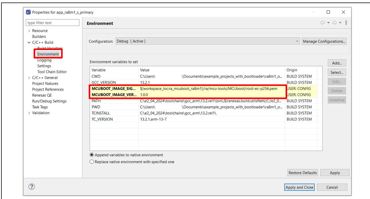
Figure 72. Configure the Signing Key and Application Version
