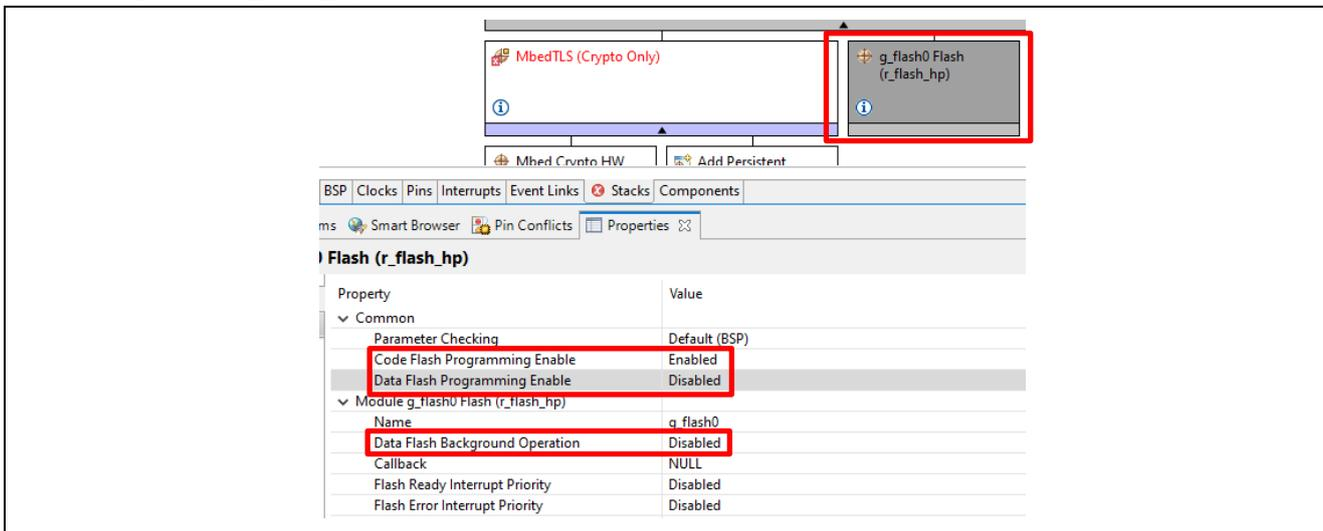
Figure 56. Configure the `r_flash_hp` Stack
