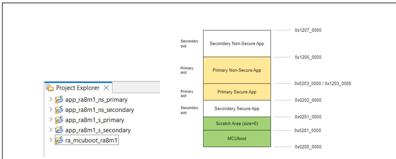
Figure 14. Example Projects for RA8M1 Overwrite Update Mode
