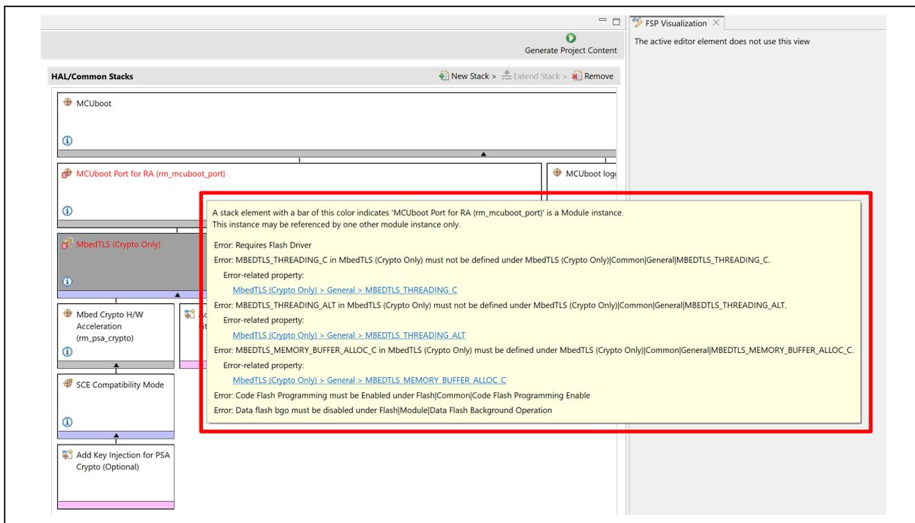
**Figure 53. Dependencies of MCUboot Module for RA Stack**
