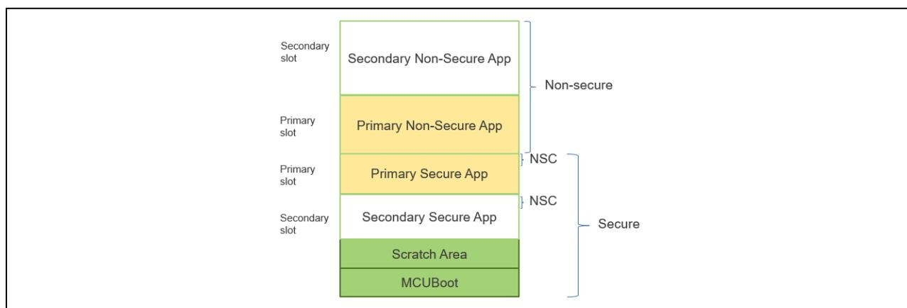
**Figure 2. Two-Image MCUboot Module Memory Map (TrustZone)**
