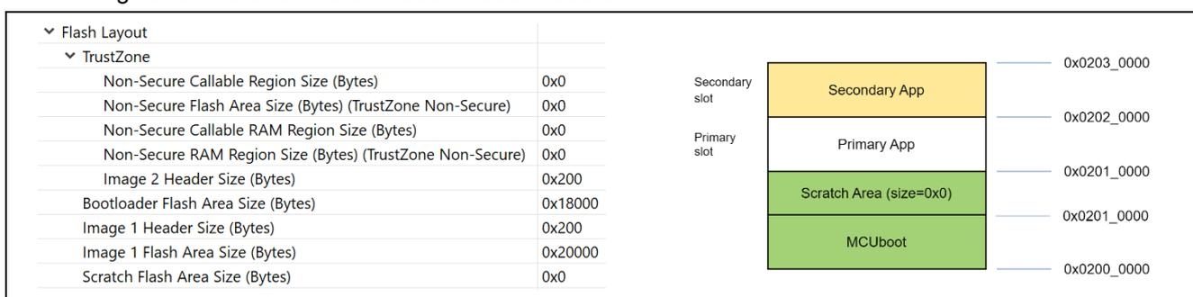
**Figure 63. Memory Configuration of Overwrite Update Mode RA8M1 without TrustZone**
