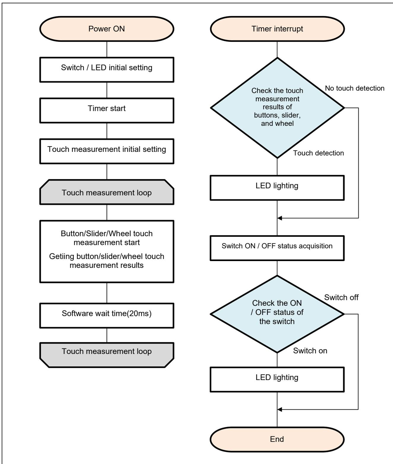
Figure 3-2 Processing Flowchart (Self-Capacitance Buttons / Wheel / Slider Board)
