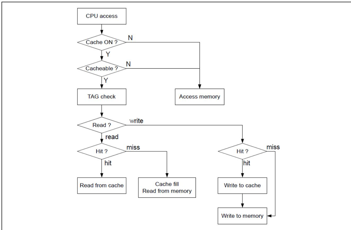
Figure 4. Access flow from CPU to S cache
