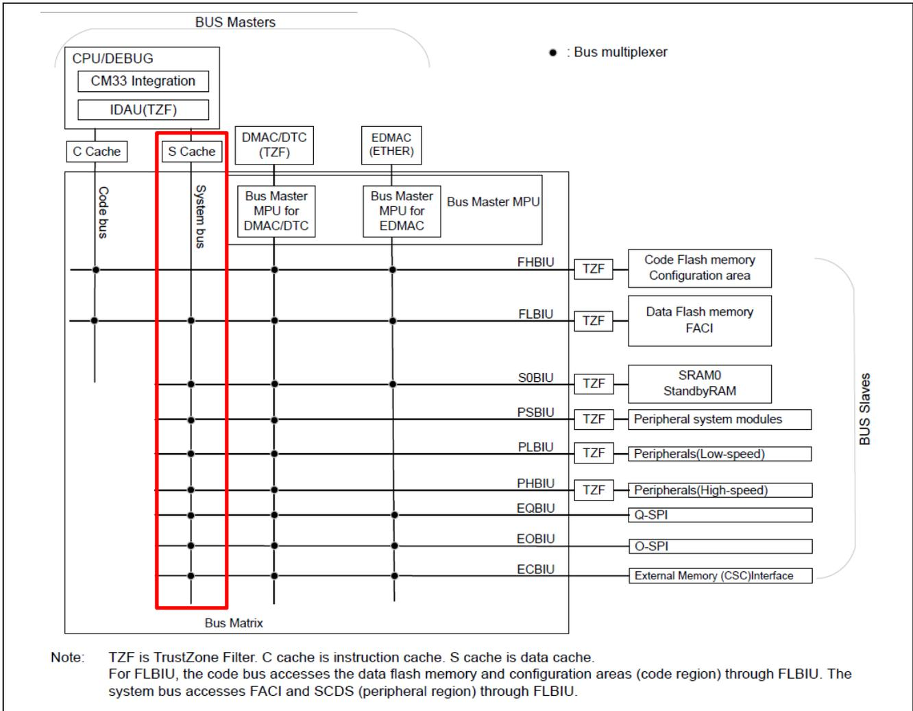
Figure 1. Bus Architecture for RA6M4 and RA6M5
