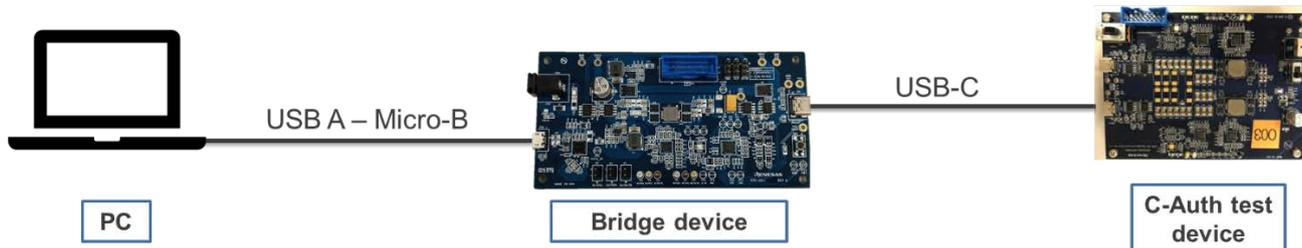
Figure 4-3 C-Auth Test Suite connection between PC and a test device
