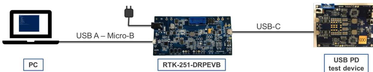
Figure 4-1 Exerciser connection with PC and a test device
