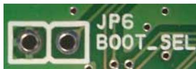
Figure 11 Switch Jumper (JP6) Serial Writer Function
