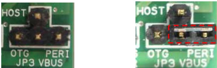
Figure 6 JP3 VBUS switch “Peripheral” setting
