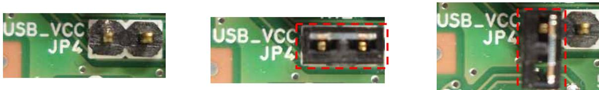
Figure 7 JP4 USB\_VCC switch Power supply “ON” (Short) setting Power supply “OFF” (Open) setting
