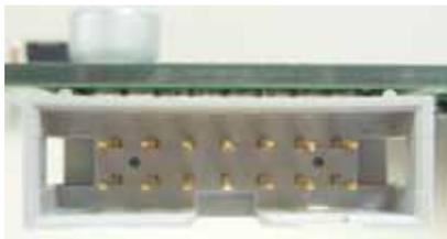
Figure 8 Connector for E8a Emulator (CN6)
