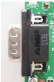
Figure 10 D-sub9 Pin Male Connector (CN5)
