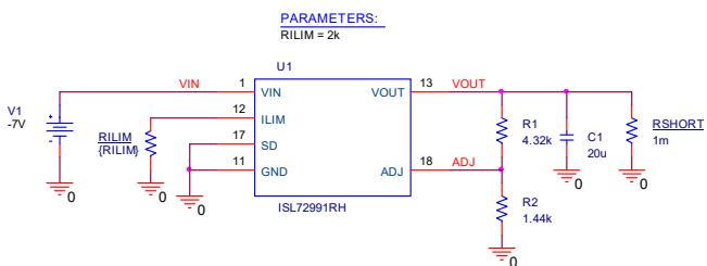
Figure 7. Short-Circuit Current Limiting PSpice Circuit
