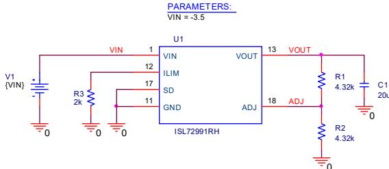
Figure 5.  $V_{REF}$  vs  $-V_{IN}$  PSpice Circuit
