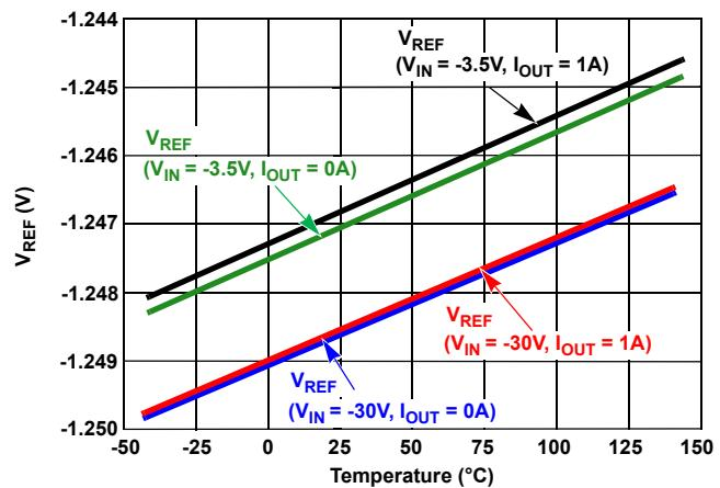
Figure 10.  $V_{REF}$  vs  $V_{IN}$  and Temperature
