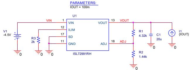
Figure 6. Dropout Voltage vs Output Current PSpice Circuit
