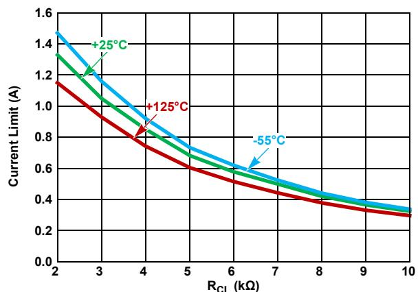
**Figure 16. I<sub>SC</sub> -12V<sub>IN</sub>, -5V<sub>OUT</sub> (Characterization Results)**
