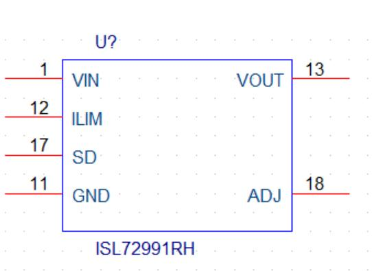
**Figure 1. ISL72991RH Sub-Circuit (ISL72991RH.OLB)**
