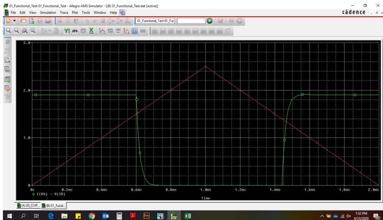
Figure 4. ISL72991RH PSpice General Functional Turn-Off/Turn-On Simulation Results
