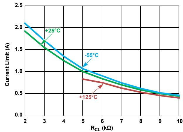
Figure 20.  $I_{SC}$  -20V<sub>IN</sub>, -10V<sub>OUT</sub> (Characterization Results)
