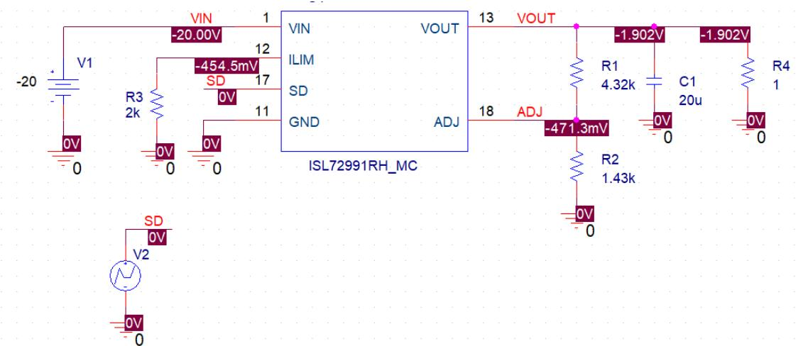
Figure 3. ISL72991RH PSpice General Functional Test Schematic
