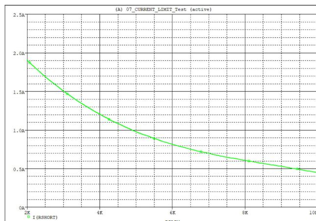
Figure 19.  $I_{SC}$  -20V<sub>IN</sub>, -10V<sub>OUT</sub> (PSpice Results)
