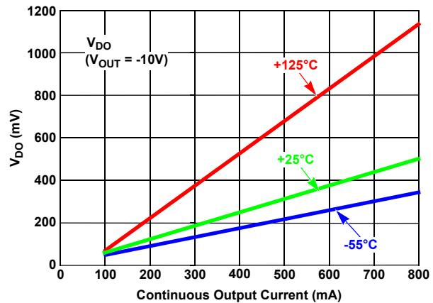
**Figure 12. Dropout Voltage vs Output Current (Characterization Results)**
