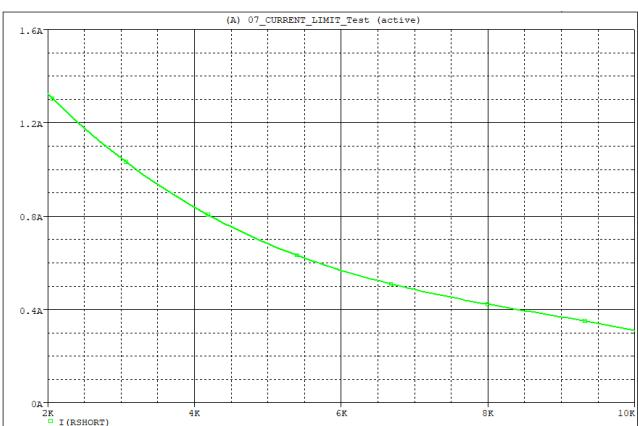
**Figure 15. I<sub>SC</sub> -12V<sub>IN</sub>, -5V<sub>OUT</sub> (PSpice Results)**
