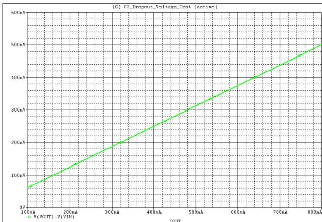
**Figure 11. Dropout Voltage vs Output Current (PSpice Results)**
