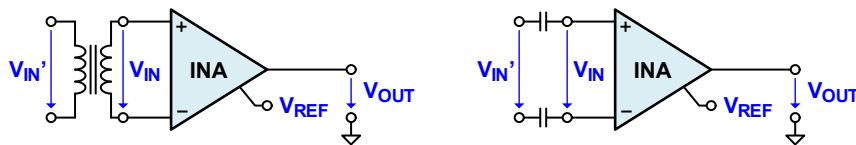
Figure 6. AC-Coupling Removes the Ground Reference of the Original Input Signal, V_{IN}' , so that V_{IN} is Floating
