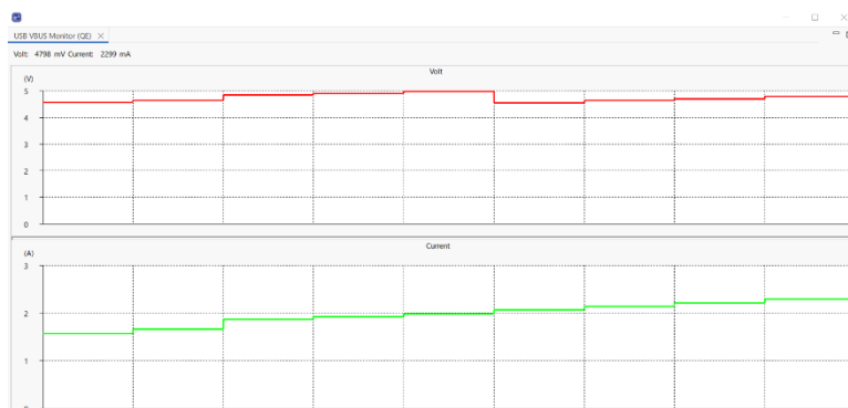
Figure 8-1 Checking Current and Voltage Supplied through USB Type-C
