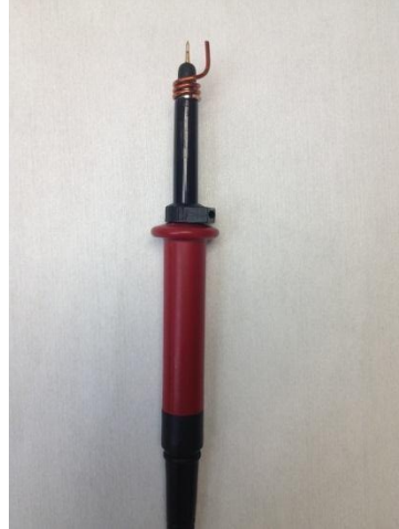
Fig.7 Probe with short ground lead – should be used
