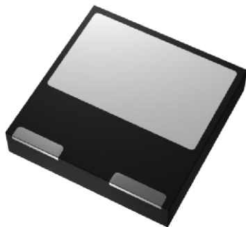
Figure 10. TPH320xLDG – common drain package configuration (bottom view)
