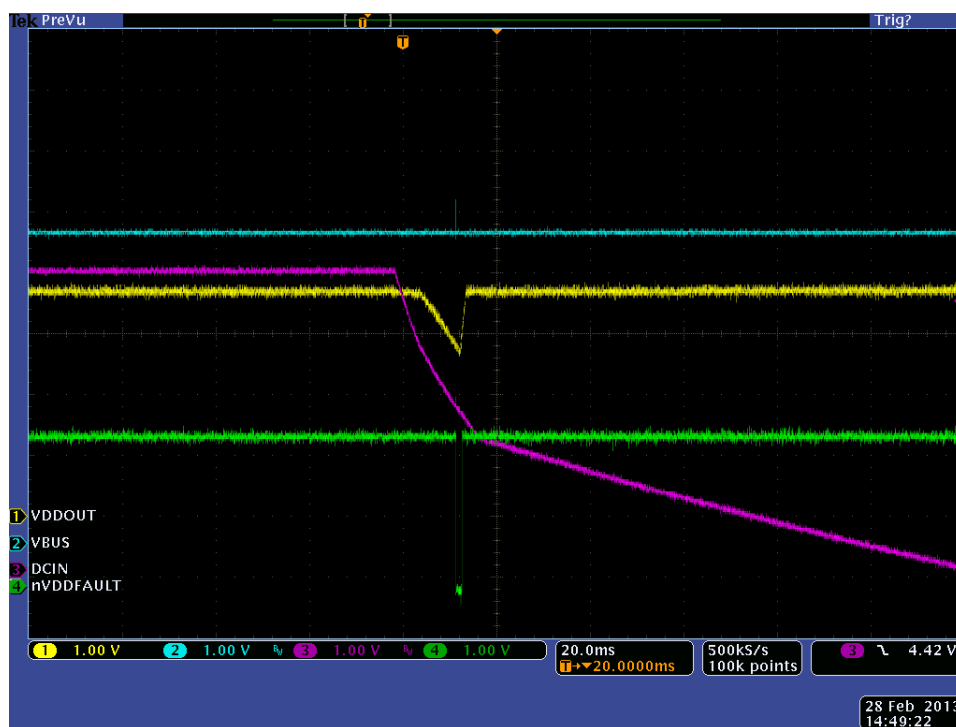
Figure 3 A 30 mA load is added on VBUCKCORE, 100 \mu F capacitor on VDDOUT
