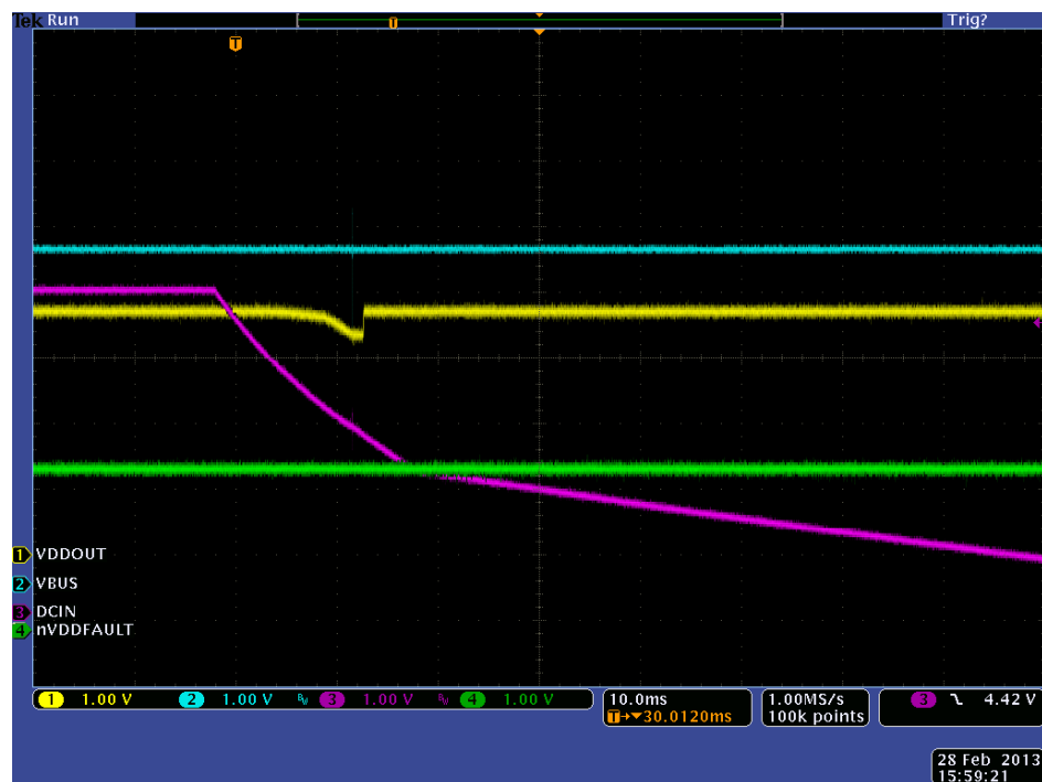
Figure 2 No load on VBUCKCORE
