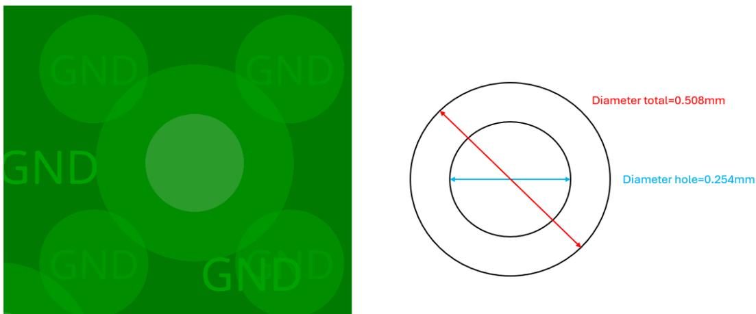
Figure 32. 9QXL1200 GND Plane – Via Implementation
