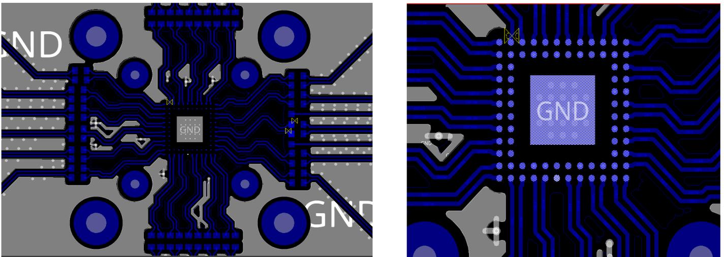
Figure 21. 9QXL2001 Differential Traces Layout (top layer)
