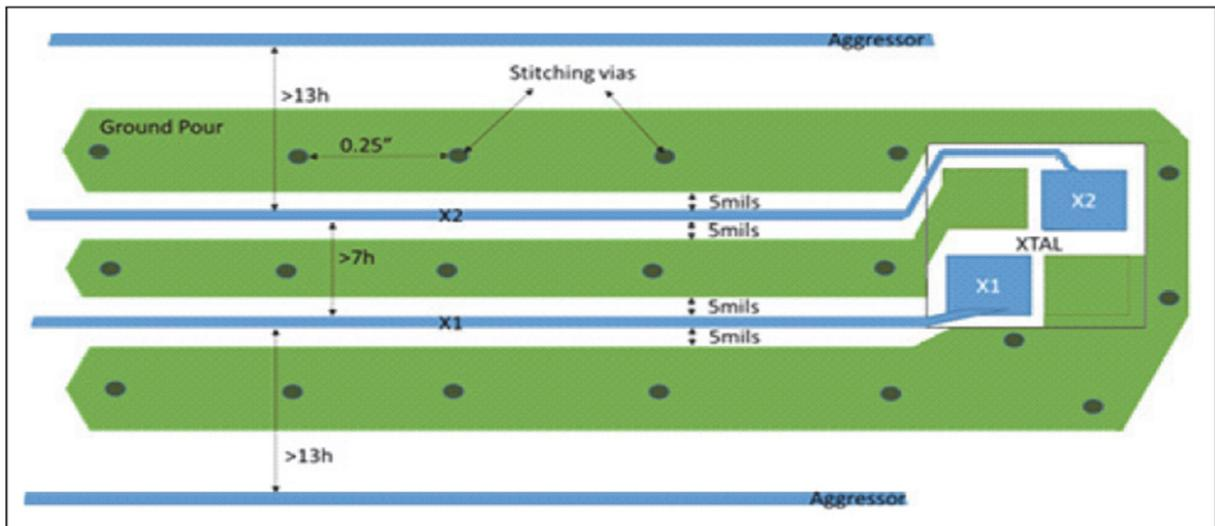
Figure 27. GND Shielding Layout Practices – XTAL Example
