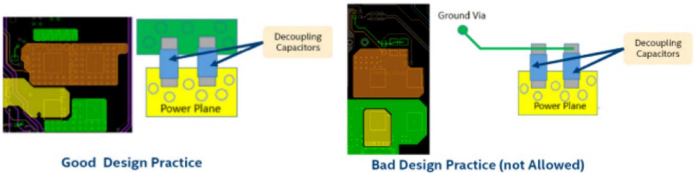
Figure 12. Power-GND Plane + Decoupling Capacitors Layout Practices
