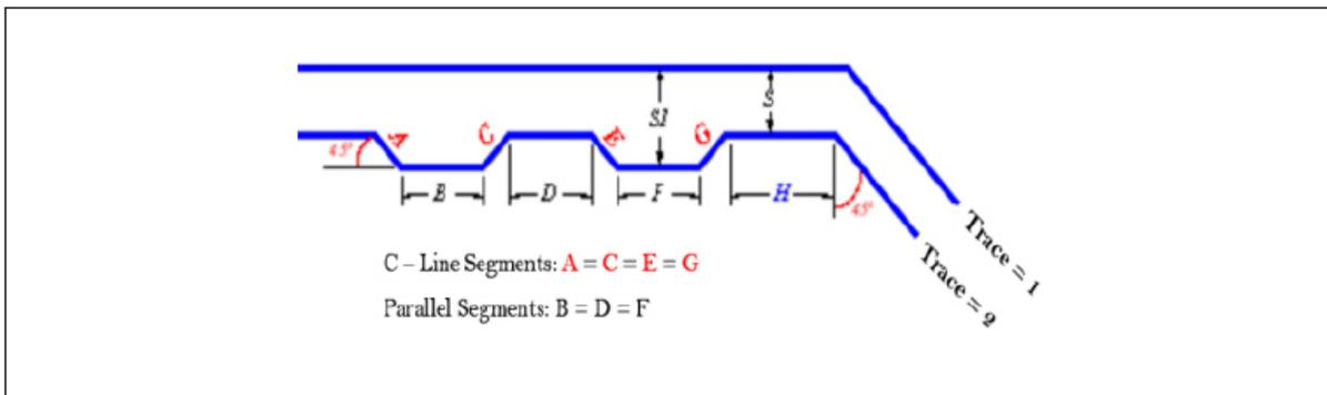
**Figure 17. Serpentine Differential Mismatched Length Compensation**
