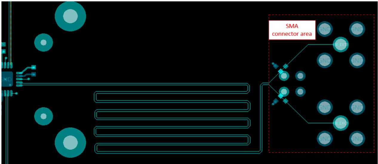
Figure 20. 9DBL0455 EVB Differential Traces Layout (2)
