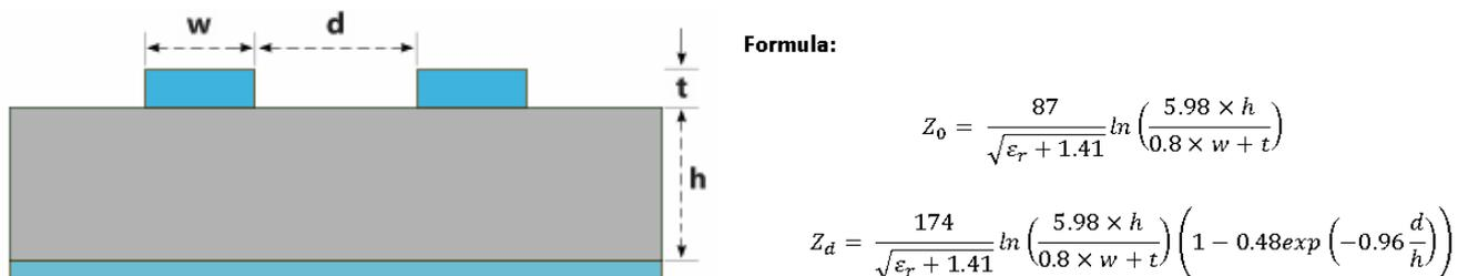
Figure 5. Microstrip Profile – Impedance Calculation
