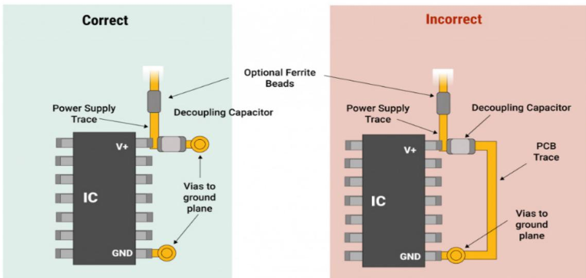
Figure 11. Power Filtering Layout Practices
