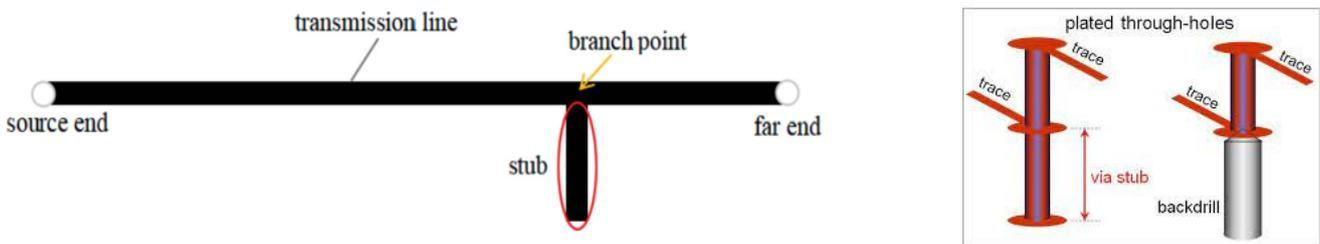
Figure 8. Stub PCB Layout
