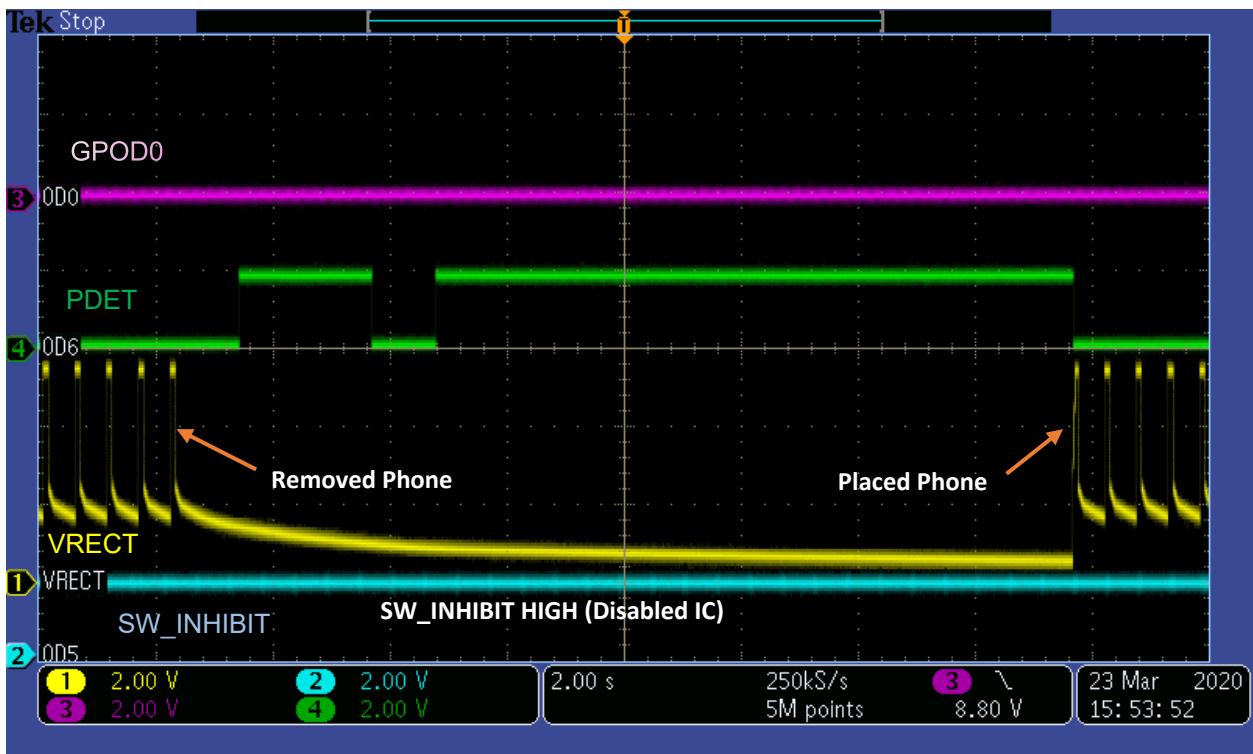
Figure 3. Waveform of PDET (OD6) Output Indicating Rx Removal and Placement with SW_Inhibited.
