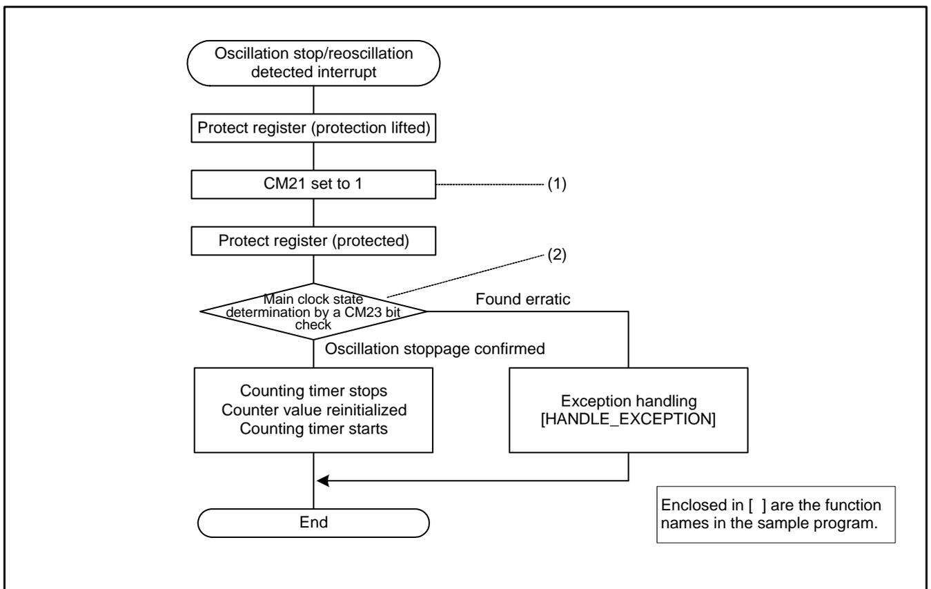
Figure 2. Oscillation Stop/Reoscillation Detected Interrupt Handling Flowchart
