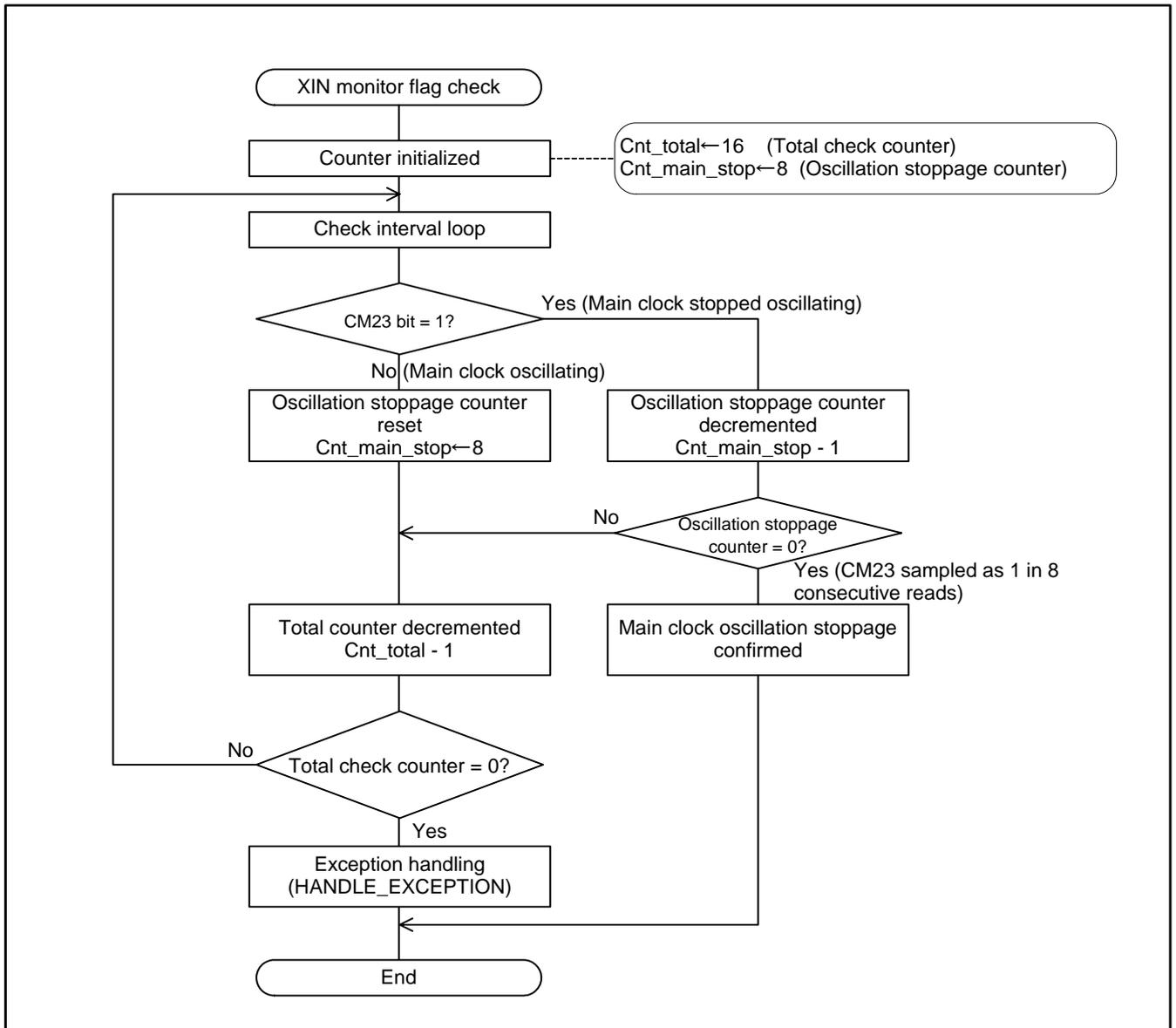
Figure 3. CM23 Bit (XIN Monitor Flag) Check Flowchart
