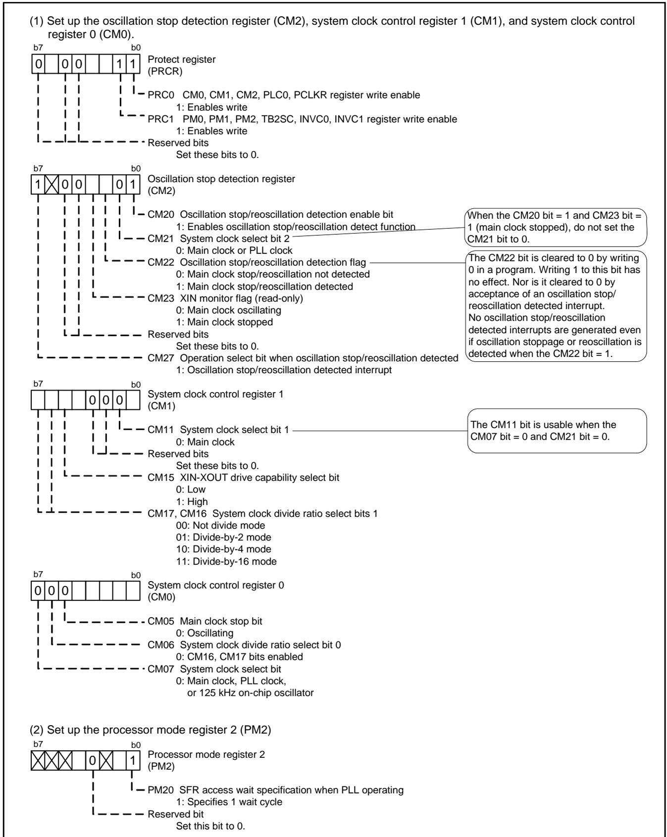
Figure 4. Procedure for Setting Up the Registers to Use the Oscillation Stop/Reoscillation Detect Function (1)
