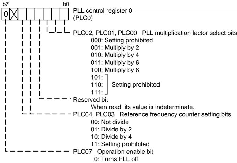
To set up the PLL control register (PLC0), write to it when the PLC07 bit = 0 (PLL turned off).
