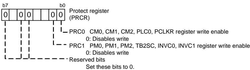
Figure 5. Procedure for Setting Up the Registers to Use the Oscillation Stop/Reoscillation Detect Function (2)
