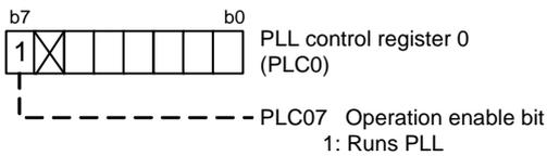
Before setting the PLC07 bit to 1 (PLL operating), set the CM05 bit to 0 (main clock oscillating) first.
