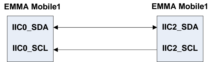
Figure 3-4 Hardware Connection of Write and Read as a Slave
