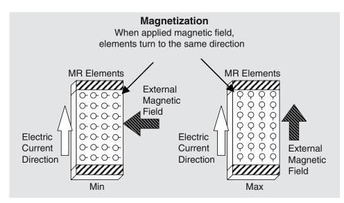
Figure 2-3 Resistance value vs Magnetic field direction
