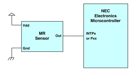
Figure 3-3 MR sensor typical connexion for open/close detection
