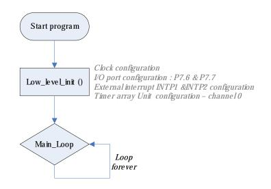
Figure 4-8 Main processing overview flowchart
