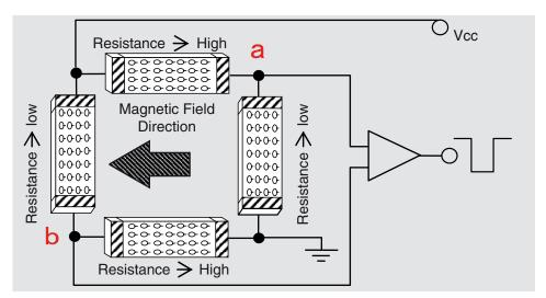
Figure 2-4 MR Sensor operation
