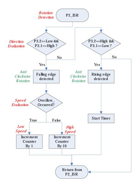
Figure 4-11 INTP2 interrupt flowchart
