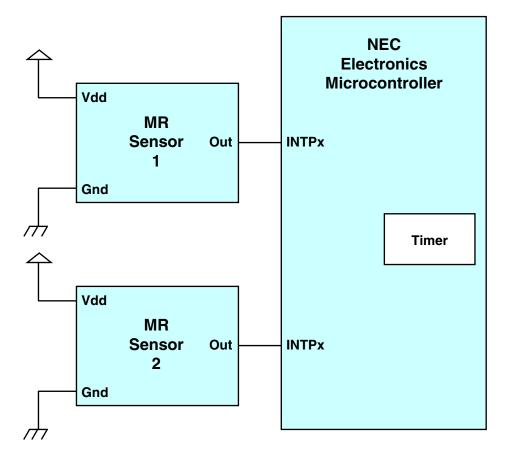
Figure 4-7 MR sensor typical connexion for jog dial application
