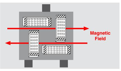
Figure 2-6 Horizontal operating magnetic field
