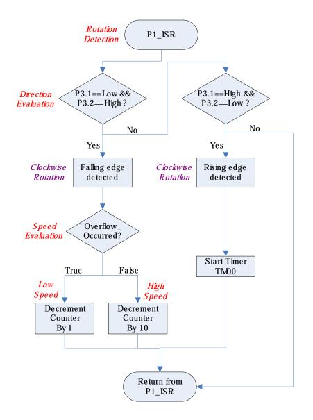
Figure 4-10 INTP1 interrupt flowchart
