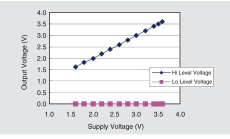
Figure 2-5 Output level voltage VS Supply voltage
