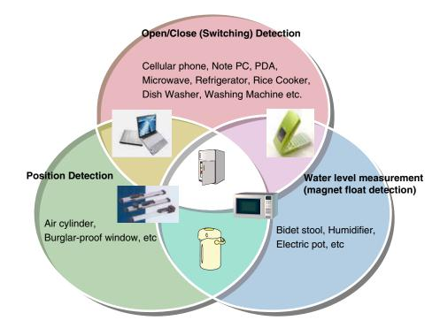
Figure 2-10 Examples of MR sensor applications
