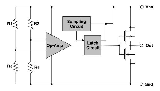
Figure 2-2 MR Sensor equivalent block diagram
