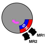
Figure 4-5 Detection of direction with two MR sensors
