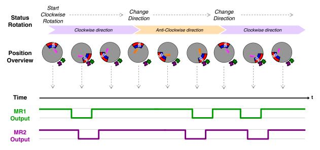
Figure 4-6 MR sensor output waveforms depending of direction
