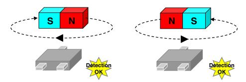
Figure 2-7 Dual operating magnetic pole
