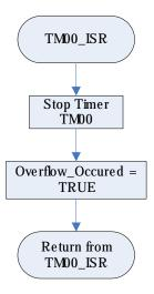
Figure 4-9 TM00 interrupt flowchart
