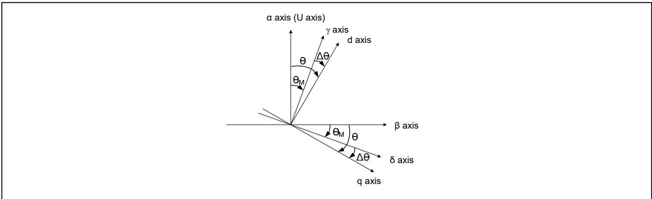
**Figure 3-4 Relation between d q axis and  $\gamma \delta$  axis**
