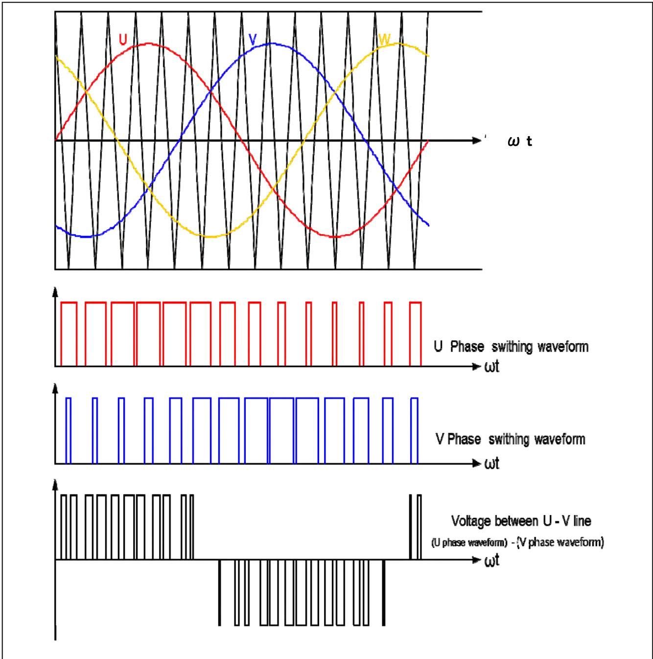
Figure 3-6 Conceptual diagram of the triangular wave comparison method
