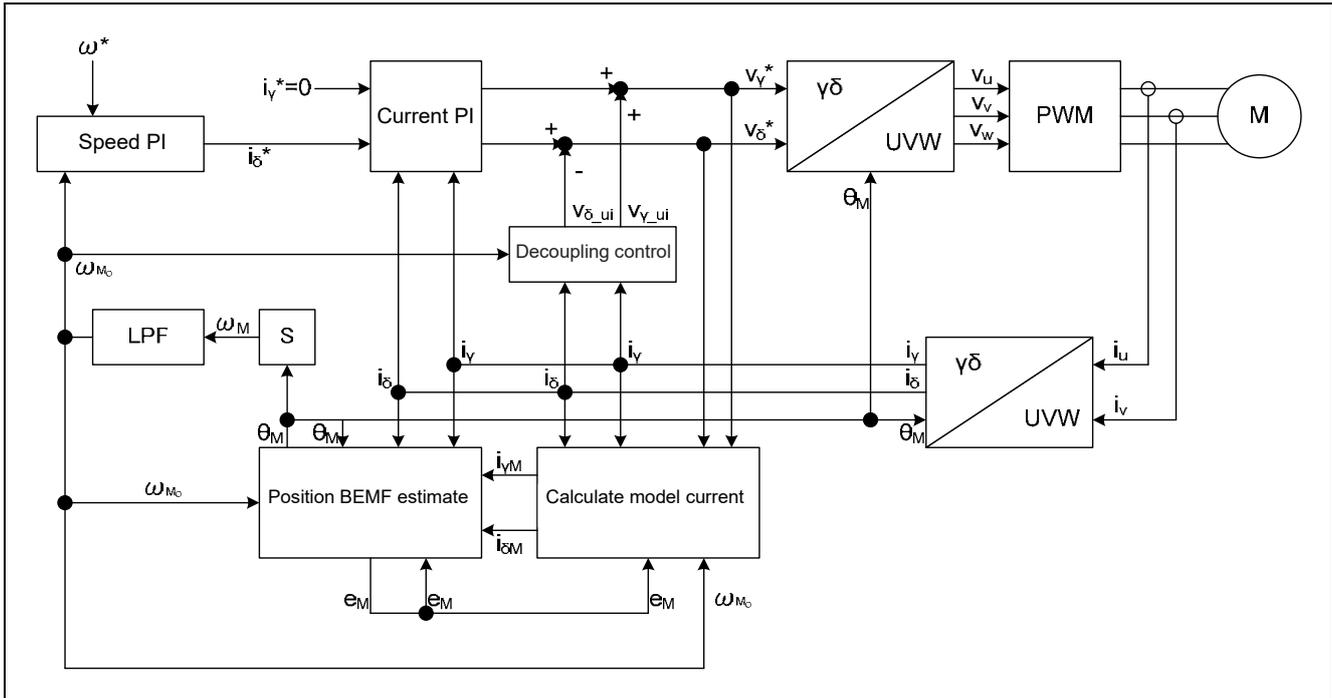
Figure 3-5 Control flow of the sensorless vector control based on the current estimation error method
