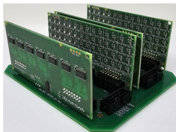
Figure 2. Example Setup with 4 HSx PCBs Connected
