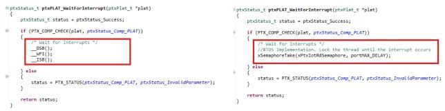
Figure 8. ptxPLAT\_WaitForInterrupt Implementation
