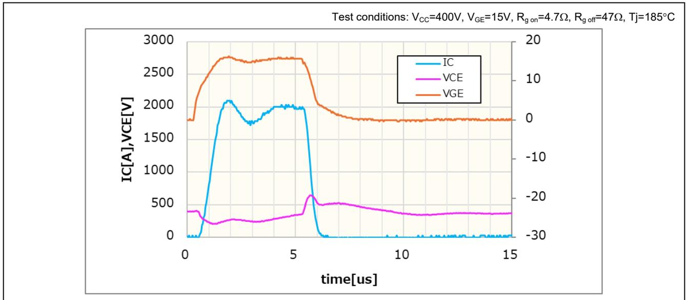
Figure 3-5 Short-circuit Waveform (AE5)
