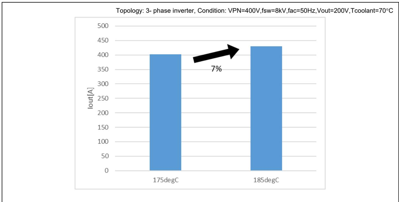
Figure 1-1 Output Current Value During Inverter Operations (AE5  $175^{\circ}\text{C}$  vs.  $185^{\circ}\text{C}$ )
