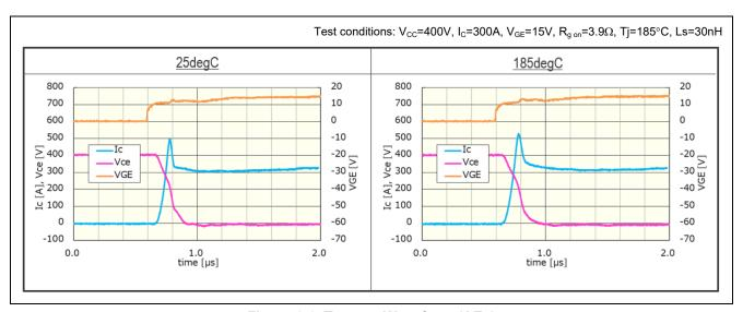
Figure 3-3 Turn-on Waveform (AE5)
