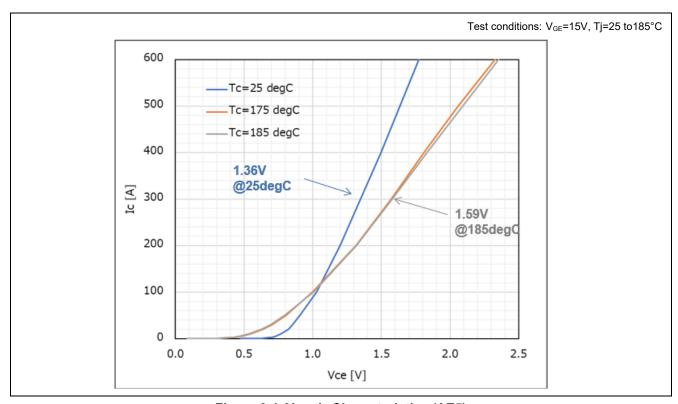
Figure 3-1 V<sub>CE</sub> - I<sub>C</sub> Characteristics (AE5)
