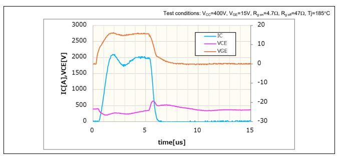
Figure 3-5 Short-circuit Waveform (AE5)
