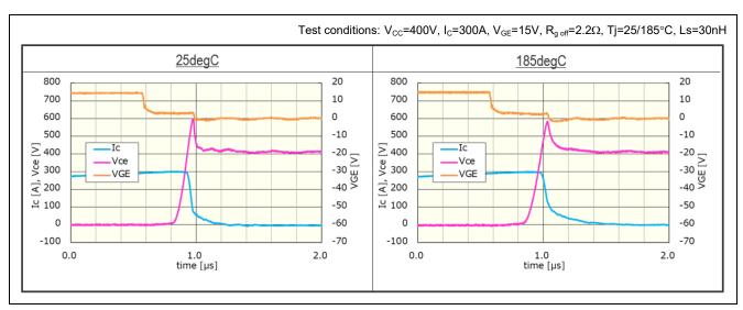
Figure 3-2 Turn-off Waveform (AE5)
