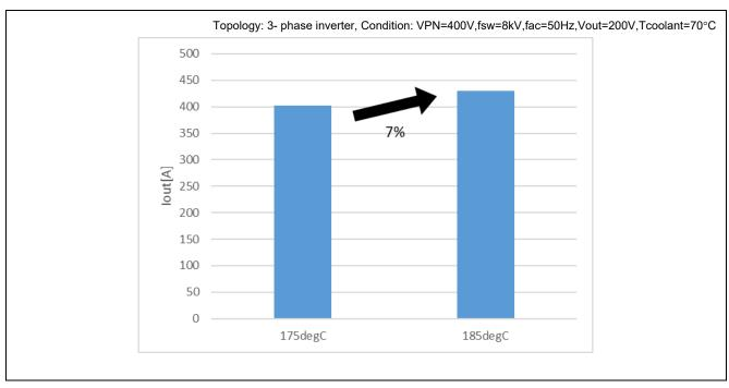
Figure 1-1 Output Current Value During Inverter Operations (AE5 175°C vs. 185°C)
