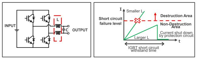
Figure 1-2 Conceptual of tsc with inductor
