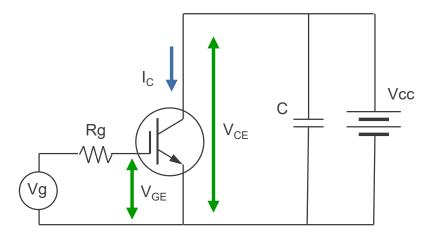
Figure 1-3 Circuit diagram for LSC
