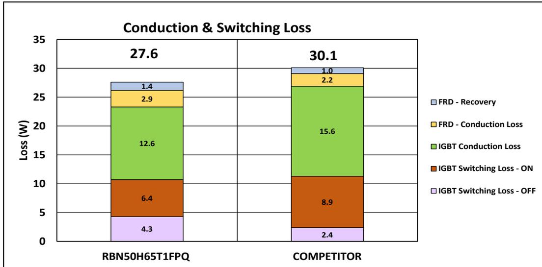
Figure 3-3 Conduction & Switching Loss Comparison
