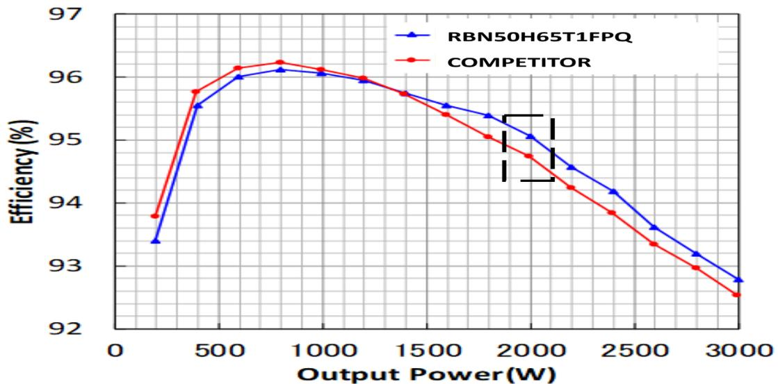
Figure 3-2 Output Power versus Efficiency Change
