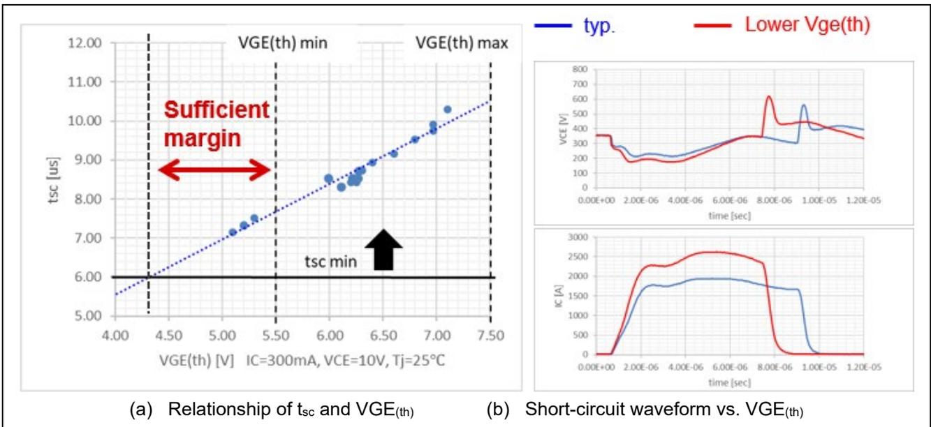
Figure 3-2 Relationship Between  $t_{sc}$  and  $V_{GE(th)}$  and Short-circuit Waveform Examples
