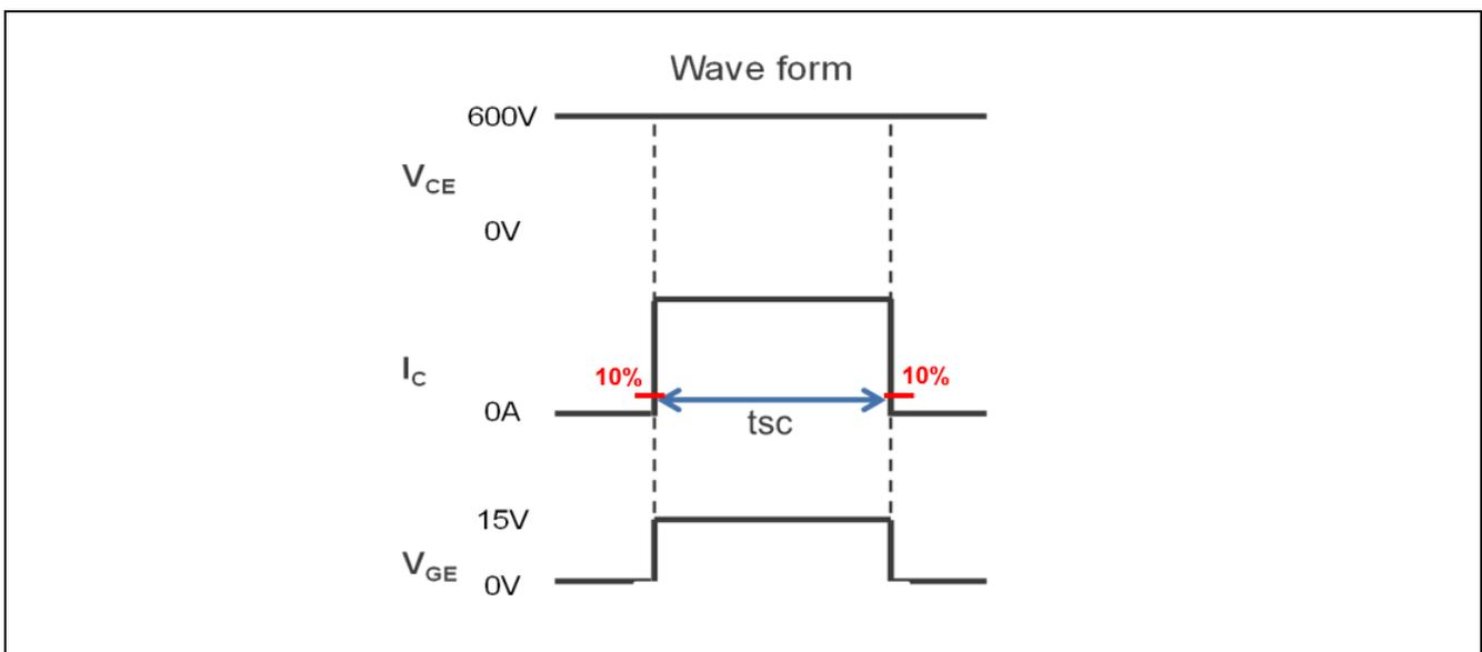
Figure 1-2 Simplified Example of Short-circuit Wave Form
