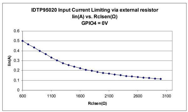
Figure 3 - Typical Input Current Limiting via external resistor, GPIO4=GND
