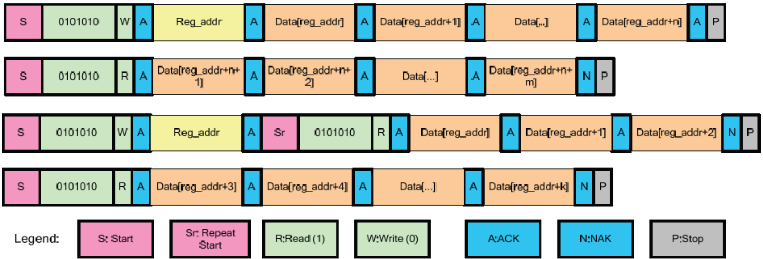
Figure 4 - I 2 C Read/Write Operation
