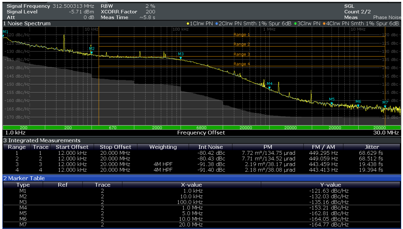
Figure 8. Phase Noise Plot of a 312.5MHz Output from an RC38312 FC3W Device Operating in Jitter Attenuator Mode using a 49.152MHz Crystal with an APLL VCO Frequency of 9.375GHz and a 25MHz + 1ppm Reference Input; measured using a Rohde & Schwarz FSWP. Range 1 and 2 show Unfiltered RMS Jitter. Range 3 and 4 show RMS Jitter with a 4MHz High-Pass Filter applied
