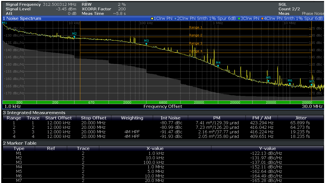
Figure 2. Phase Noise Plot for a 312.5MHz Output from an RC32312 FC3 Device Operating in Jitter Attenuator Mode, using a 49.152MHz Crystal along with an APLL VCO Frequency of 10GHz, and a 25MHz + 1ppm Reference Input, measured using a Rohde & Schwarz FSWP; RMS Jitter also displayed
