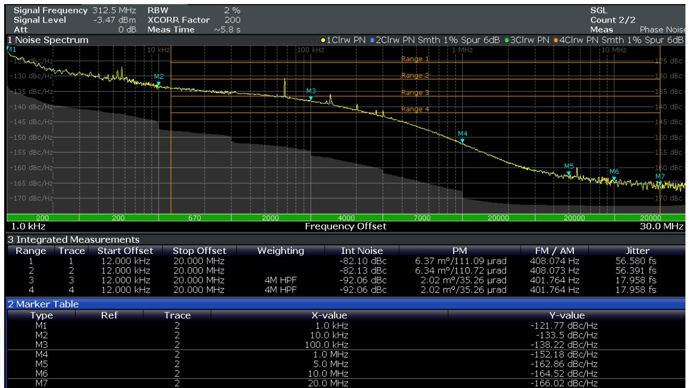
Figure 1. Phase Noise Plot for a 312.5MHz Output from an RC32312 FC3 Device Operating in Synthesizer Mode, using a 62.5MHz Crystal along with an APLL VCO Frequency of 10GHz, measured using a Rohde & Schwarz FSWP; RMS Jitter also displayed
