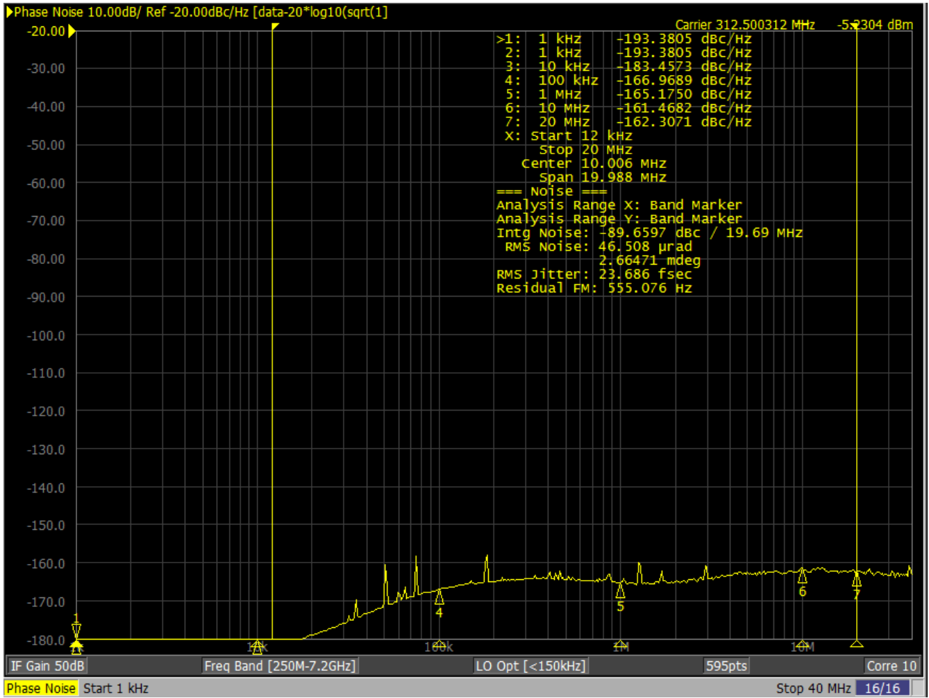
Figure 12. Phase Noise Plot using a Keysight E5052B to Approximate the Effects of a 4MHz High-Pass Filter on a 312.5MHz Output from an RC38312 FC3W Device Operating in Jitter Attenuator Mode using a 49.152MHz crystal, and a 25MHz + 1ppm Reference Clock Input; RMS jitter also displayed
