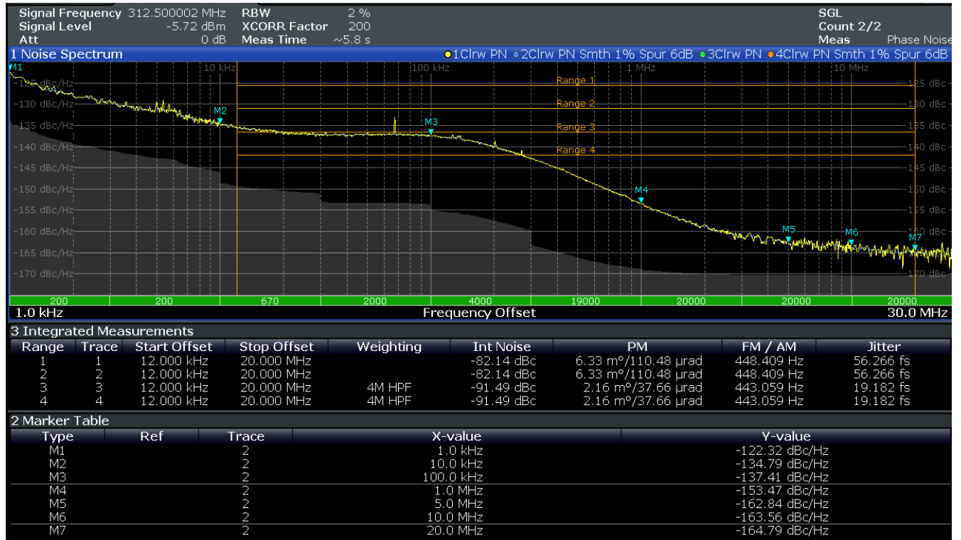
Figure 7. Phase Noise Plot of a 312.5MHz Output from an RC38312 FC3W Device Operating in Synthesizer Mode using a 62.5MHz Crystal with an APLL VCO Frequency of 9.375GHz; measured using a Rohde & Schwarz FSWP. Range 1 and 2 show Unfiltered RMS Jitter. Range 3 and 4 show RMS Jitter with a 4MHz High-Pass Filter applied
