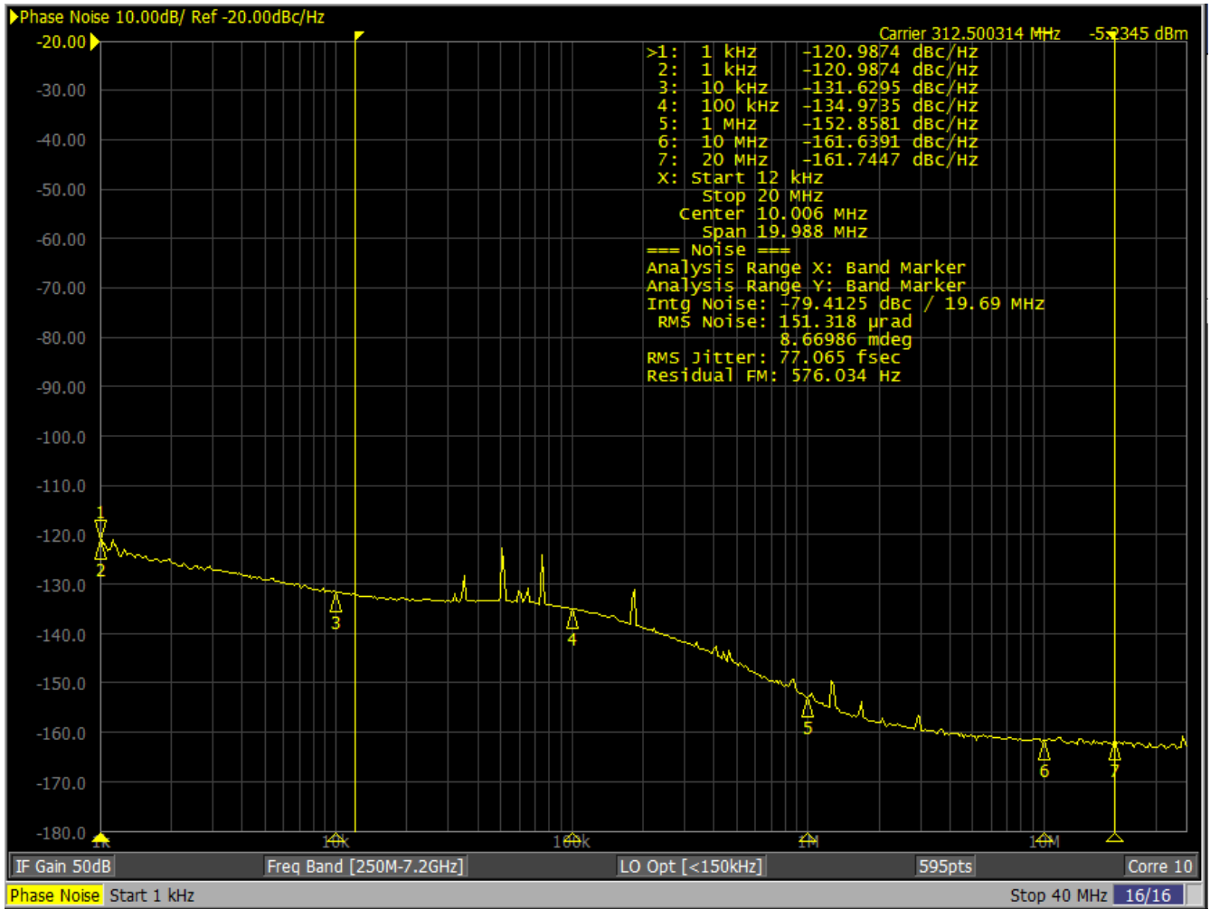
Figure 11. Phase Noise Plot for a 312.5MHz Output from an RC38312 FC3 Device Operating in Jitter Attenuator Mode using a 49.152MHz Crystal along with an APLL VCO Frequency of 9.375GHz, and a 25MHz + 1ppm Reference Clock Input; RMS Jitter also displayed
