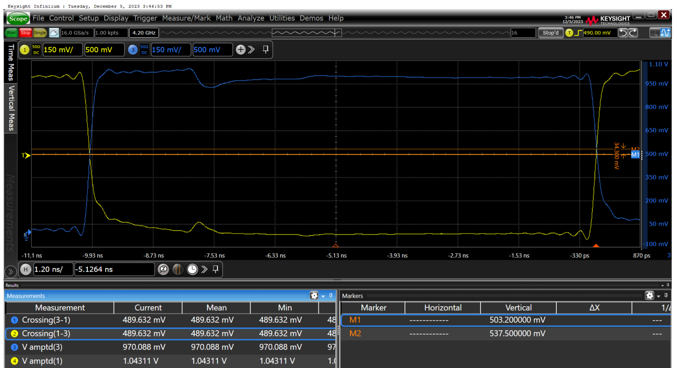
Figure 21. Vcross-HCSL Internal Termination SWING = 950mV on OUT11
