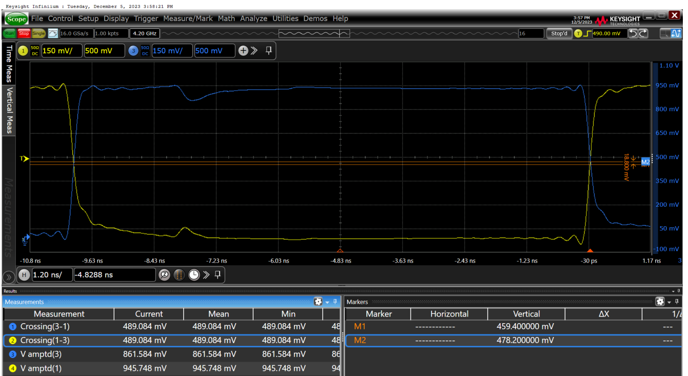
Figure 15. Vcross–HCSL Internal Termination SWING = 850mV on OUT11
