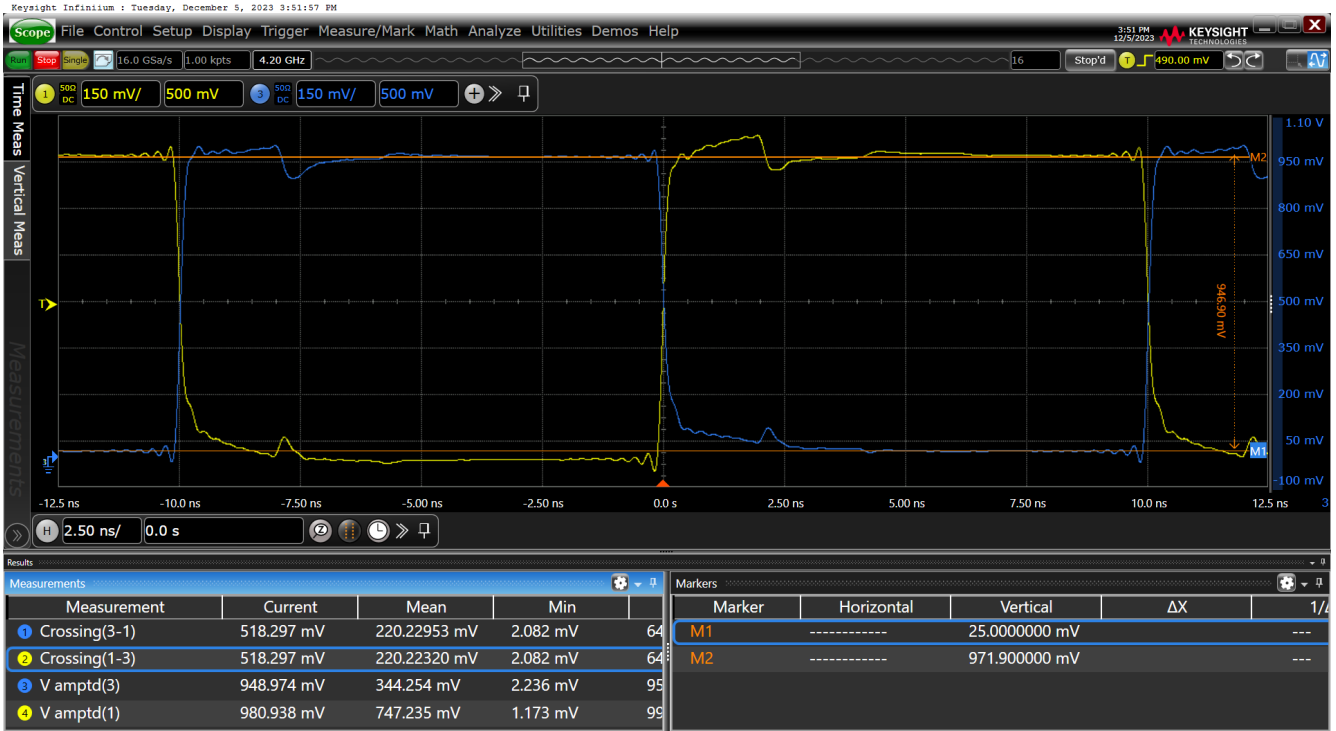
Figure 16. Vovs–HCSL Internal Termination SWING = 900mV on OUT11
