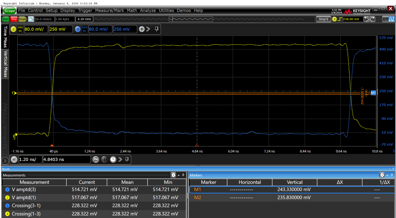
Figure 45. Vcross-HCSL Dual-Termination SWING = 950mV on OUT11
