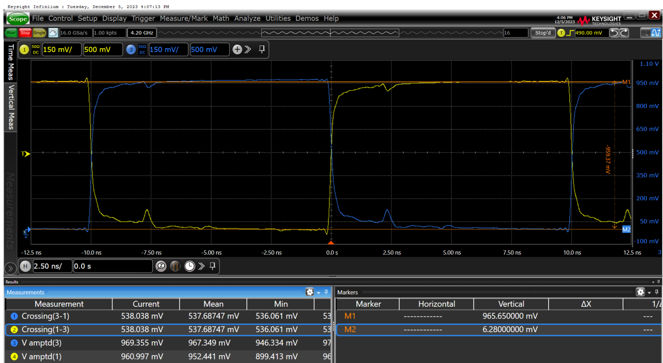
Figure 31. Vovs–HCSL External Termination SWING = 950mV on OUT11
