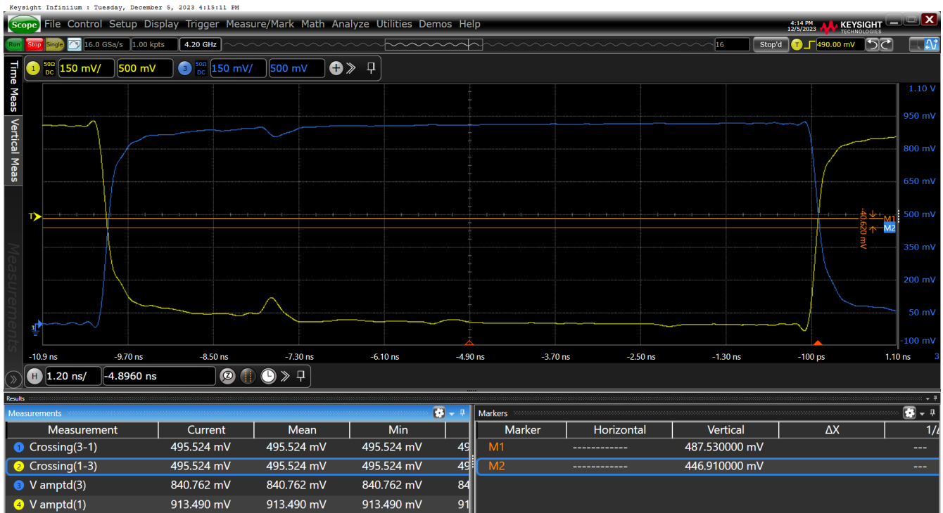
Figure 27. Vcross-HCSL External Termination SWING = 850mV on OUT11
