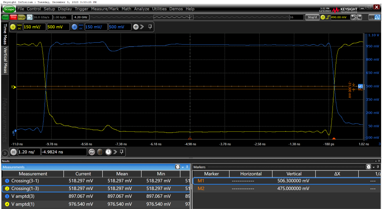
Figure 18. Vcross–HCSL Internal Termination SWING = 900mV on nOUT
