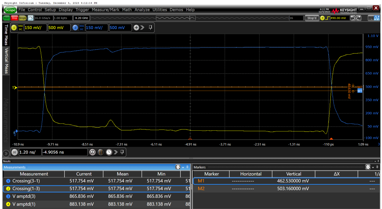
Figure 30. Vcross–HCSL External Termination SWING = 900mV on OUT11
