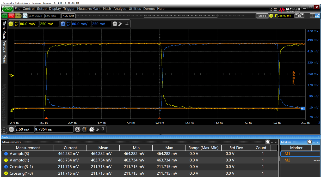
Figure 37. Vovs-HCSL Dual-Termination SWING = 850mV on OUT11
