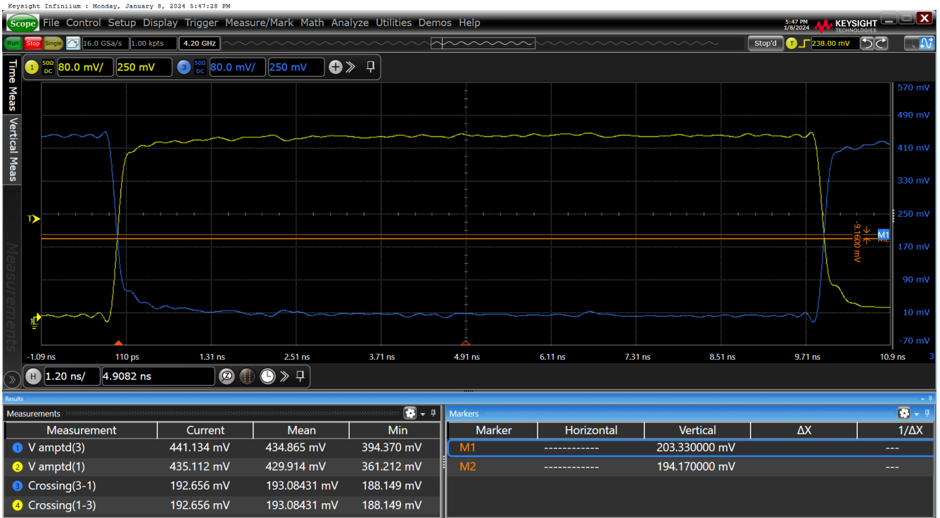
Figure 36. Vcross-HCSL Dual-Termination SWING = 800mV on OUT11
