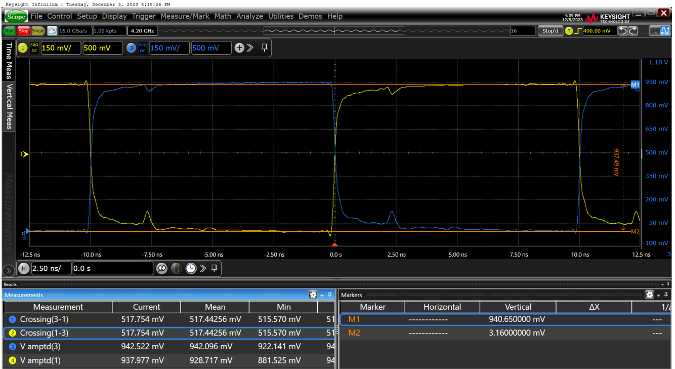
Figure 28. Vovs–HCSL External Termination SWING = 900mV on OUT11
