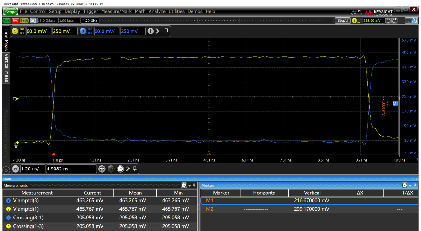
Figure 39. Vcross-HCSL Dual-Termination SWING = 850mV on nOUT11
