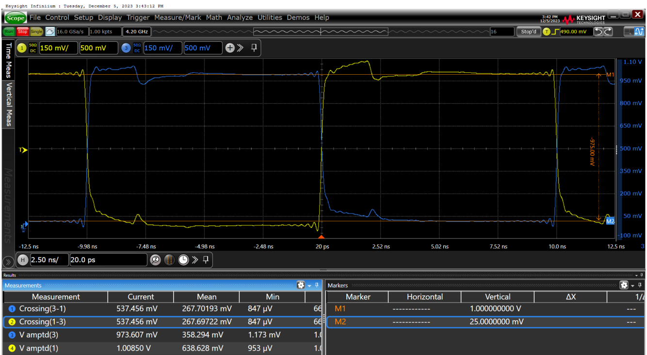
Figure 19. Vovs–HCSL Internal Termination SWING = 950mV on OUT11
