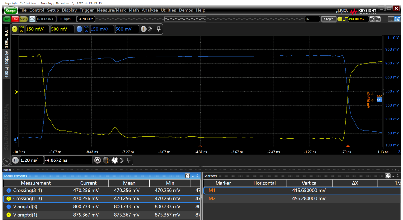
Figure 24. Vcross-HCSL External Termination SWING = 800mV on OUT11
