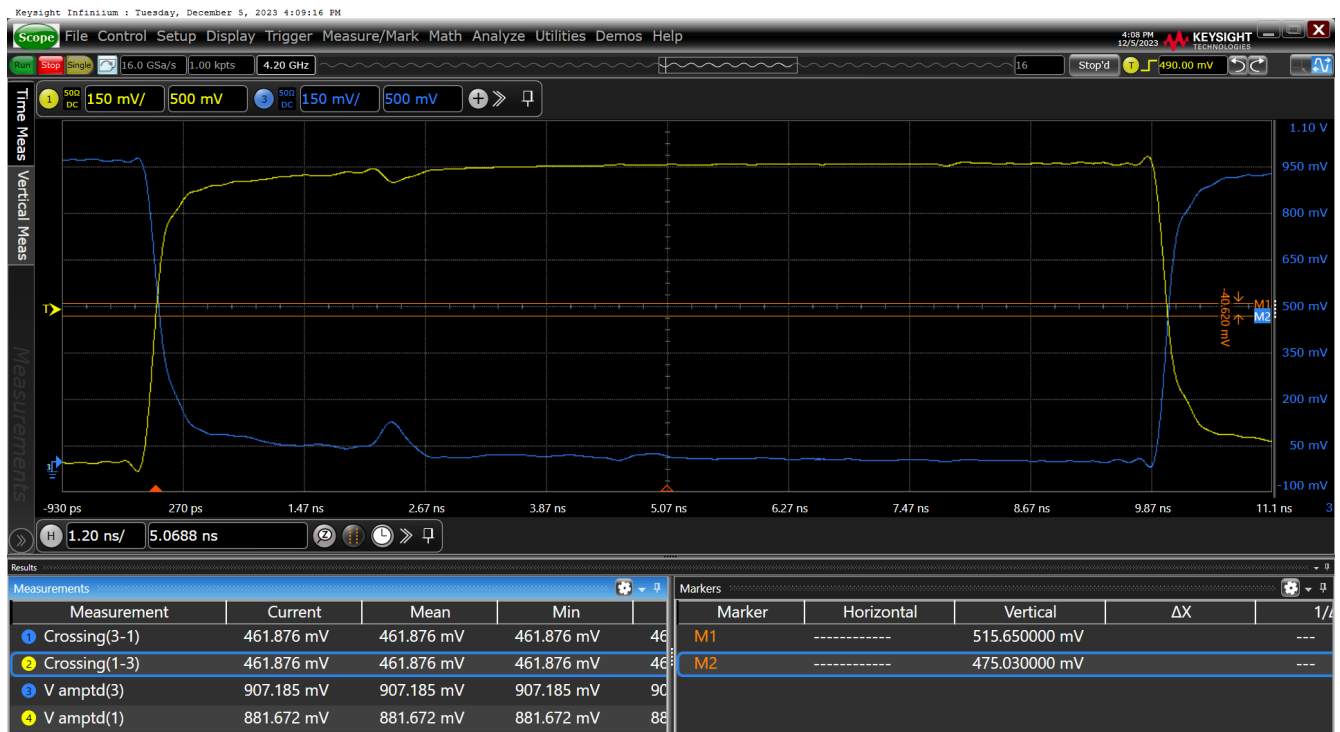
Figure 33. Vcross-HCSL External Termination SWING = 950mV on OUT11
