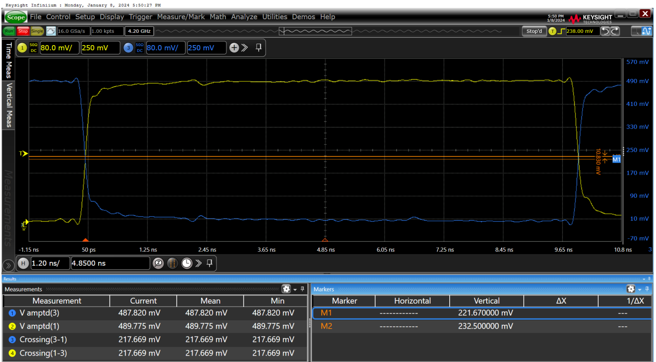
Figure 42. Vcross–HCSL Dual-Termination SWING = 900mV on OUT11
