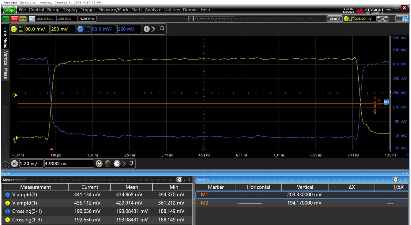
Figure 36. Vcross-HCSL Dual-Termination SWING = 800mV on OUT11
