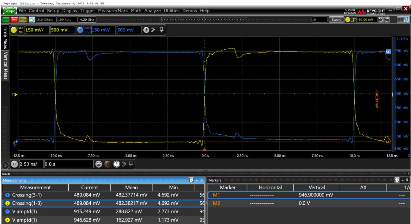
Figure 13. Vovs–HCSL Internal Termination SWING = 850mV on OUT11
