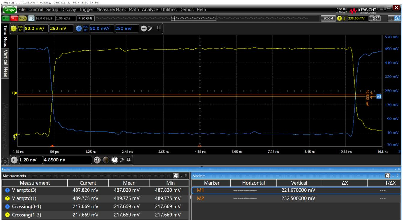
Figure 42. Vcross–HCSL Dual-Termination SWING = 900mV on OUT11
