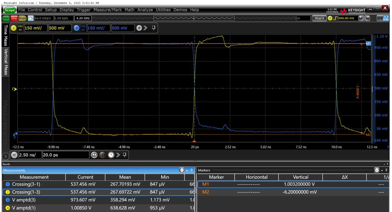
Figure 20. Vovs-HCSL Internal Termination SWING = 950mV on nOUT11
