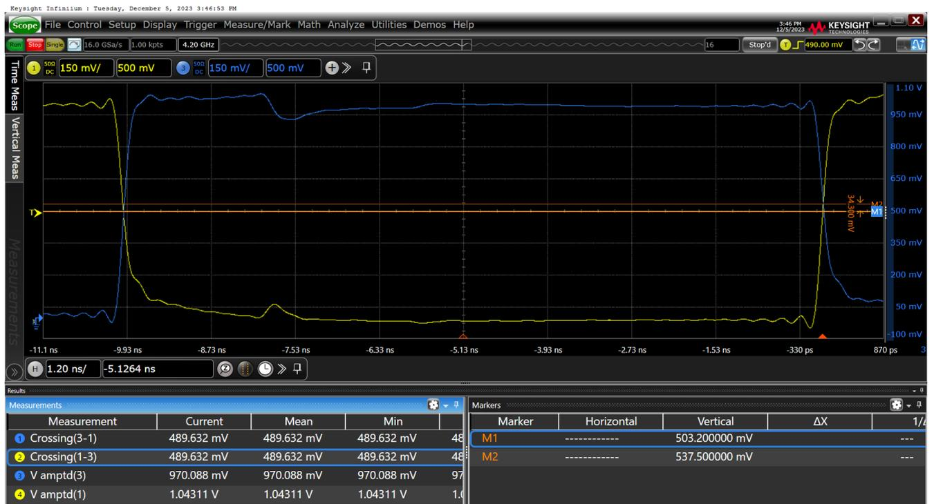
Figure 21. Vcross-HCSL Internal Termination SWING = 950mV on OUT11
