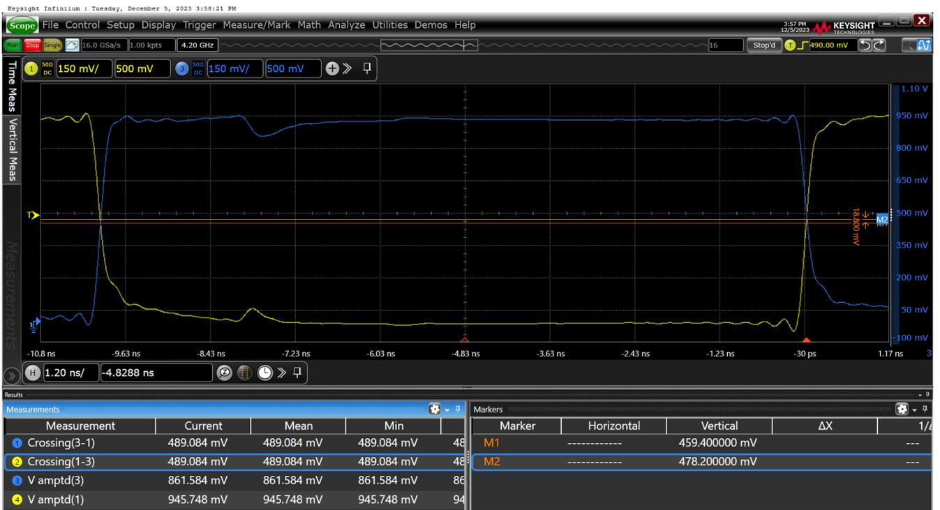
Figure 15. Vcross–HCSL Internal Termination SWING = 850mV on OUT11
