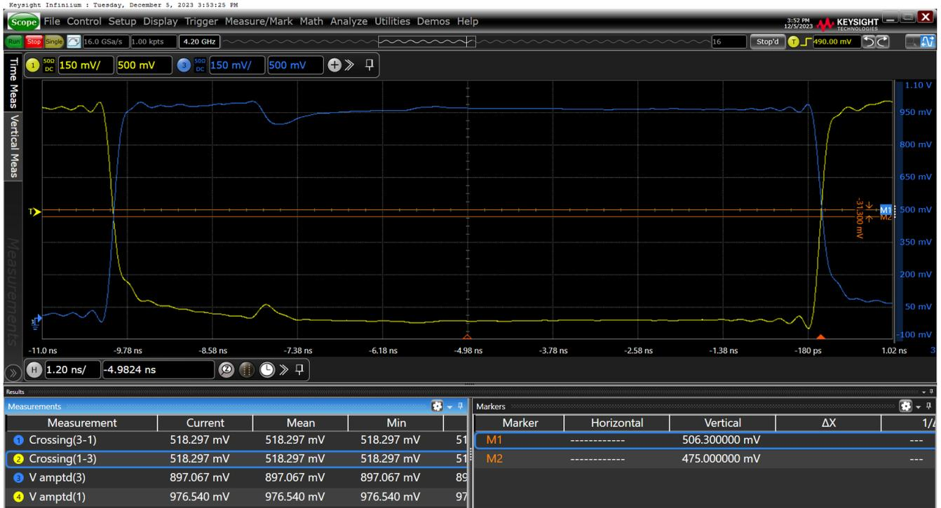
Figure 18. Vcross–HCSL Internal Termination SWING = 900mV on nOUT
