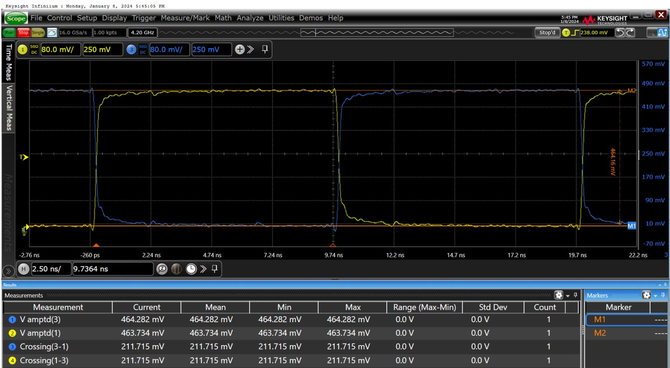
Figure 37. Vovs-HCSL Dual-Termination SWING = 850mV on OUT11
