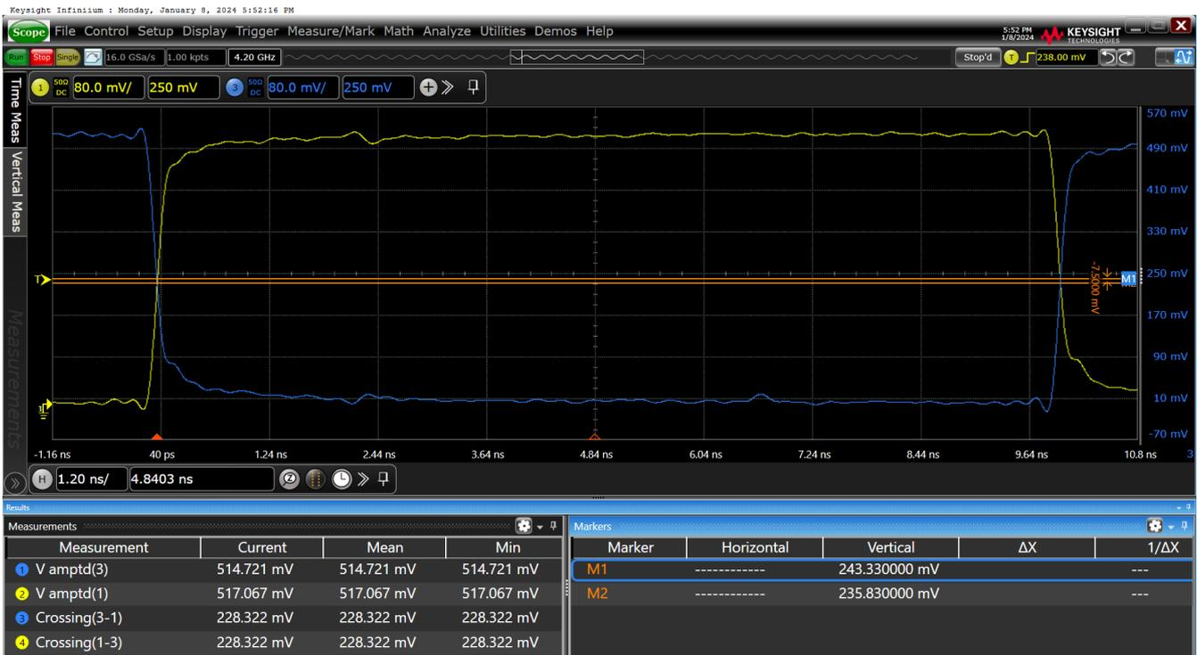
Figure 45. Vcross-HCSL Dual-Termination SWING = 950mV on OUT11
