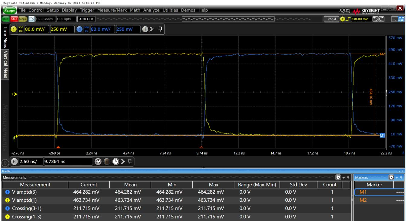
Figure 38. Vovs-HCSL Dual-Termination SWING = 850mV on nOUT11
