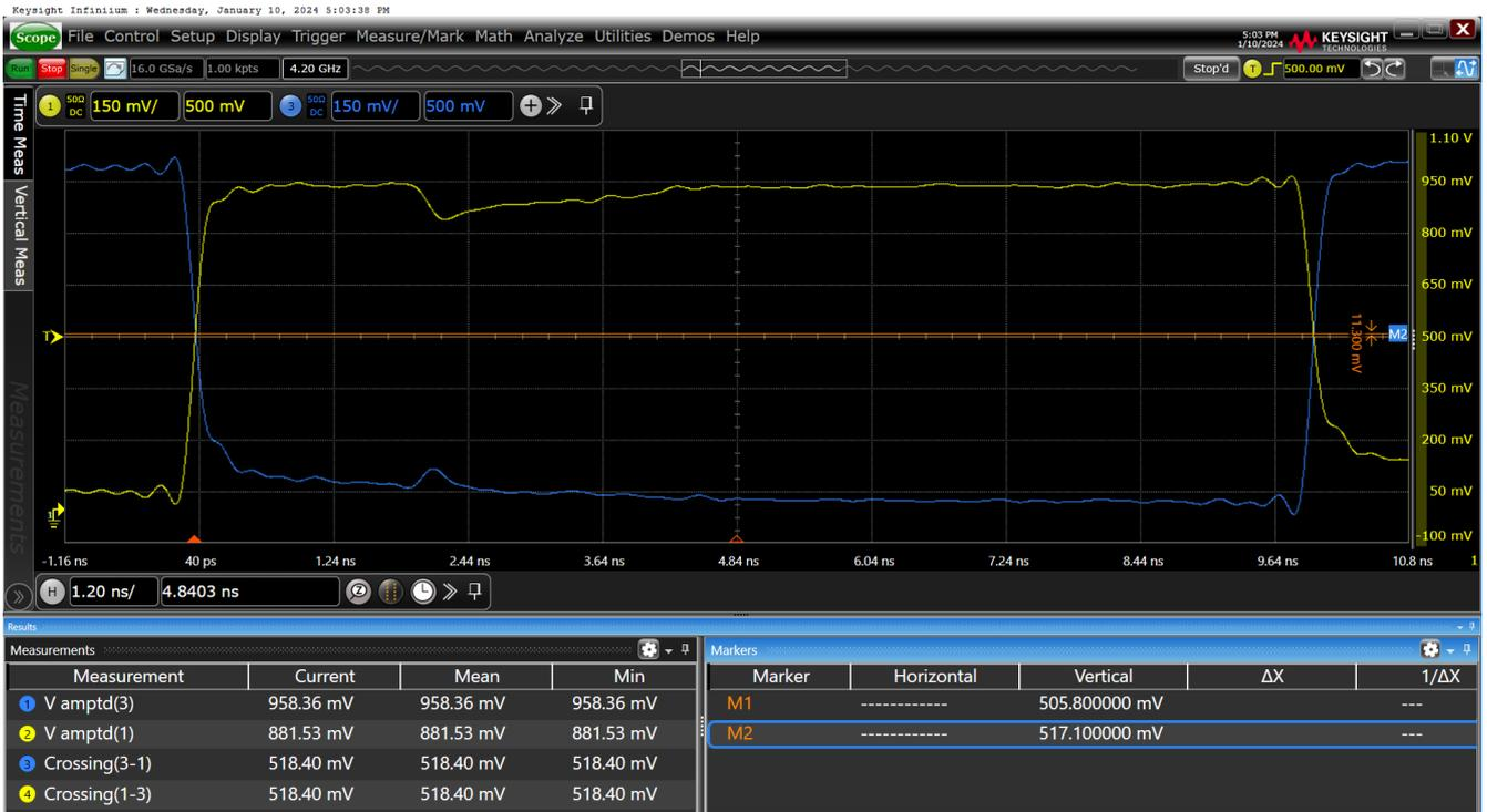
Figure 12. Vcross–HCSL Internal Termination SWING = 800mV on OUT11
