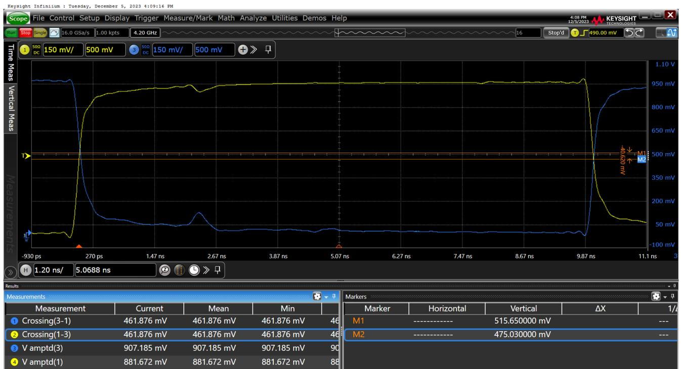
Figure 33. Vcross-HCSL External Termination SWING = 950mV on OUT11
