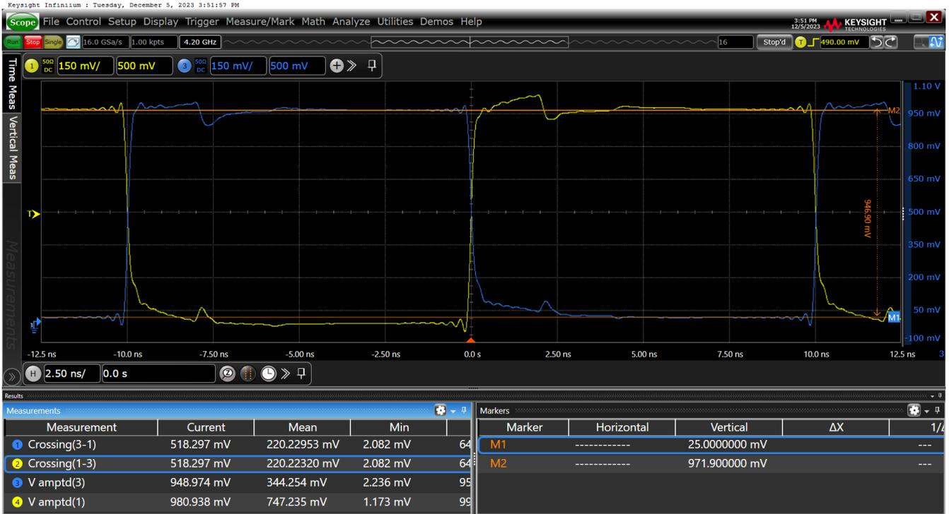
Figure 16. Vovs–HCSL Internal Termination SWING = 900mV on OUT11
