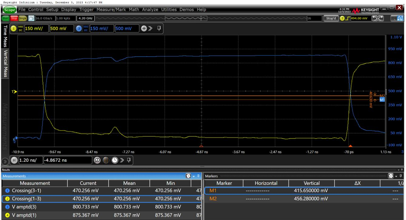
Figure 24. Vcross-HCSL External Termination SWING = 800mV on OUT11
