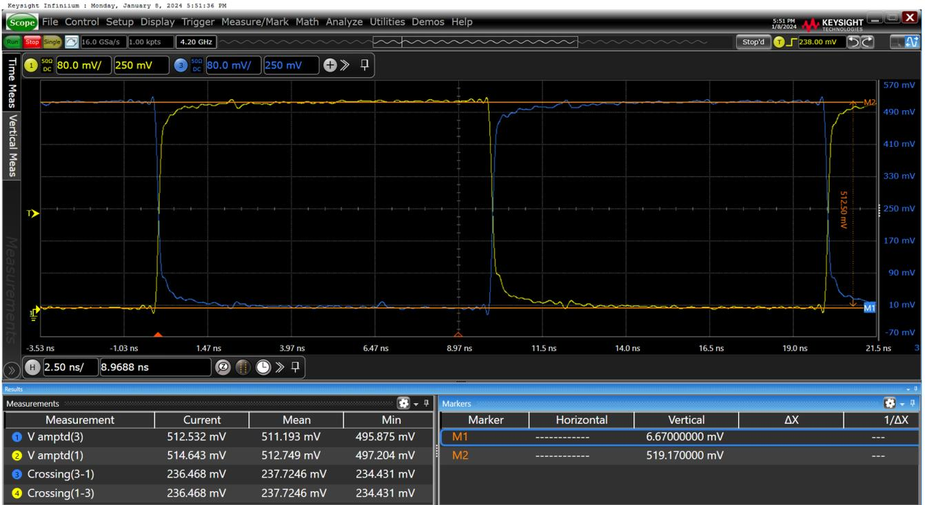
Figure 44. Vovs-HCSL Dual-Termination SWING = 950mV on nOUT11
