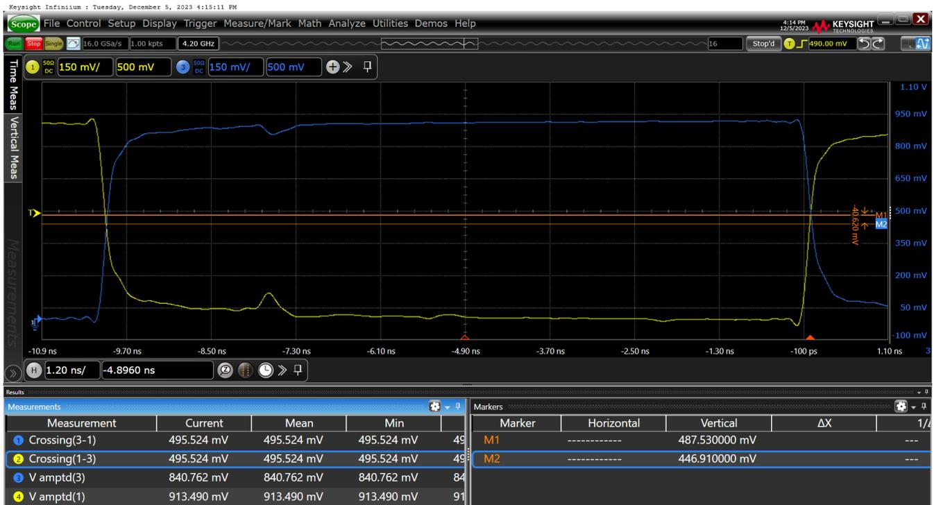
Figure 27. Vcross-HCSL External Termination SWING = 850mV on OUT11
