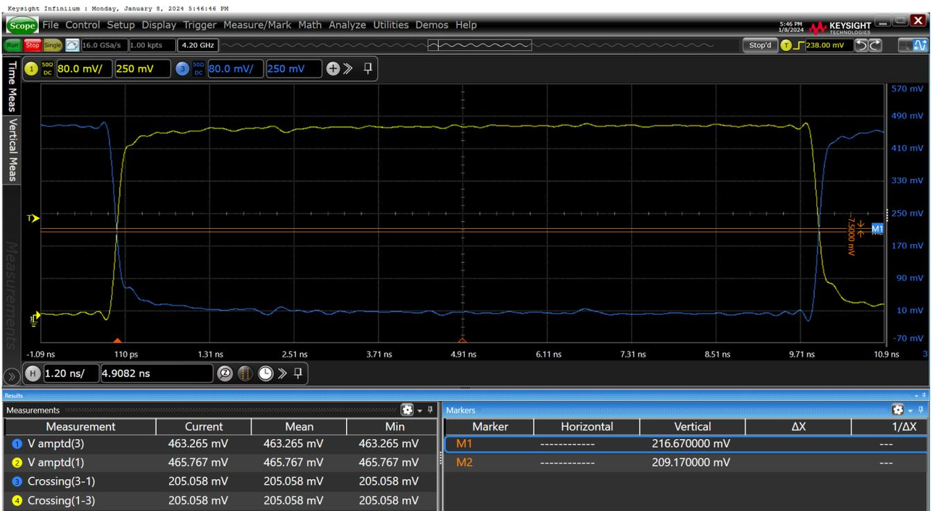
Figure 39. Vcross-HCSL Dual-Termination SWING = 850mV on nOUT11
