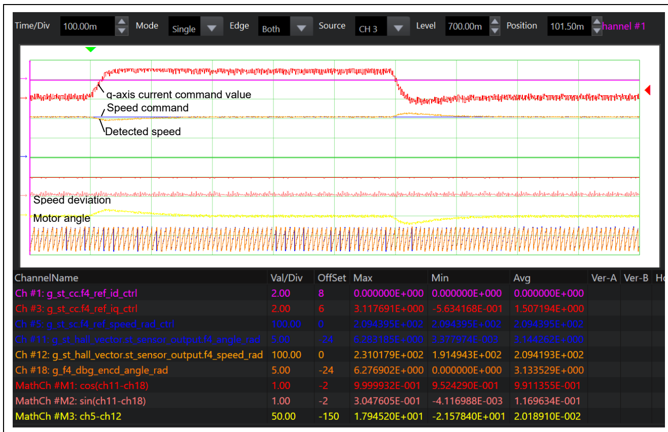
Figure 11-2 Load characteristics (at 2000r/min operation)
