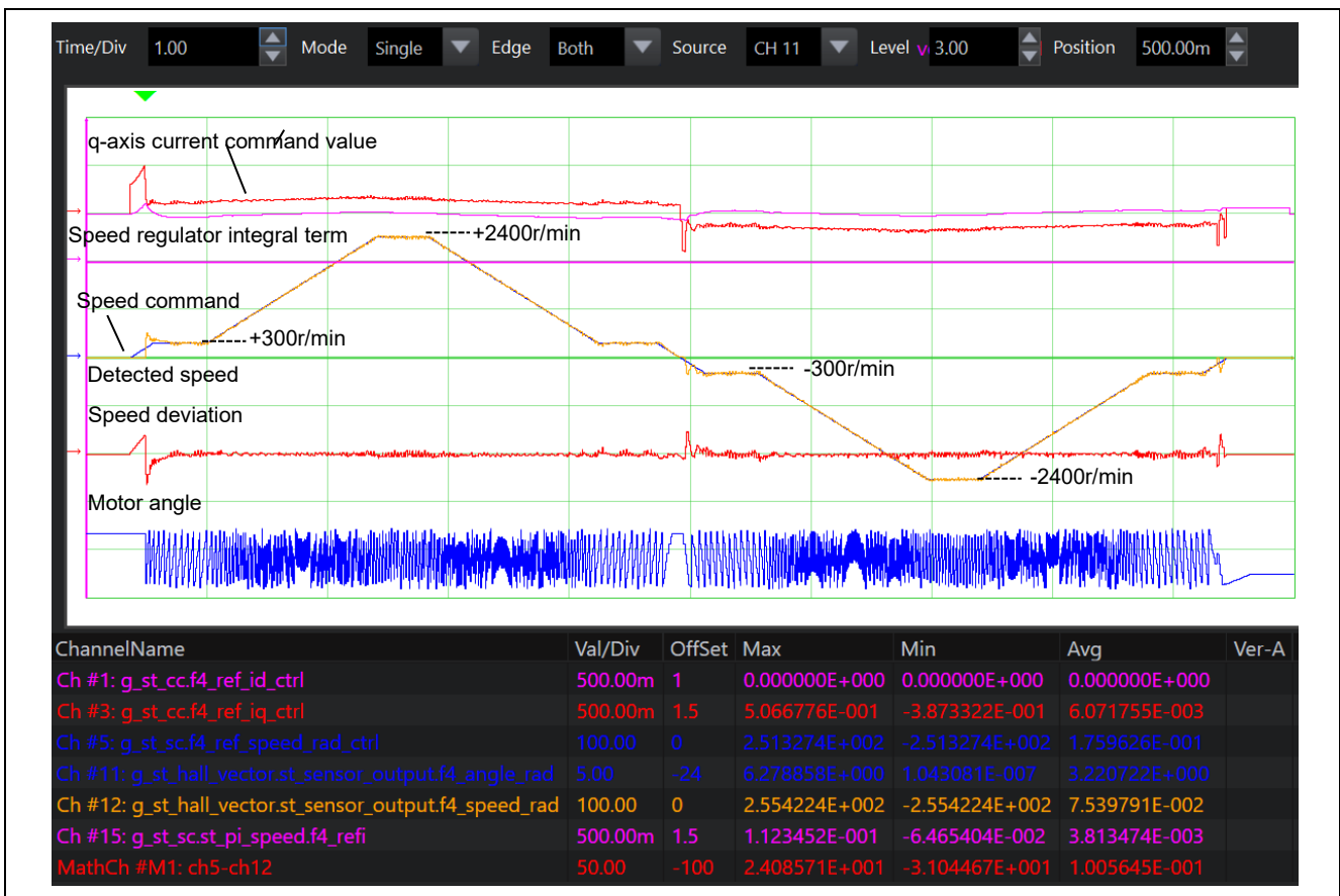
Figure 11-1 Acceleration/deceleration and forward/reverse characteristics
