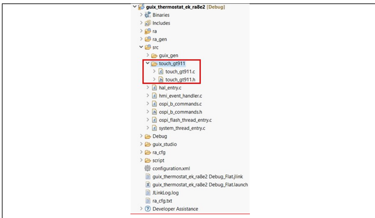
Figure 50. Copying files to the e 2 studio Project
