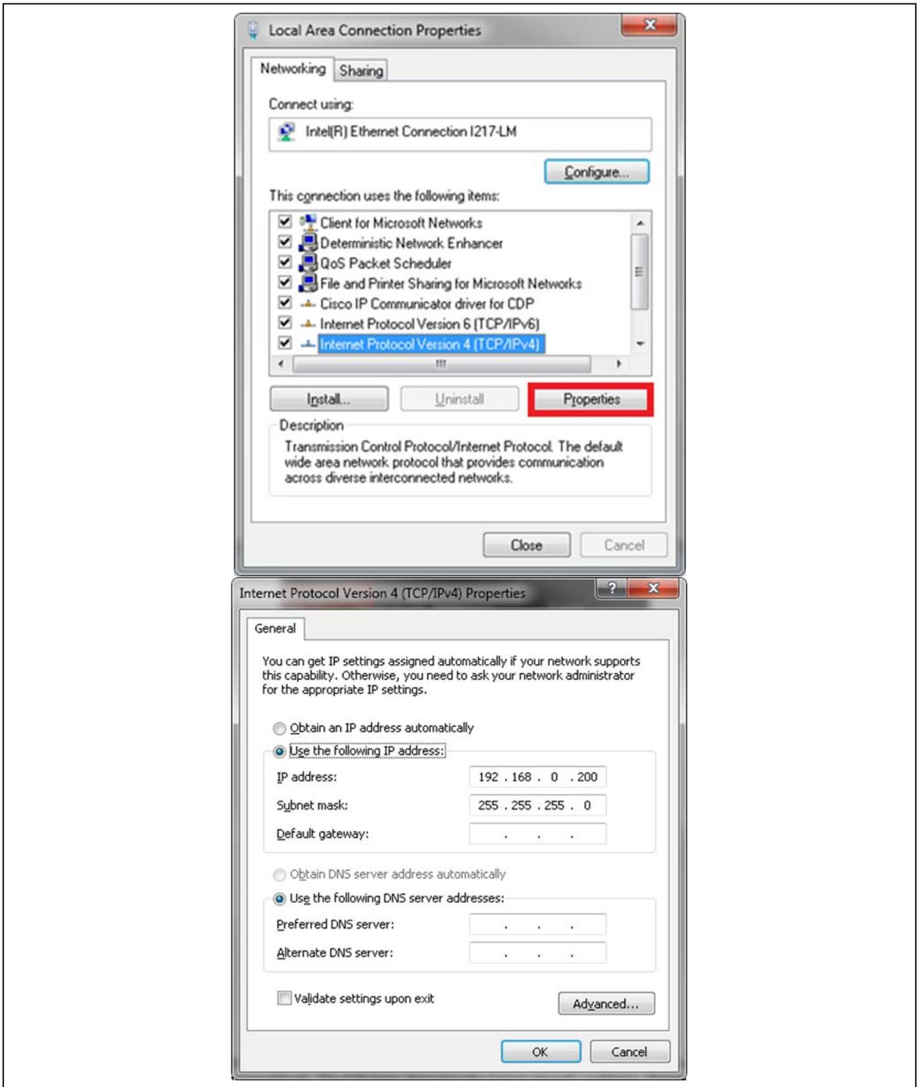
Figure 2. Static IP address for the Ethernet port of the PC
