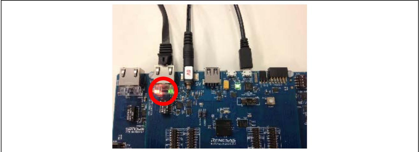
**Figure 8. Orange and green Ethernet status LEDs**
