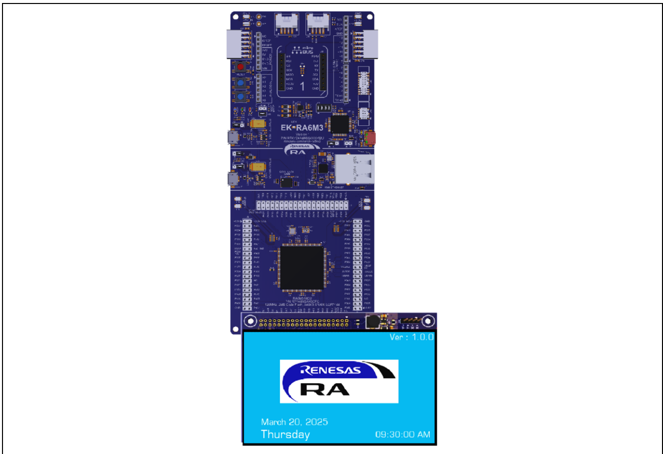
Figure 33. Connecting LCD Board to Graphics Expansion Connector of EK-RA6M3
