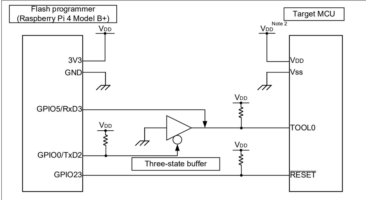
Note 1. This is a connection example when  $V_{DD}$  is 3.3V.
